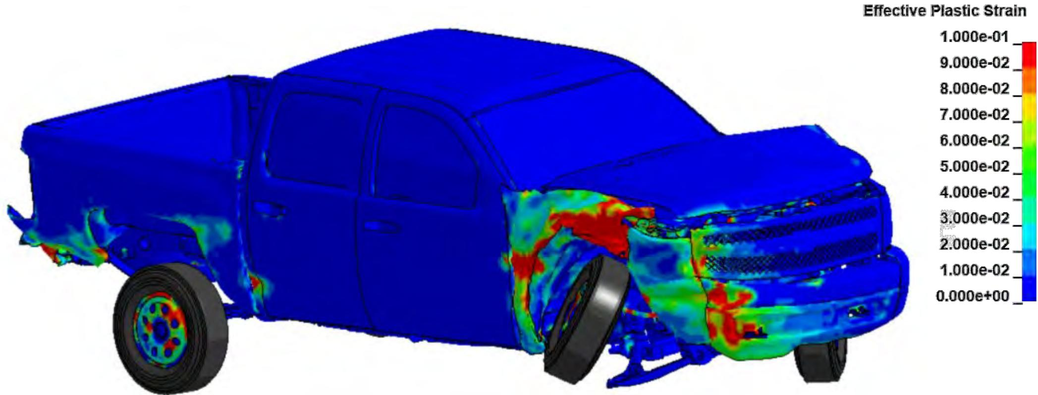
The most severe damages were to the front bumper, the front fender, the upper control arm of front suspension, fail ball joint on lower control arm, front and rear wheels, rear edge of rear door, front edge of truck bed, rear quarter panel of truck bed and rear bumper.
