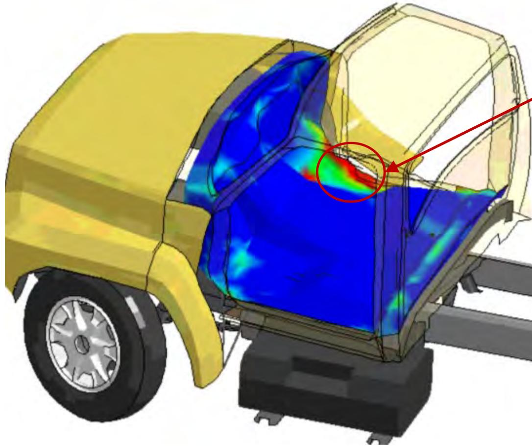
Maximum OCI was  $\approx$  5.5 inch (139 mm) and occurred at the lower right-front corner of the toe-pan at wheel well.
