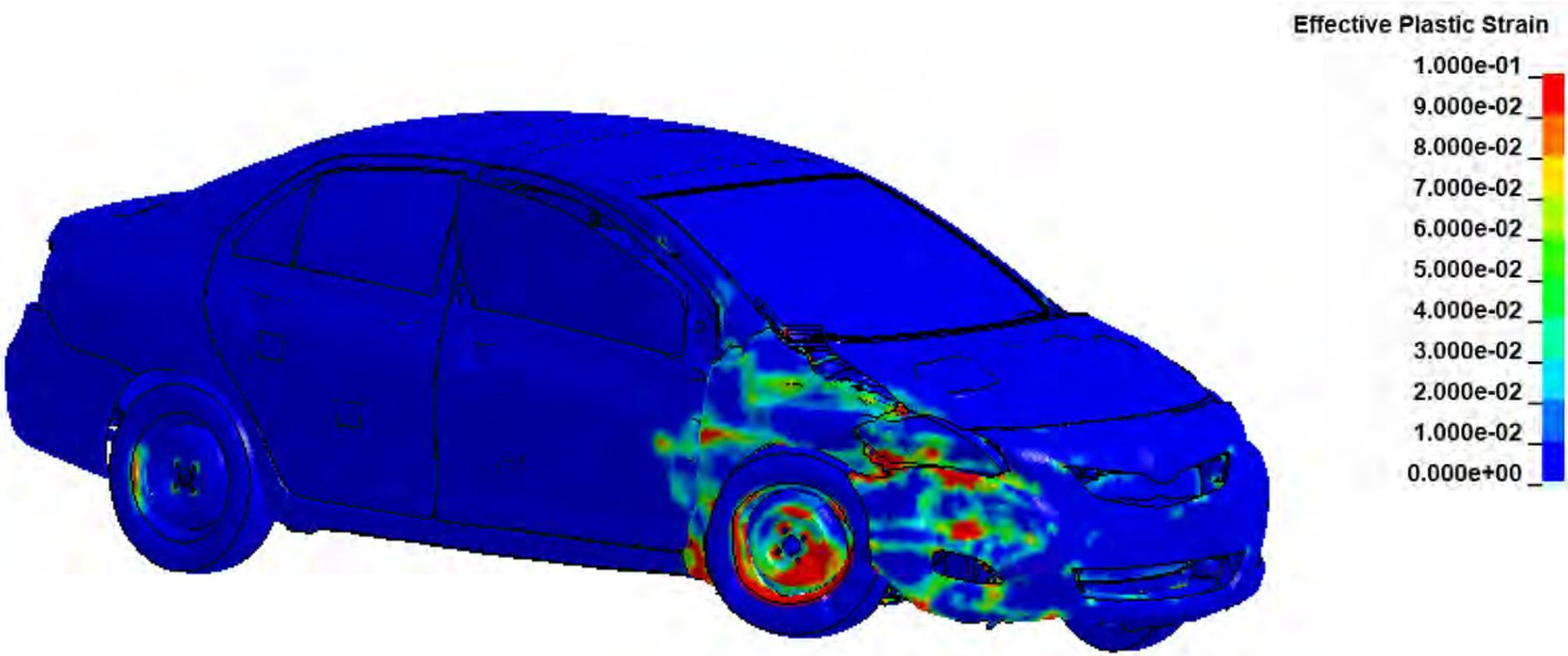
The most severe damages were to the front fender, the upper and lower control arm of front suspension, front wheel, and the leading edge of the front door on the impact side.
