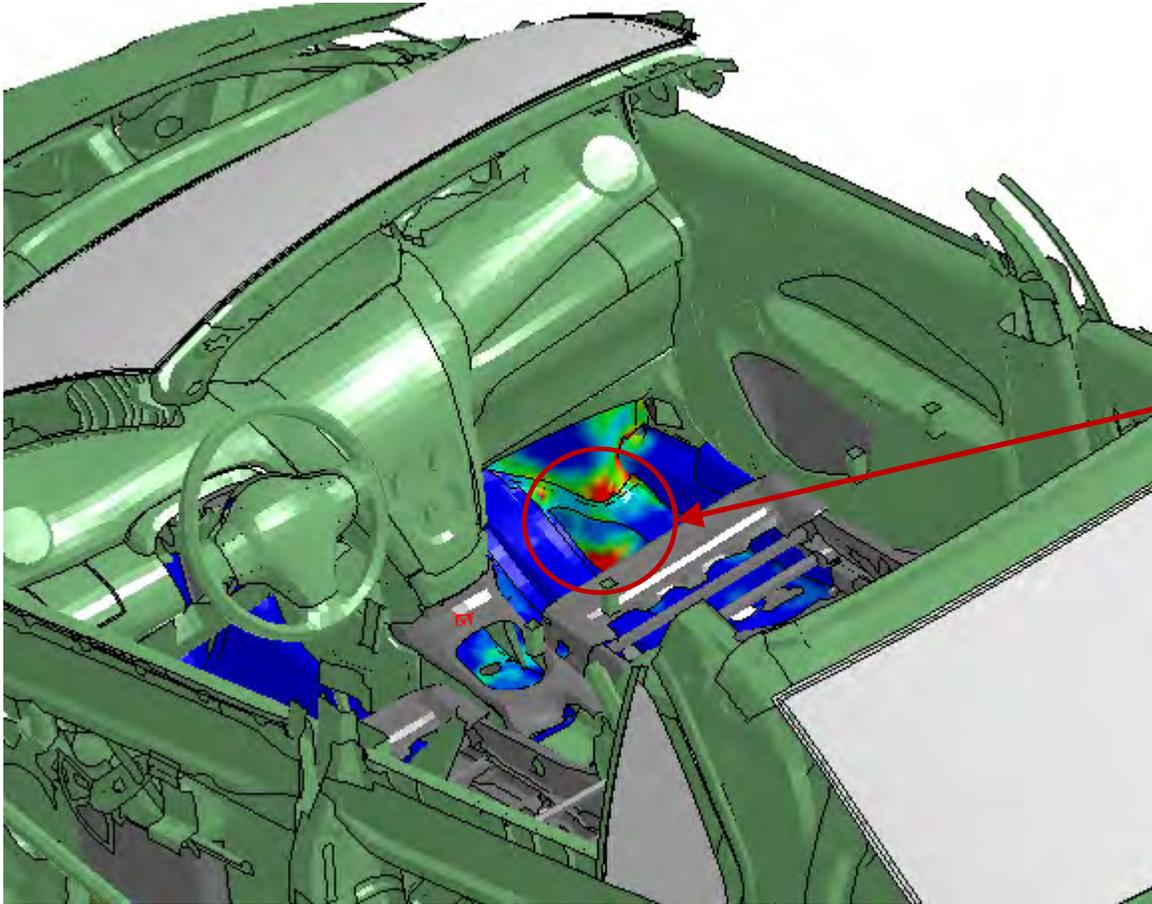
Maximum OCI of the floor, doors, and side panels was **≈3.4 inches** (87 mm) and occurred at the right-front toe-pan at the wheel well.
