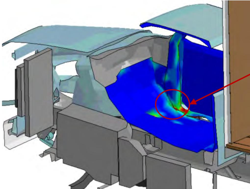
Maximum OCI was  $\approx$  1 inch (23 mm) and occurred at the lower right-front corner of the top-pan at the wheel well.
