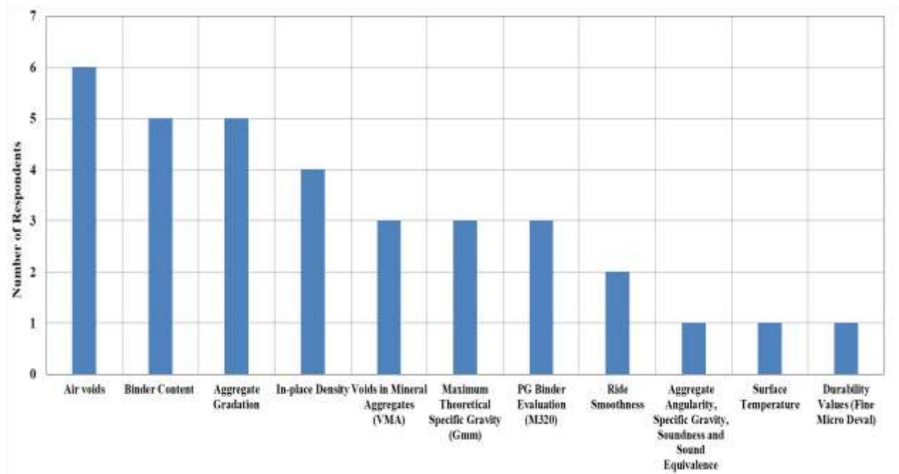
Figure 2-1. Suggested Optimal QA Tests
