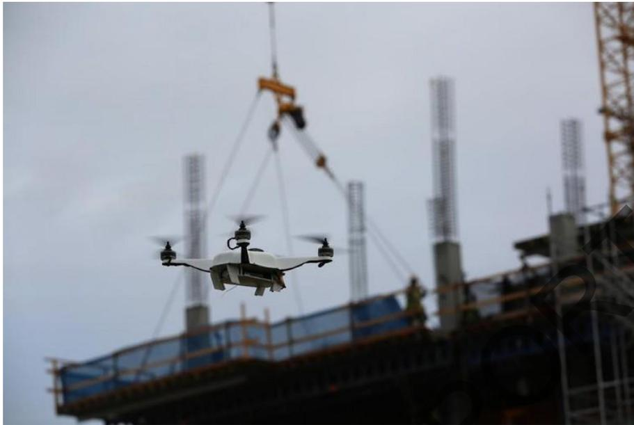
*Figure 4-17. Photo. UAV being used for time-lapse videos of construction progress.*
