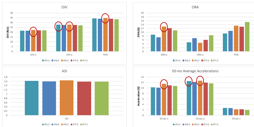
Figure 320. Comparison of occupant risk metrics computed in TRAP for Test 4-21.
