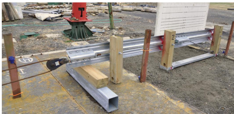
Figure 291. Test set-up for measuring force-deflection response of a standard two-post guardrail end-terminal anchor.
