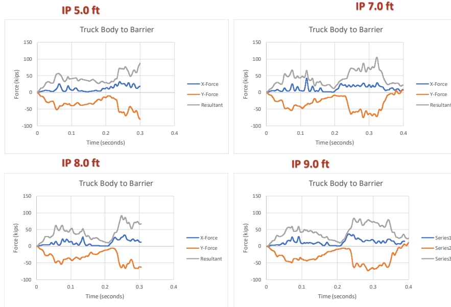
Figure 209. Longitudinal, lateral and resultant forces on barrier for each analysis case.
