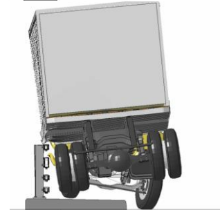
Figure 1. [Continued] Sequential views from FEA and Test NETC-3 from an upstream viewpoint.
