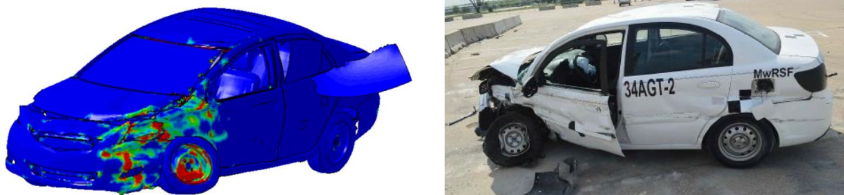
Figure 316. Comparison of vehicle damage for FEA (MaineDOT transition) and full-scale test (MwRSF transition).
