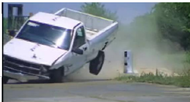
Figure 98. [Continued] Sequential views of FE analysis and Test 401181-1 from a downstream viewpoint.
