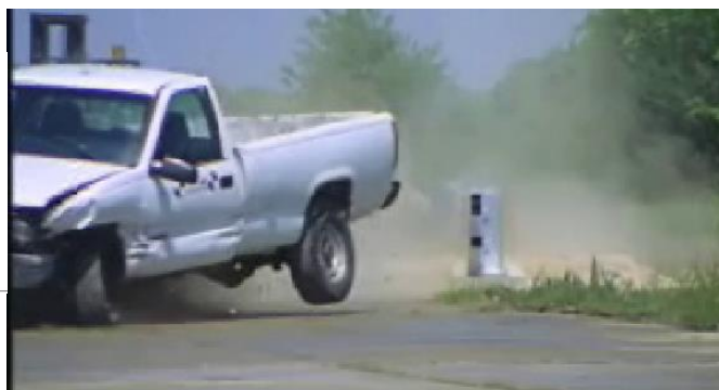
Figure 2. [CONTINUED] Sequential views from FEA and Test 401181-1 from a downstream viewpoint.
