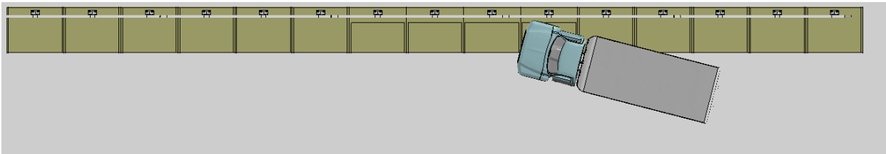
Figure S-1. Sequential views from analysis of MASH Test 4-12 for NETC 4-Bar bridge rail from an overhead viewpoint.
