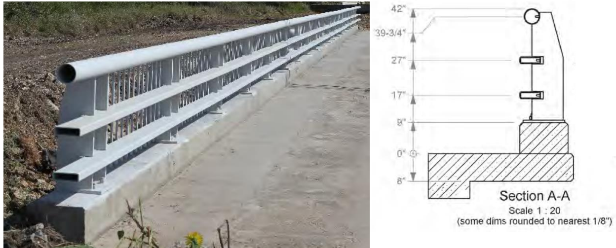
Figure 168. Photo and cross-section drawing of the MASH TL4 TxDOT C2P bridge rail.
