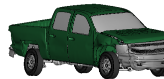
Figure Z-3. [Continued] Sequential views from analysis of MASH Test 3-21 for AGT 2-Bar bridge rail from an oblique viewpoint.
