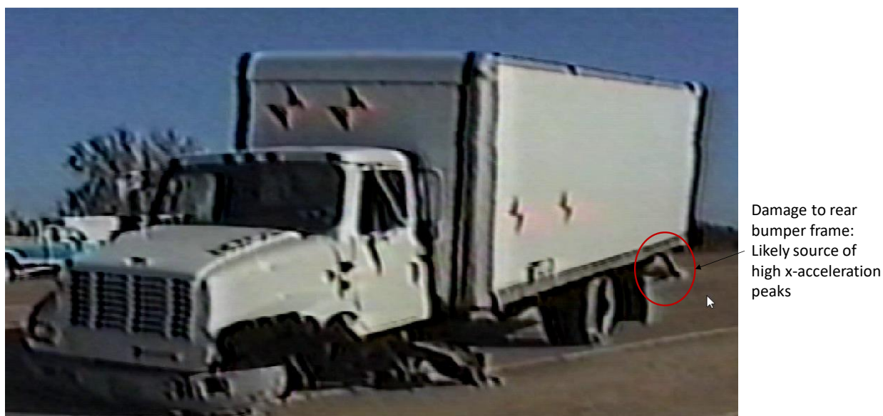
Figure 79. Post-test photo of vehicle damages.
