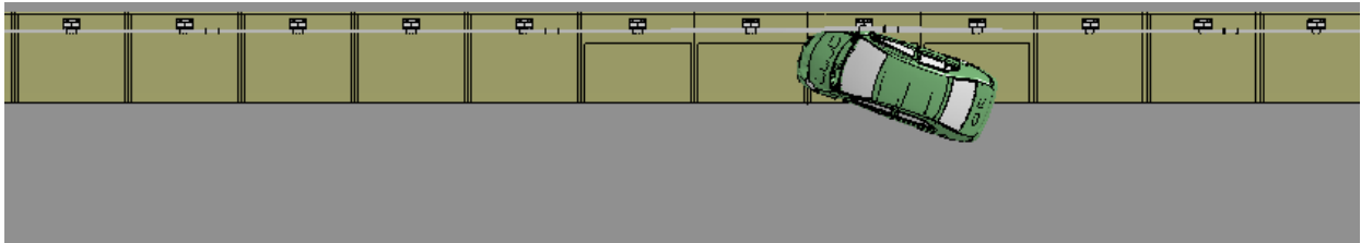
Figure Q-1. Sequential views from analysis of MASH Test 4-10 for NETC 4-Bar bridge rail from an overhead viewpoint.
