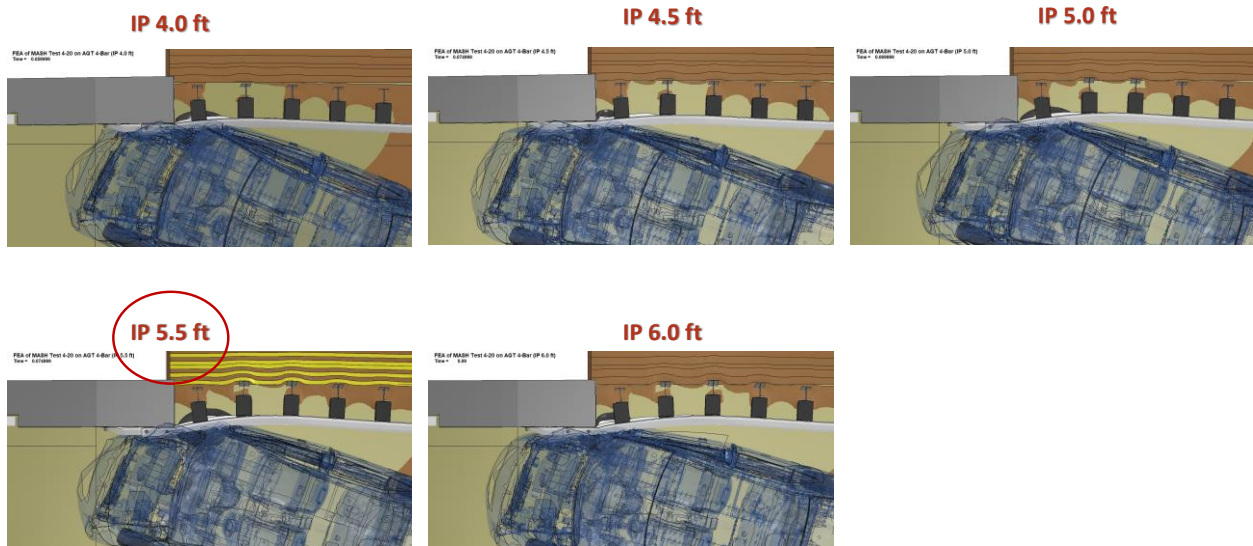
Figure 293. Results of the Test 4-20 simulations showing the deformation and position of the vehicle just before the tire impacted against the buttress for each case.
