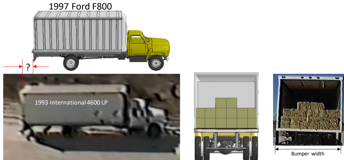
Figure 63. FEA vehicle and test vehicle illustrating the differences in cargo-box length and bumper design.
