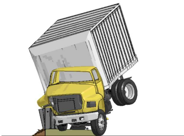
Figure 359. Working width for Test 4-22 on MaineDOT transition.
