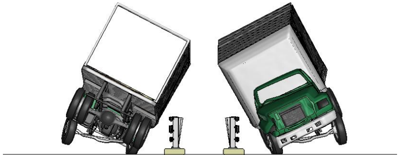
Figure M-2. [Continued] Sequential views from analysis of MASH Test 4-12 for NETC 3-Bar bridge rail from upstream and downstream viewpoints – Case 2.
