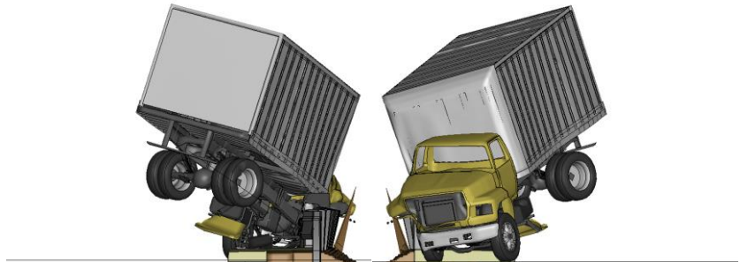
Figure V-2. [Continued] Sequential views from analysis of MASH Test 4-22 for AGT 4-Bar bridge rail from upstream and downstream viewpoints.
