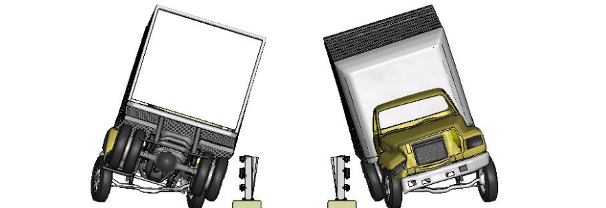
Figure K-2. [Continued] Sequential views from analysis of MASH Test 4-12 for NETC 3-Bar bridge rail from upstream and downstream viewpoints – Case 1.
