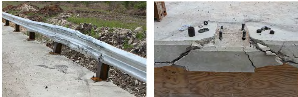
Figure 12. Punching shear damage mode experienced in NCHRP Report 350 Test 3-11 on the TxDOT T101 bridge rail.
