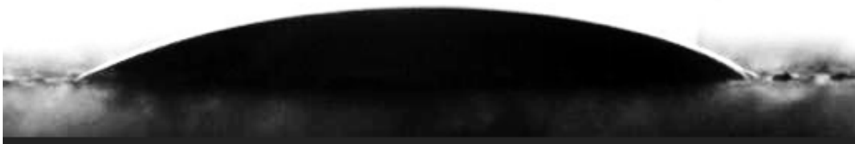
Image of a droplet of liquid paint C on G2b surface, Trial 4, at t = 6 sec, contact angle = 30^\circ
