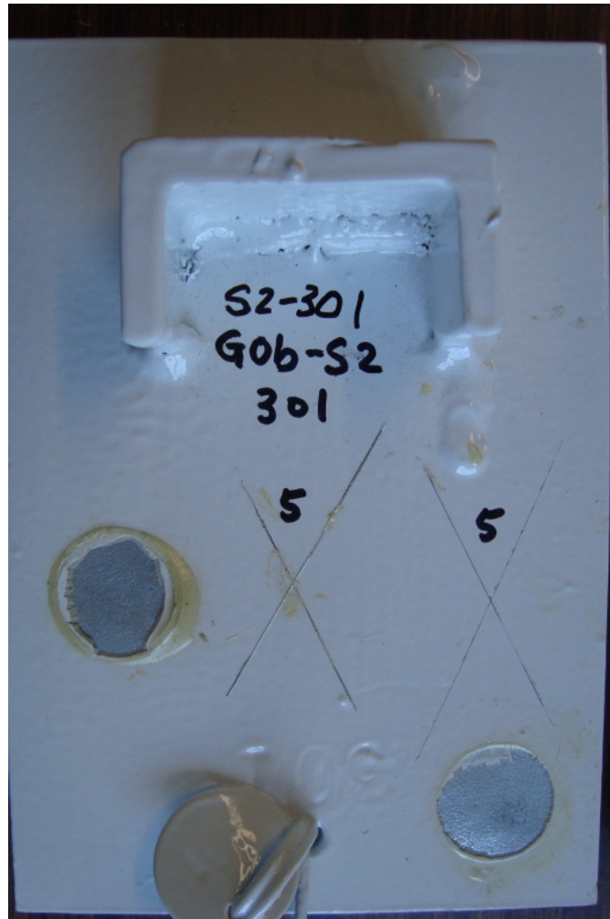
Fig 18. A photograph showing the X-cut scores of 5 for Test panel #301 with G0b-S2 coating.
