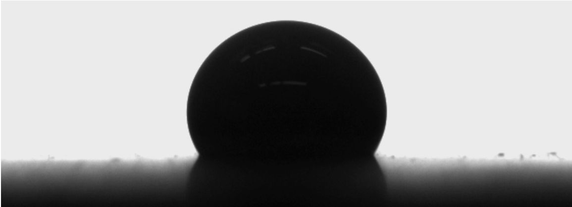
Image of a droplet of liquid paint S1 on the G0m surface, trial 1 t = 6 sec. Contact angle \theta = 123^\circ .
