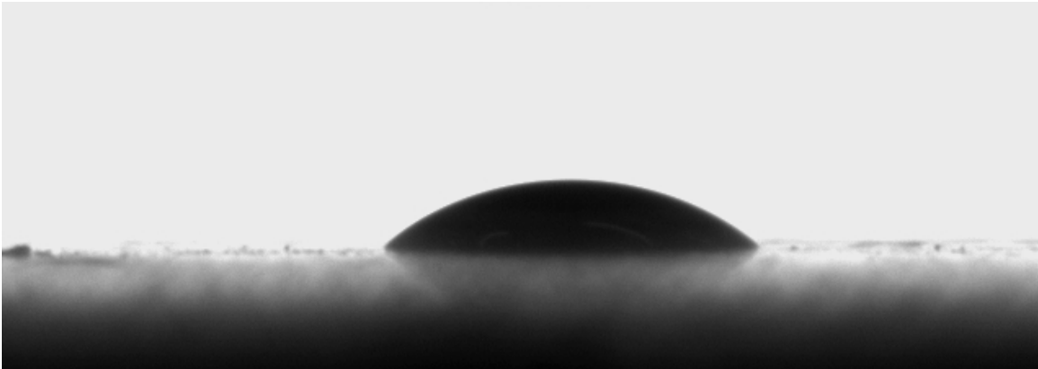
Paint I droplet on G0m surface trial 2 at t = 3 second, contact angle = 42^\circ
