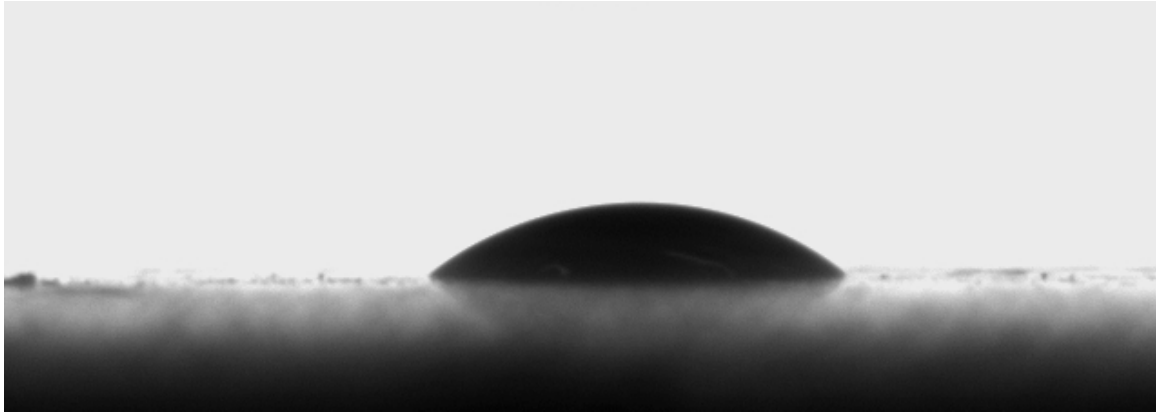
Paint I droplet on G0m surface trial 2 at t = 30 sec, contact angle = 40^\circ Contact angle at t = 5 sec is 41^\circ ,
