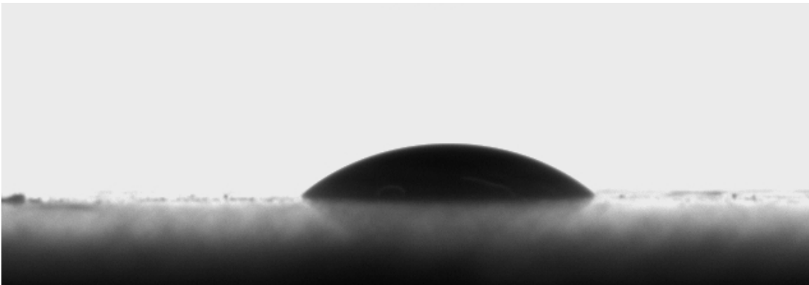
Paint I droplet on G0m surface trial 2 at t = 6 sec, contact angle = 40^\circ
