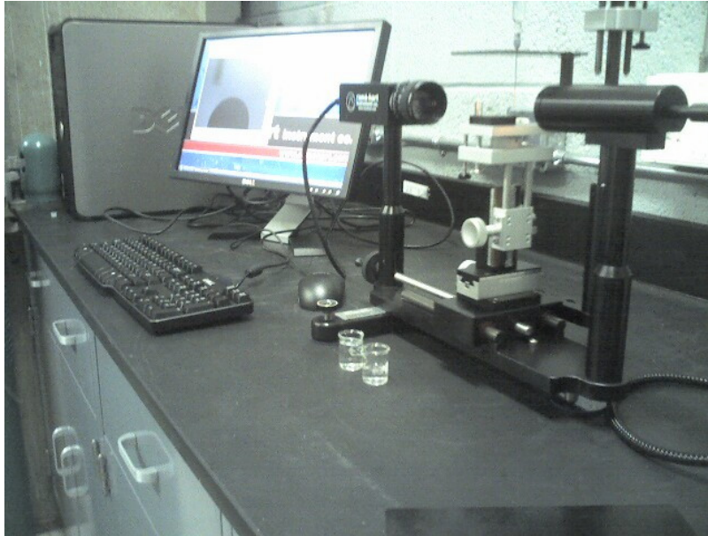
Figure 5. A goniometer for measuring the liquid paint wetting of a profiled zinc surface.
