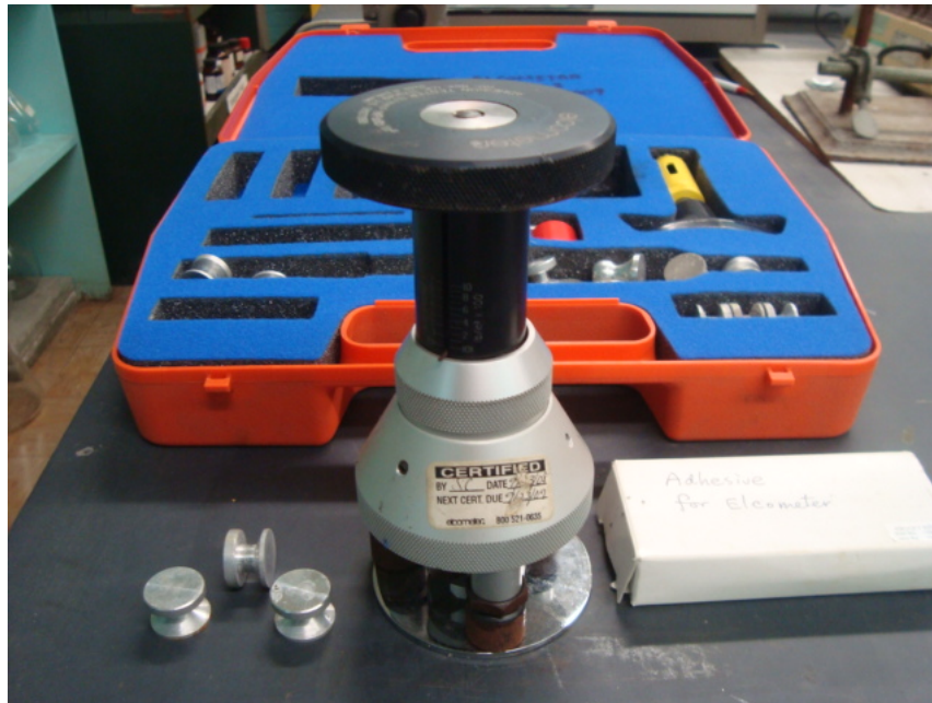
Fig. 13. Pull-off Strength tester, Elcometer Model 106, manufactured by Elcometer, Michigan.
