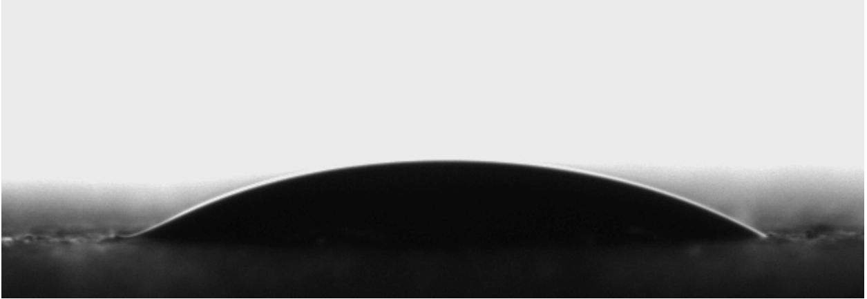
Image of a droplet of liquid paint S2 on G2b surface, trial 5, contact angle \theta = 26^\circ at t = 5 sec
