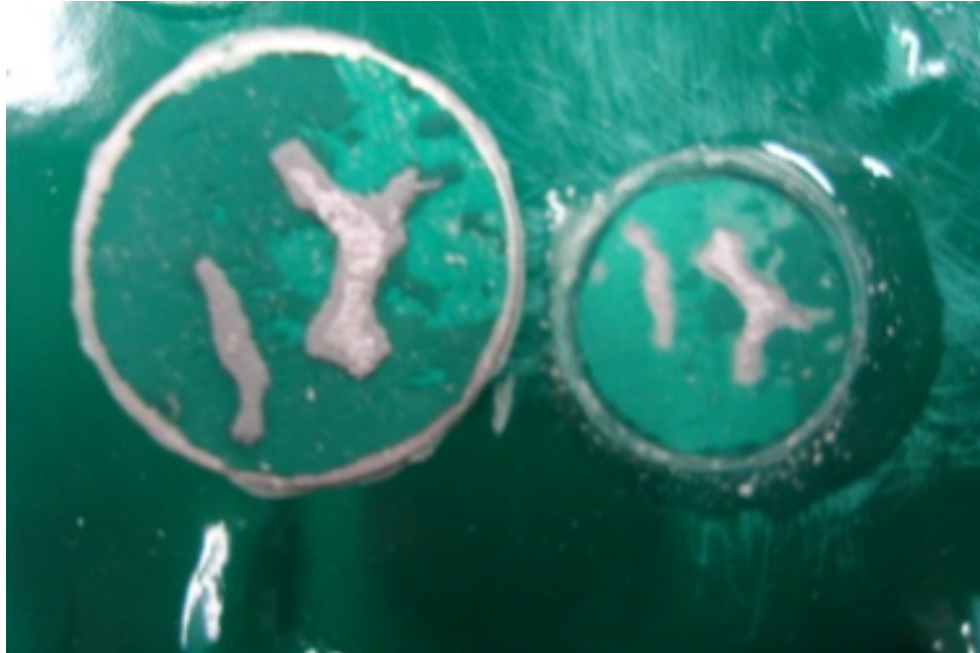
Figure 15. Photograph of the break surfaces on the Dolly (left) and the Test Spot for G2b-I, Test 1.
