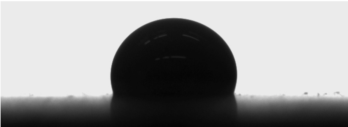
Image of a droplet of liquid paint S1 on the G0m surface, trial 1 t = 6 sec. Contact angle \theta = 109^\circ .
