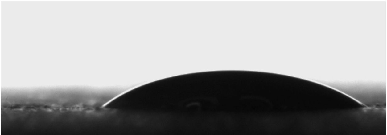
Image of a droplet of liquid paint S2 on G2b surface, trial 3, contact angle \theta = 38^\circ at t = 5 sec.
