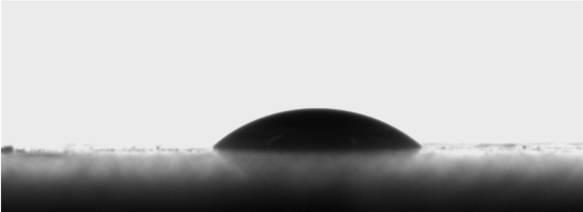
Paint I droplet on G0m surface trial 2 at t = 0 second, contact angle = 43^\circ
