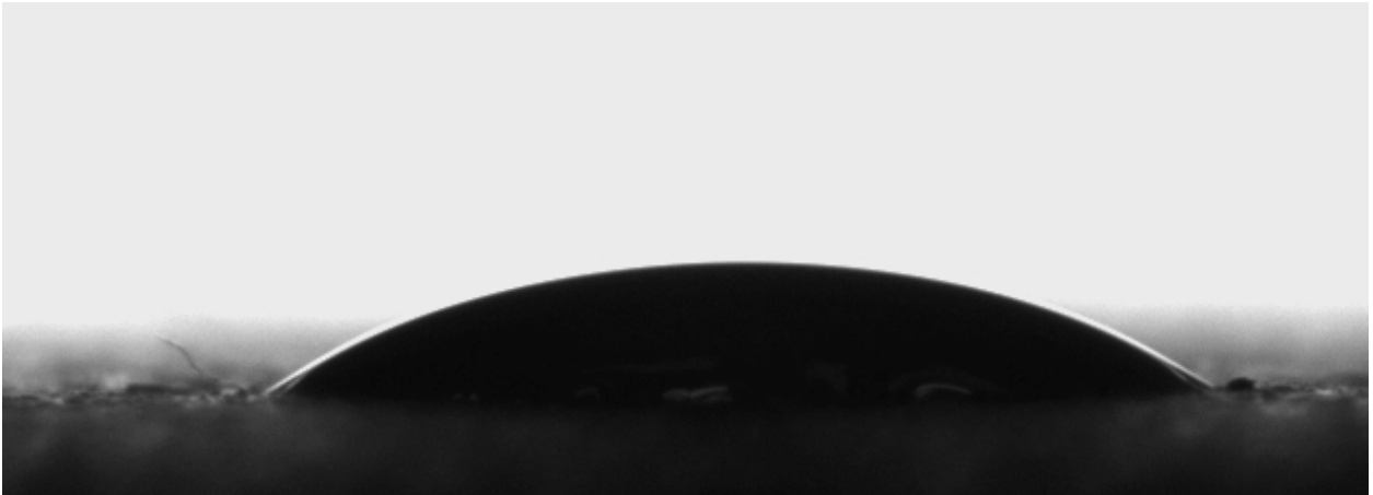
Image of a droplet of liquid paint S2 on G2b surface, trial 7, contact angle \theta = 35^\circ at t = 5 sec.
