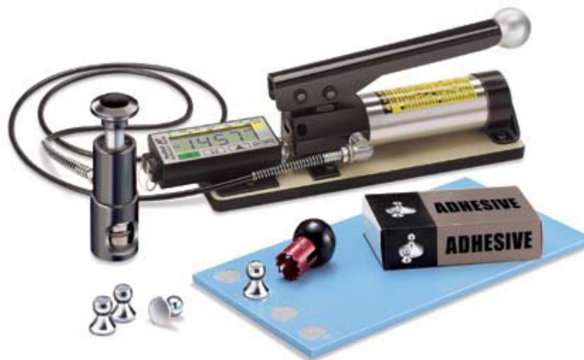
Figure 14 Pull-off strength tester. PosiTest AT-M manufactured by DeFelsko, New York.
