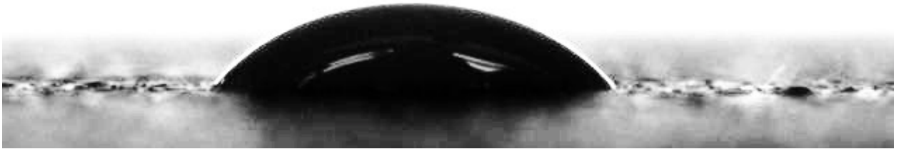
Image of a droplet of liquid paint S1 on G2b surface, trial 1 t = 6 sec, contact angle \theta = 45^\circ
