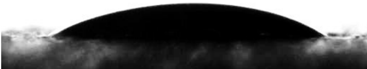
Image of a droplet of liquid paint C on G2b surface, Trial 5, at t = 6 sec, contact angle = 35^\circ
