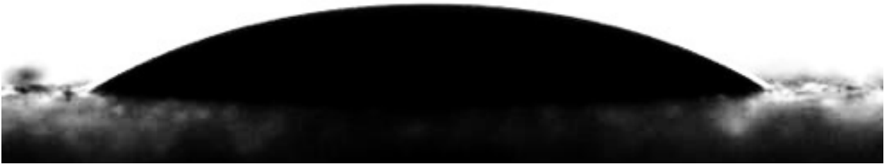
G2b-S2, Trial 1. A droplet of paint S2 on Galvanized, stored for 2 weeks before blast profiling and painting. At t=5 sec, \theta = 36^\circ
