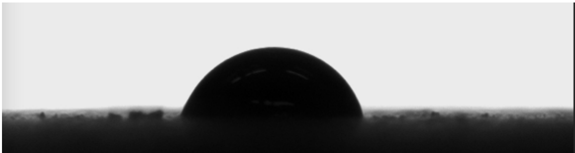
M0-I Trial 2, t = 5 sec., contact angle = 75^\circ .
