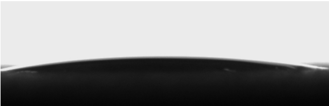
M0-S3 Trial 2, a droplet of sealant S3 on the surface of M0 at t = 1 sec, contact angle 5^\circ .
