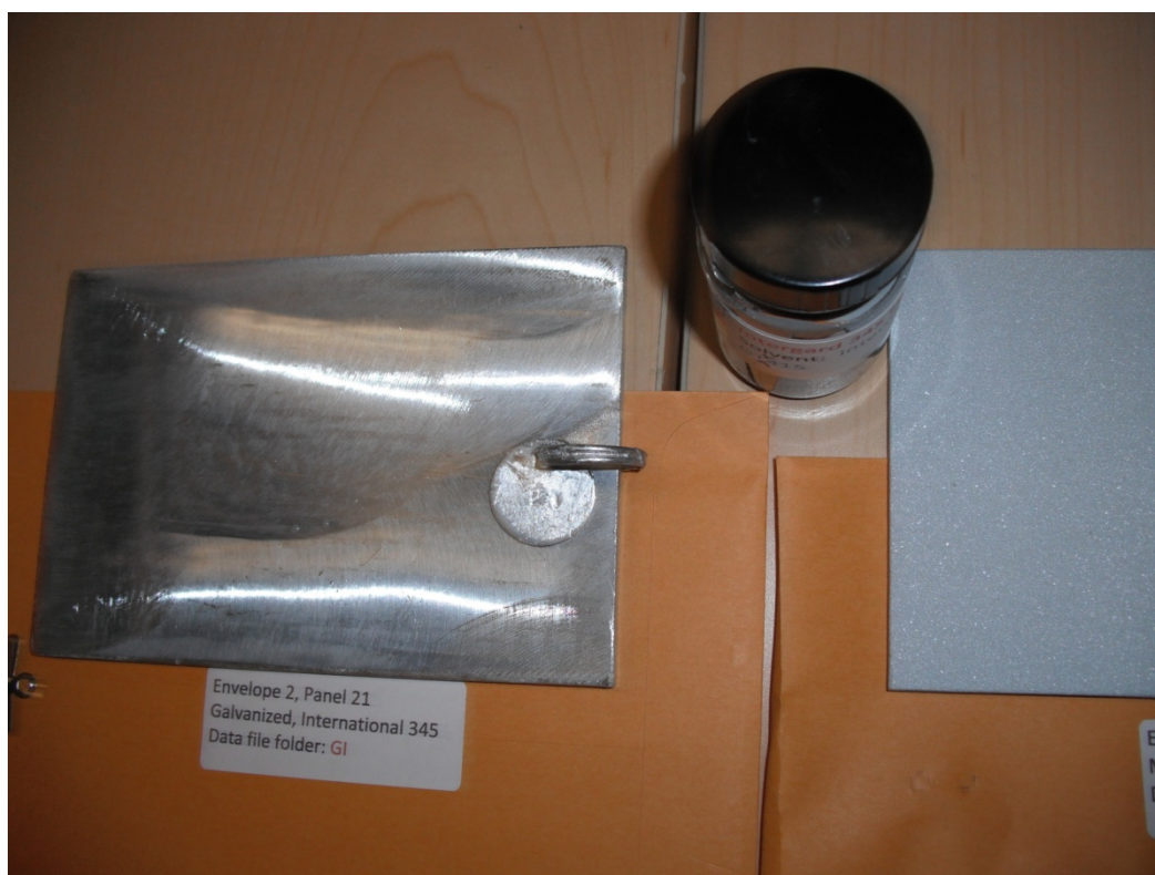
Figure 4. Rough zinc surfaces produced by different methods. Left: Galvanized steel surface profiled by mechanical grinding. Right: Zinc metallized steel produced by thermal spray.
