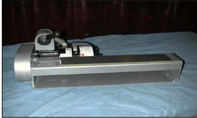
Figure 4. Flexural Tension Tester
