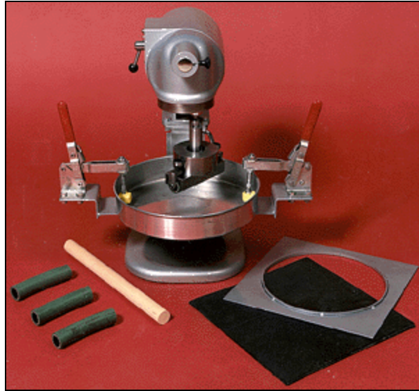
Figure 3. Abrasion Tester (Picture courtesy www.benedictslurry.com )
