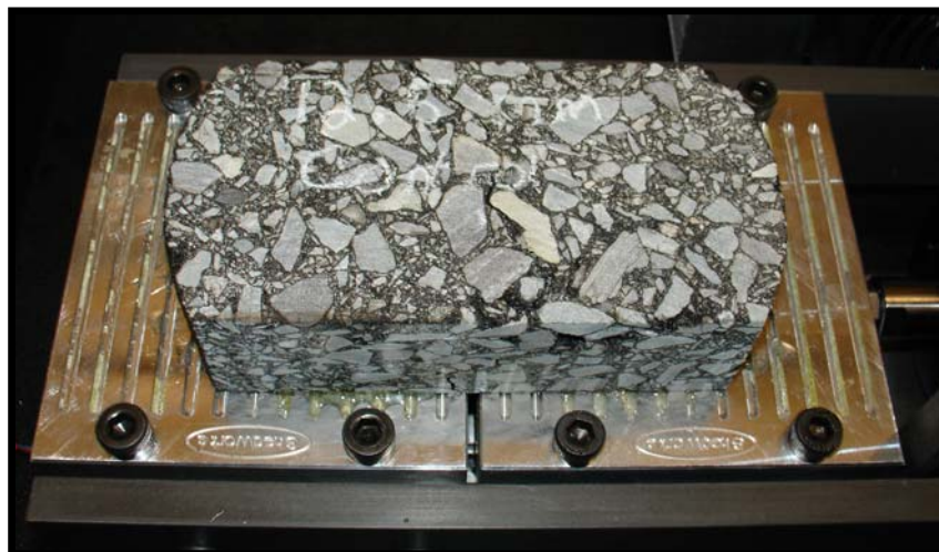
Figure 7. Overlay Tester - Test Specimen Assembly
