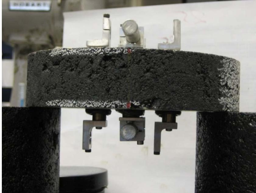
**Figure 2.8 Brackets and Brass Targets Curing**
