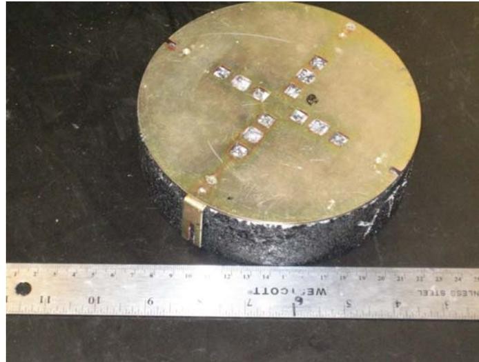
**Figure 2.5 Brass Gluing Jig**
