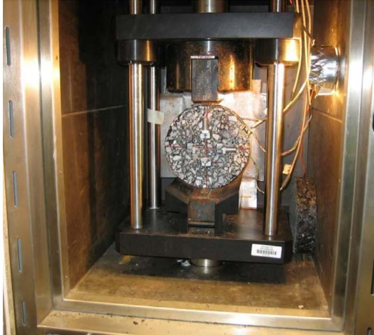
**Figure 2.10 Instrumented Specimen Ready for Testing**
