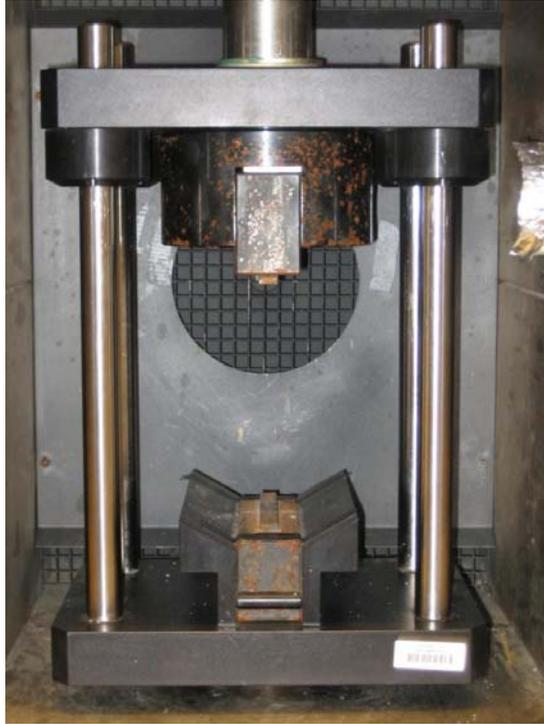
**Figure 2.3 ITC IDT Load Fixture in Environmental Chamber**
