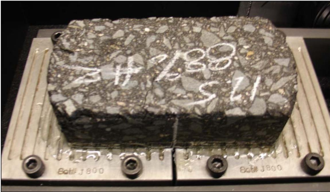
Figure 7. Overlay test specimen setup
