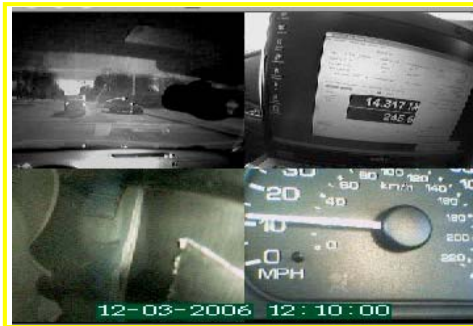
Figure 13: Approaching one of two stop signs (upper left). Note the lead vehicle is within 14.3 m (upper right), the vehicle is traveling approximately 12 mph (lower right), the driver is looking generally straight ahead and the foot is on the brake (lower left).
