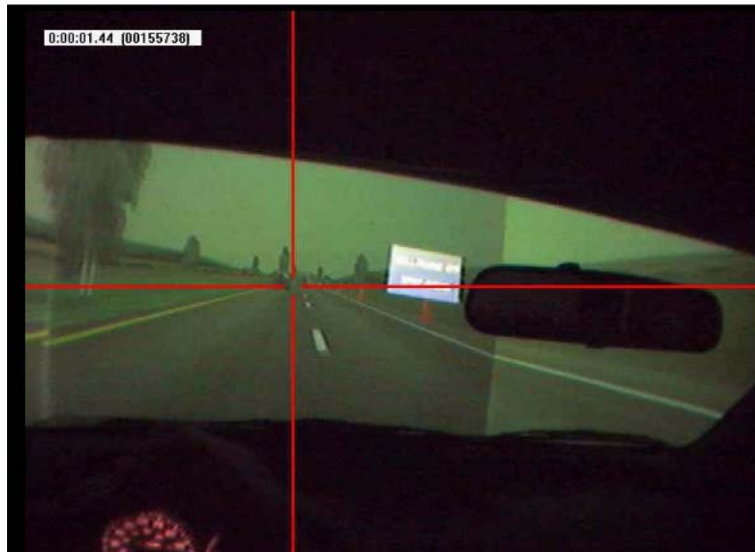
Figure 17 Illuminated flashing warning displayed at the roadside, “SLOW AHEAD TURN PHONE OFF.”
