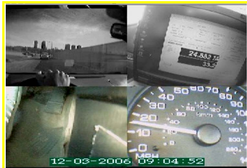
Figure 12: View approaching a road bump (upper left). The lead vehicle is seen braking in response to the road bump ahead. The driver's foot is on the brake pedal (lower left).
