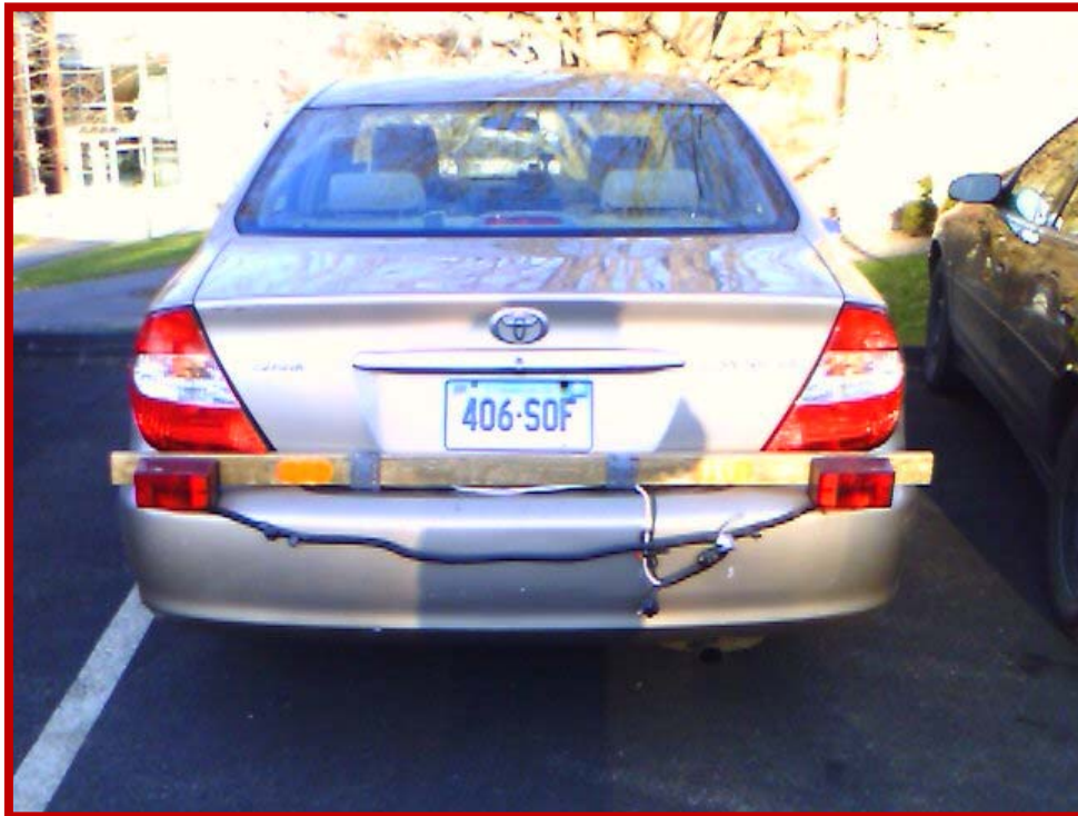
Figure 7: The modified brake light system that was utilized in Study II.
