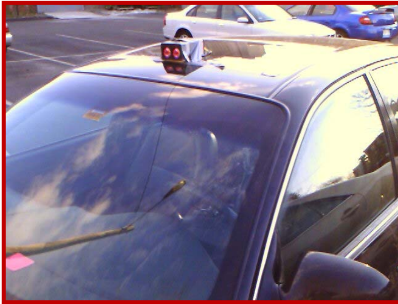
Figure 8: United Laboratories Systems range finder placed on the driving school vehicle.
