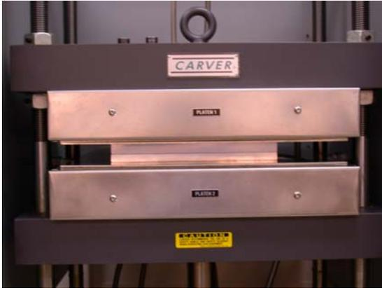
(e). Mold Curing in the Heat Press
