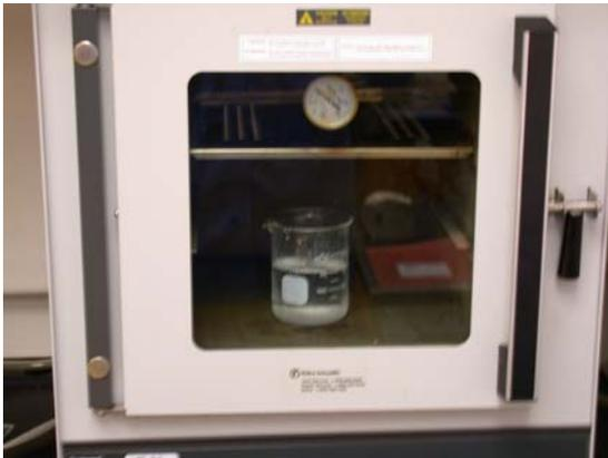
(c). Vacuum the Resin in the Vacuum Oven
