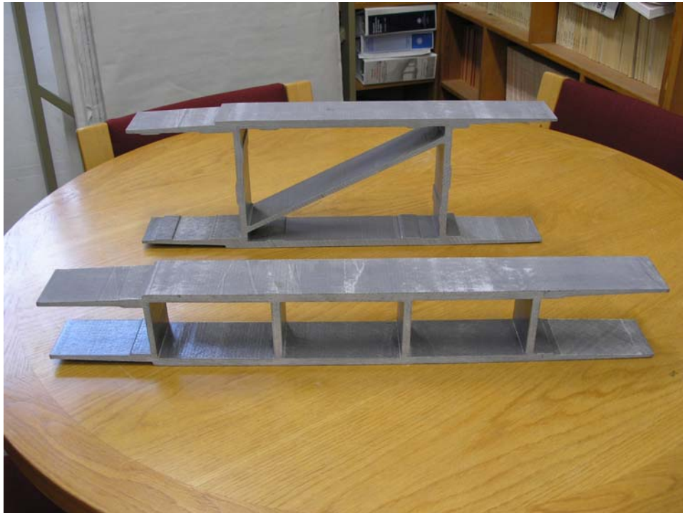
Figure 2.12 – Different bridge deck sections (4 in. and 8 in. deep) manufactured by Bedford Plastics
