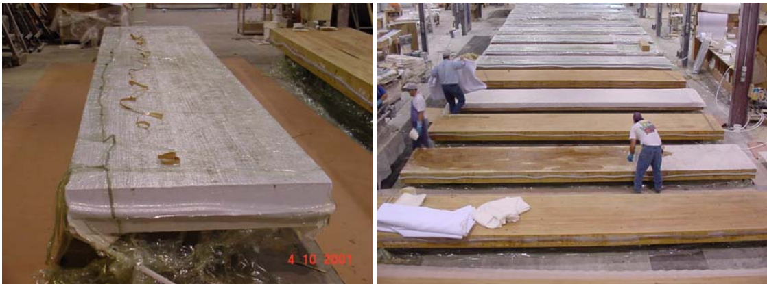
Figure 4.6 – Fabrication of FRP-glulam deck panels for the Skidmore Bridge (Photograph courtesy of Dale Peabody, Maine DOT)
