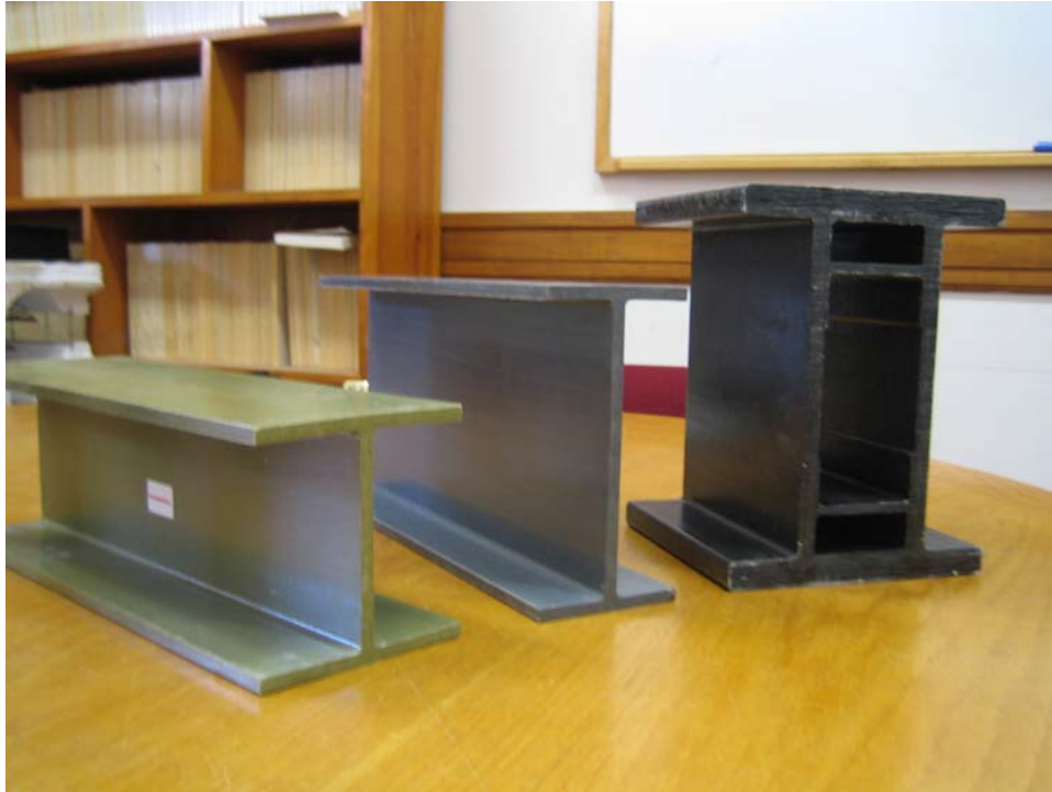
Figure 2.13 – Structural shapes produced by Strongwell for use in bridge decks
