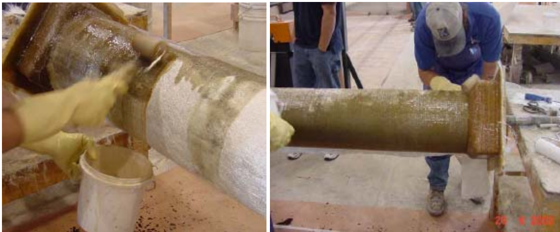
Figure 4.15 – Fabrication of glass fiber-reinforced drain using wet-layup procedure (Photograph courtesy of Dale Peabody, Maine DOT)
