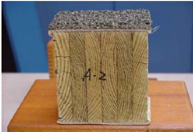
Figure 4.9 – Vertically laminated glulam panels used in the Milbridge Municipal Pier (Photograph courtesy of Dale Peabody, Maine DOT)
