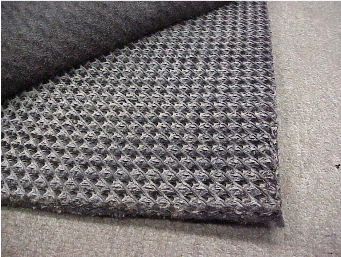
Figure 3.3 Photo of internal structure of drainage geocomposite and external filter fabric.
