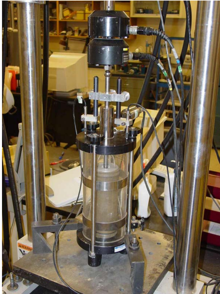
Figure 86. Resilient Modulus test in Progress
