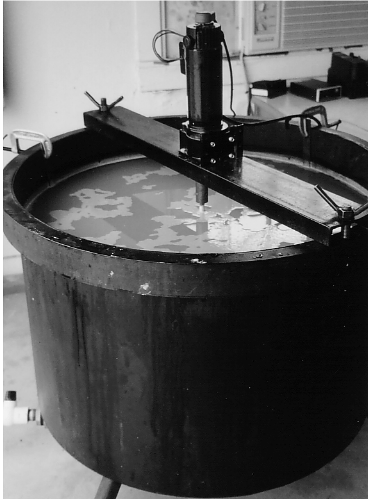
Figure 7.6 Shear Stress Test Tank
