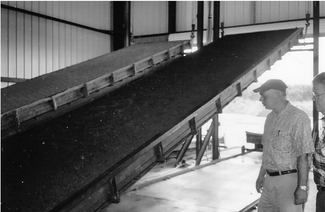
Figure 7.1 Sheet Erosion Test Beds at TTI College Station, Texas
