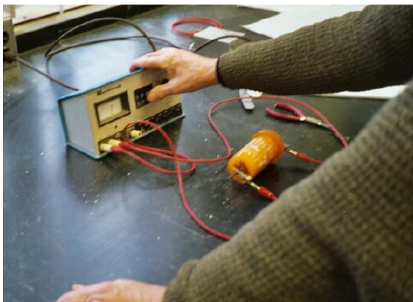
Figure D-2 Conductivity Bridge used to Determine Moisture in Salt
