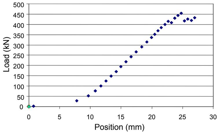
Figure 5.7 Load vs. Crosshead Position for Specimen T2
