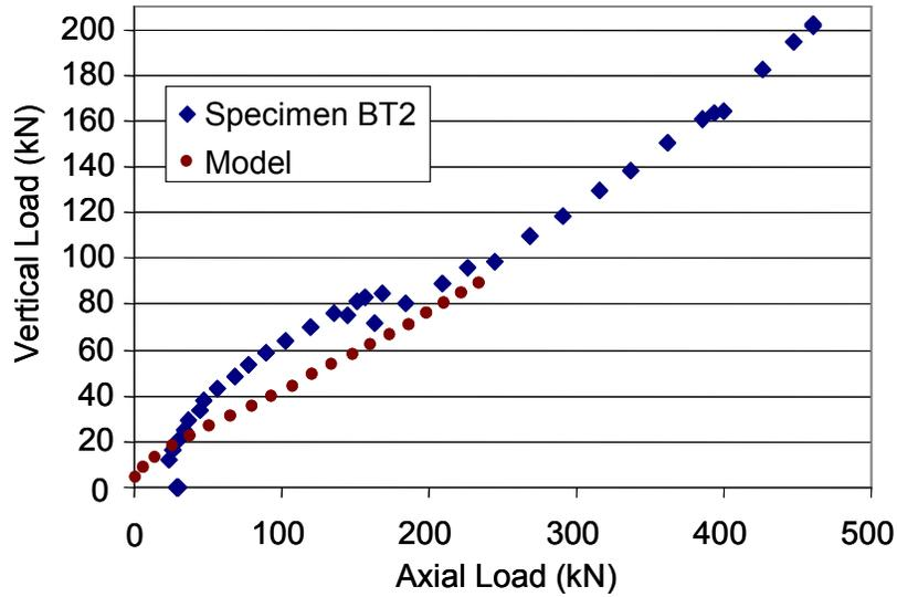
Figure 6.9 Specimen BT2 Transverse Load vs. Axial Tension
