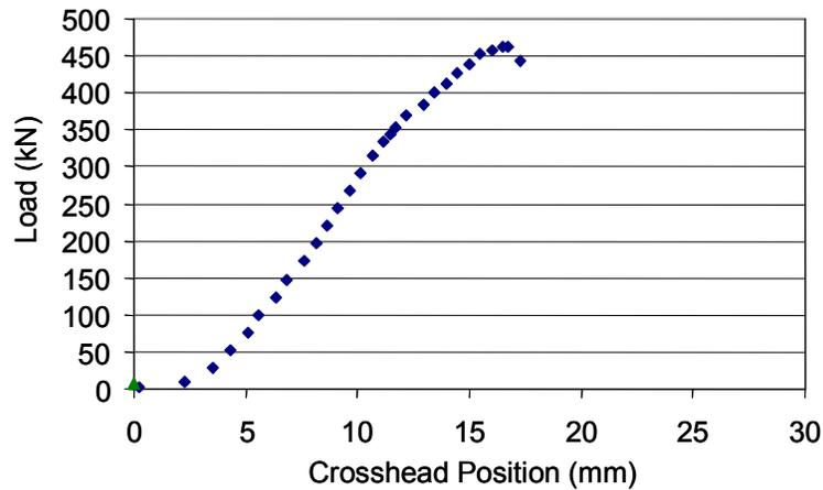
Figure 5.4 Load vs. Crosshead Position for Specimen T1
