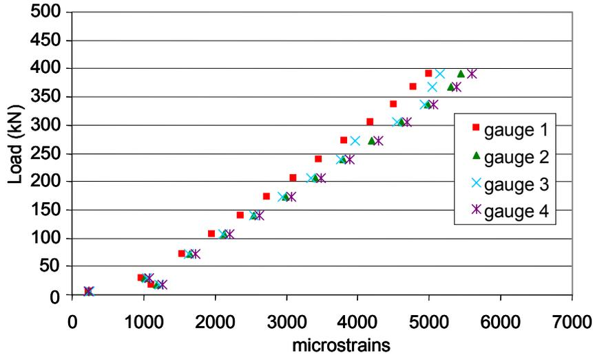
Figure 5.12 Load-Strain Relation for Specimen T5
