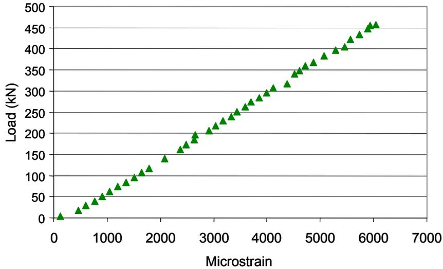
Figure 5.3 Load-Strain Relation for Specimen T1
