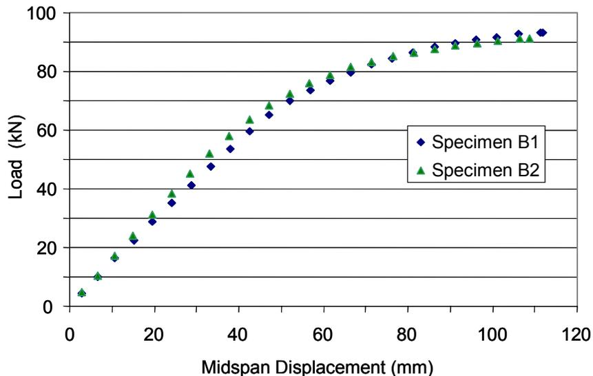
Figure 4.3: Flexural Load-Displacement Response
