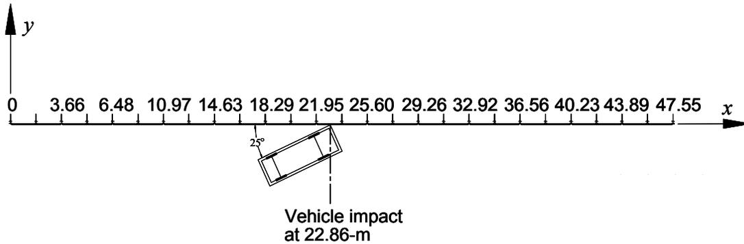
Figure 2.1 Guardrail System Layout (all dimensions in meters)
