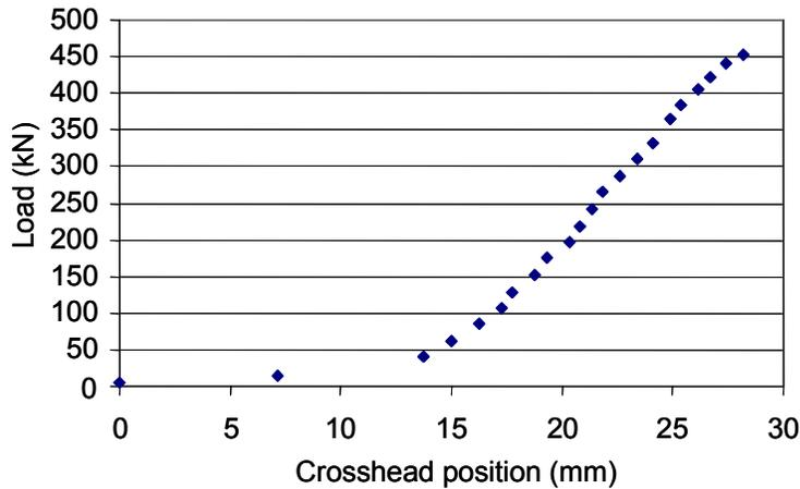
Figure 5.9 Load vs. Crosshead Position for Specimen T3
