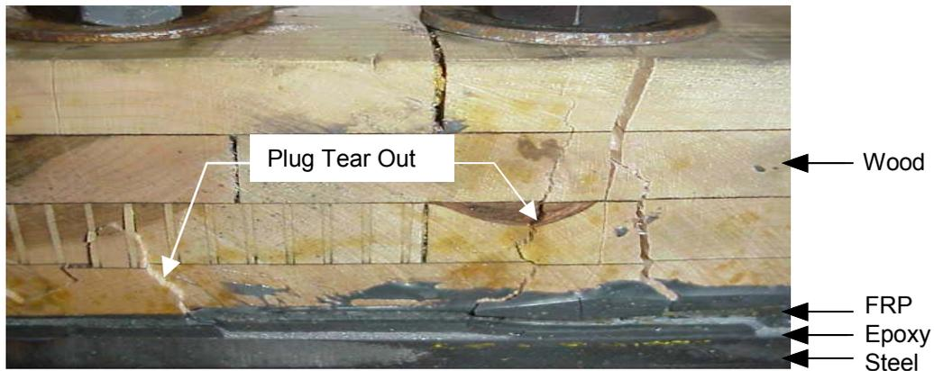
Figure 5.5 Bolt Plug Tear-Out for Specimen T1
