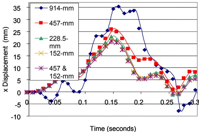
Figure 2.2: Displacement Convergence with Decreasing Element Size
