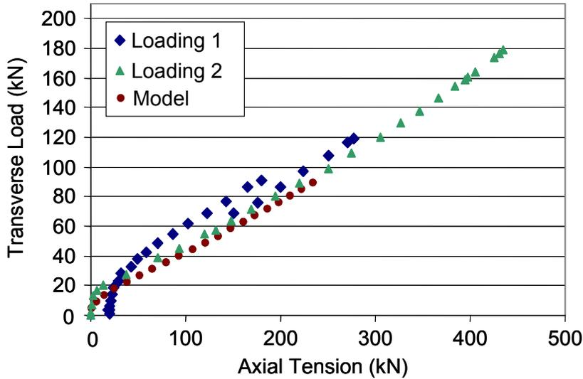
Figure 6.6 Specimen BT1 Transverse Load vs. Axial Tension
