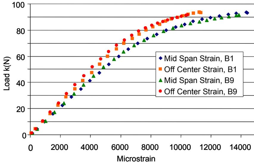
Figure 4.5: Load-Strain Response
