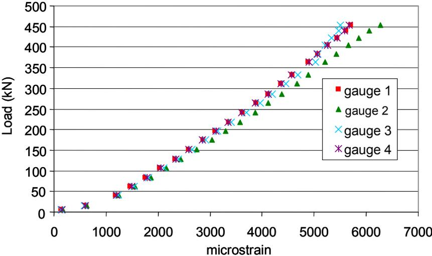
Figure 5.8 Load-Strain Relation for Specimen T3
