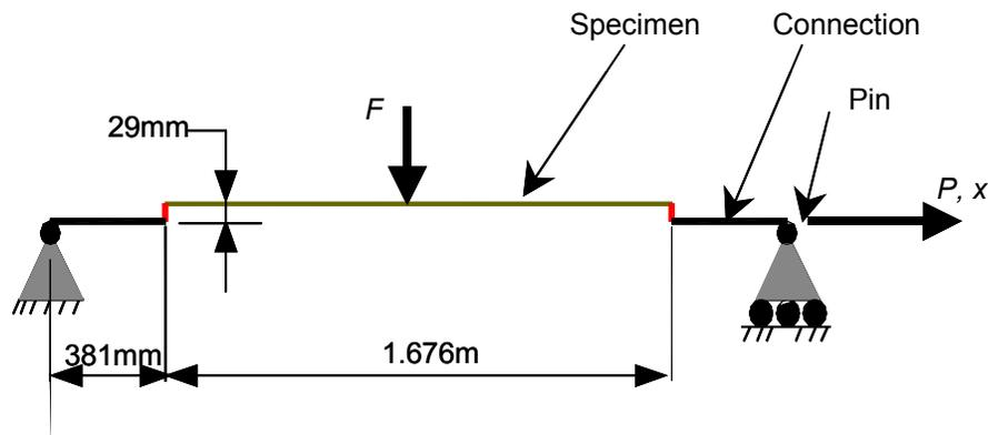
Figure 6.2 Idealization and Geometry of Combined Bending-Tension Test
