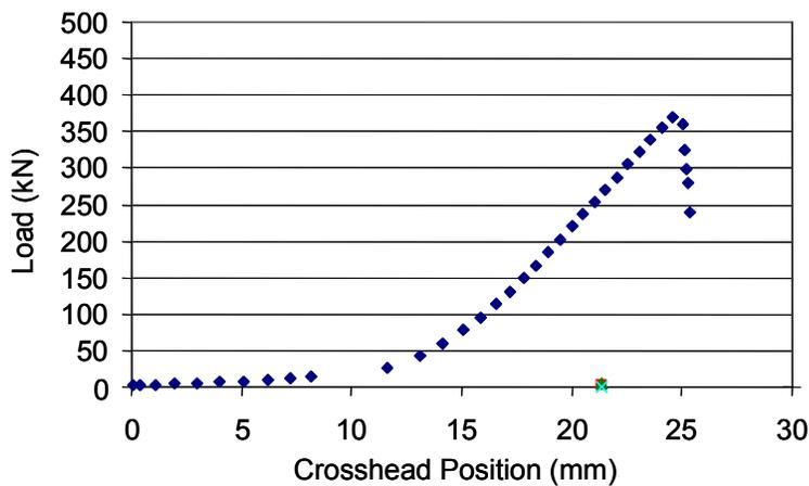
Figure 5.15 Load vs. Crosshead Position for Specimen T6
