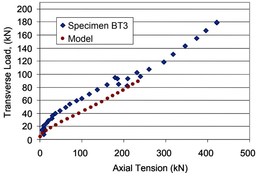
Figure 6.13 Specimen BT3 Transverse Load vs. Axial Tension
