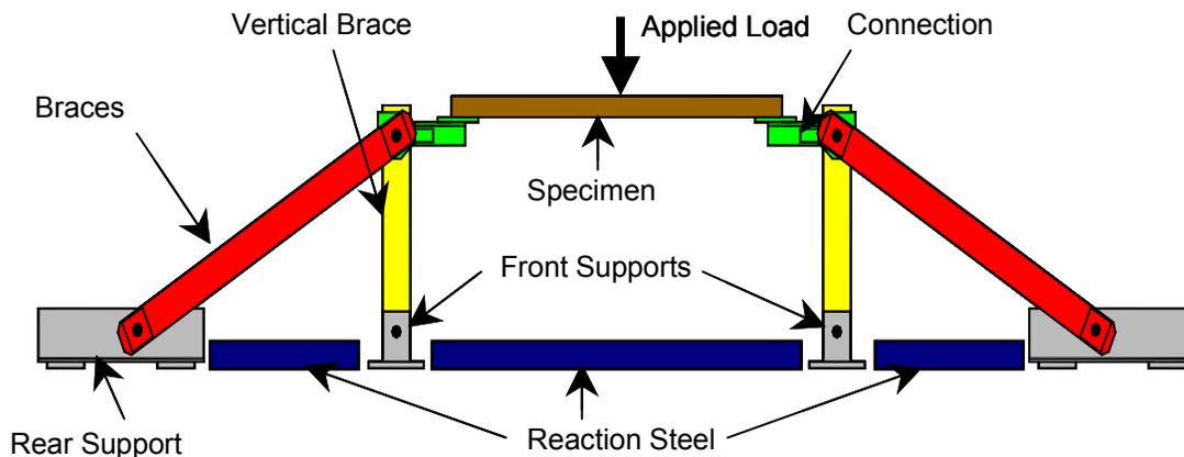
Figure 6.1 Combined Bending and Tension Reaction Fixture
