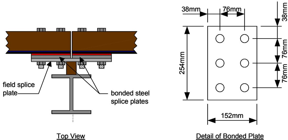
Figure 5.1: Splice Connection
