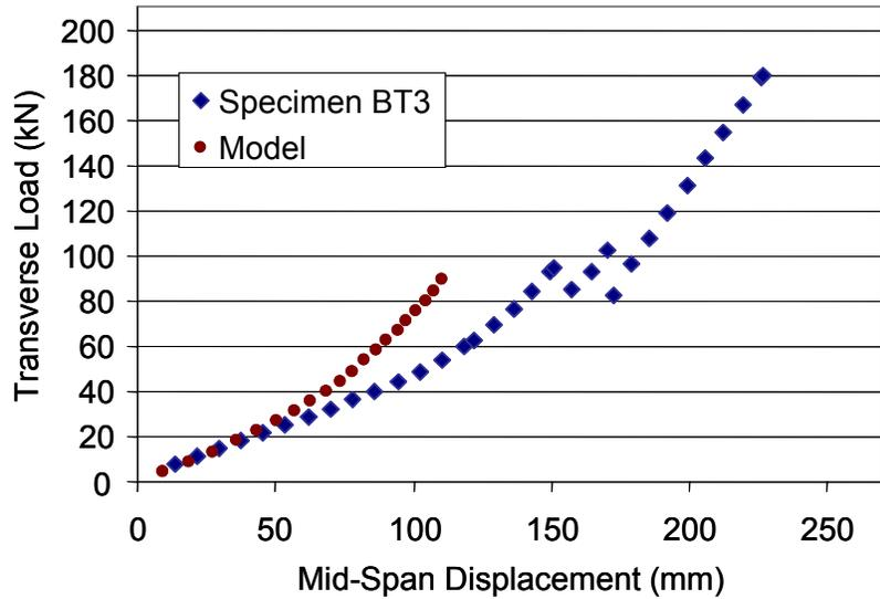
Figure 6.12 Specimen BT3 Load-Displacement
