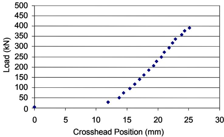
Figure 5.13 Load vs. Crosshead Position for Specimen T5
