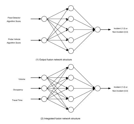
**Figure 1-4** Two neural network structures fusing fixed detector and probe vehicle data (Source: Ivan *et al.*, 1995)
