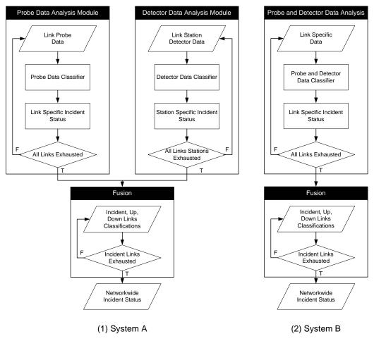
**Figure 1-6** Multi-state and multi-sensor arterial incident detection systems (Source: Thomas, 1998)
