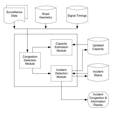
Figure 1-8 Congestion-oriented incident detection system (Source: Rau and Tarko, 2000)
