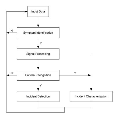
**Figure 1-10** MSRPT-based arterial incident detection system architecture (Source: Sheu and Ritchie, 1998)
