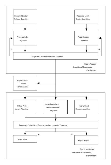
**Figure 1-3** A compound loop detector and probe vehicle incident detection system (Source: Westman *et al.*, 1996)
