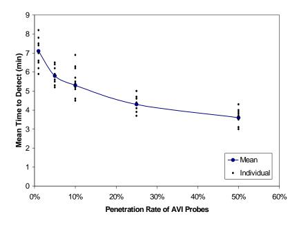
(3) Mean time to detect versus probe penetration rate
