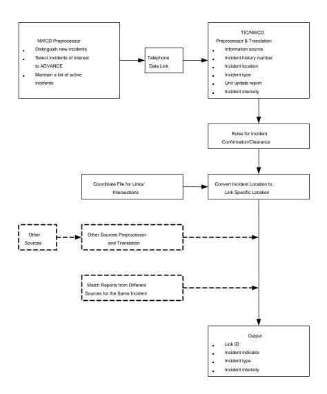
**Figure 1-2** Example anecdotal incident detection algorithm configuration (Source: Bhandari *et al.*, 1995)
