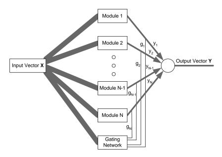
**Figure 1-9** Modular neural network-based arterial incident detection architecture (Source: Khan and Ritchie, 1998)
