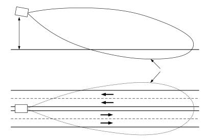
Figure 4-2 Illustration of the typical coverage of a microwave senso Receipt detection (Source: Lion and Roussel, 1995)
