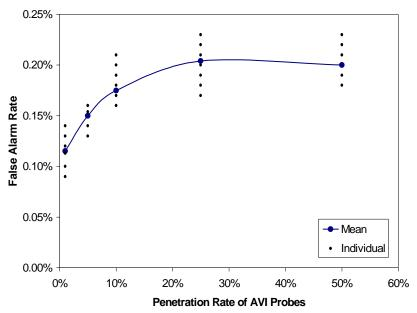
(2) False alarm rate versus probe penetration rate
