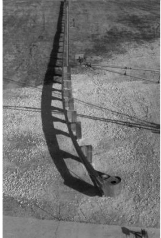
Figure 2. NETC-MELT installation prior to testing.
