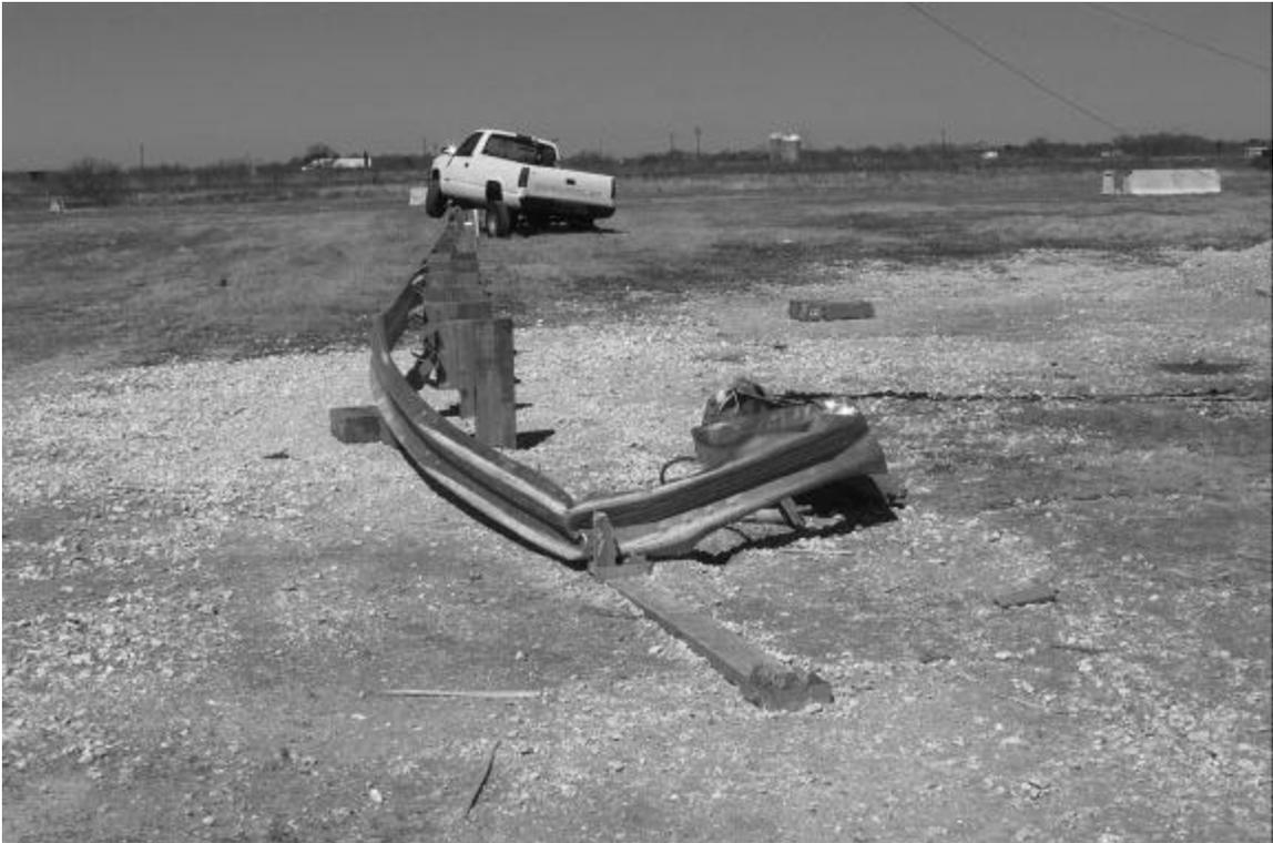
Figure 14. Vehicle trajectory after test 400401-2.
