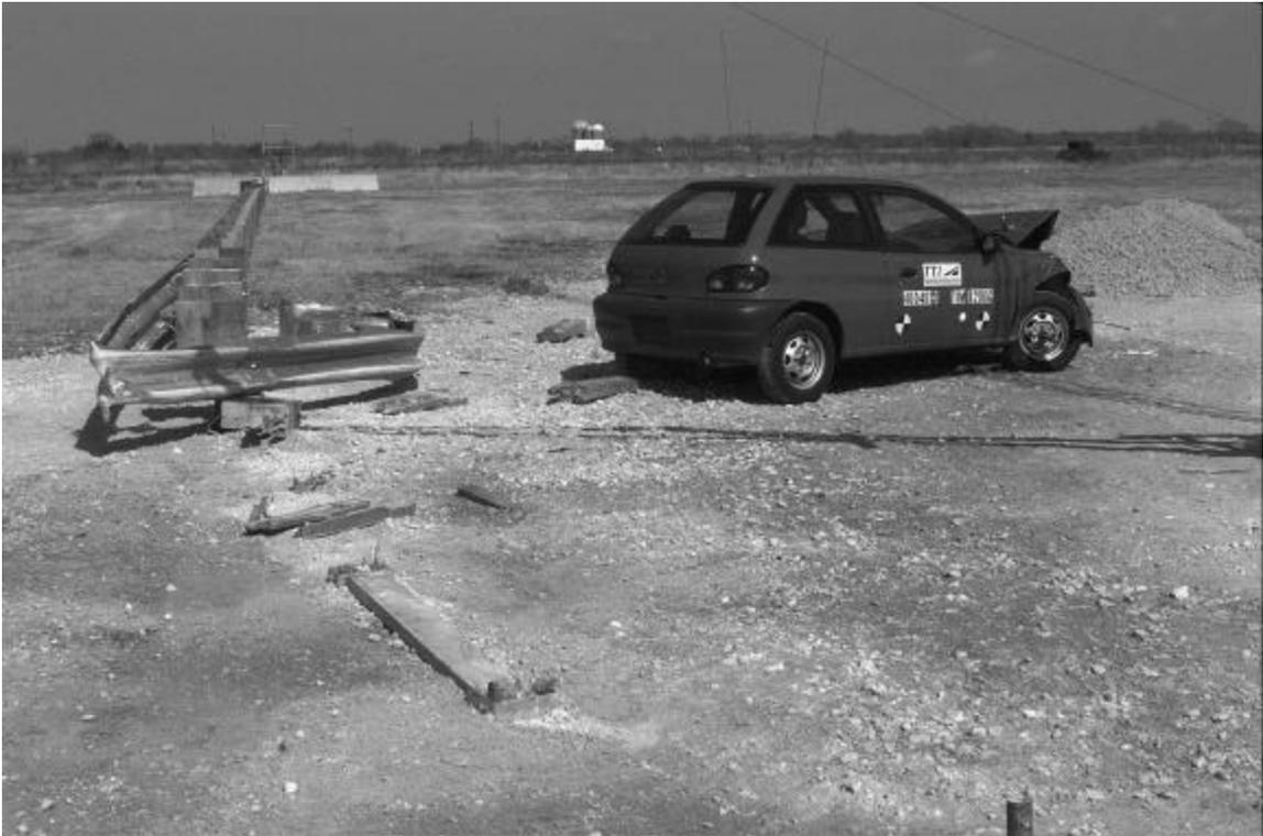
Figure 7. Vehicle trajectory after test 400401-1.
