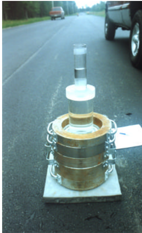
FIGURE 5.1.3 Sketch and photo of permeameter.
