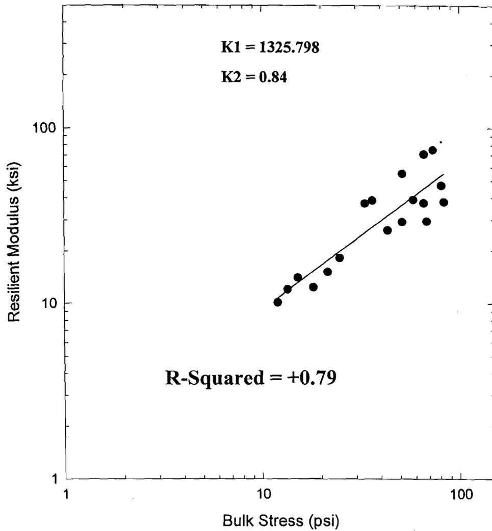
Figure 4.20 Results of Resilient Modulus Testing for Massachusetts Crushed Stone
