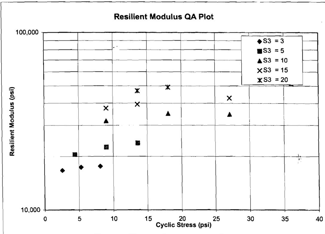
FIGURE 5.17 - Logarithmic Plot of Resilient Modulus ( $M_R$ ) vs Cyclic Stress ( $S_C$ )
