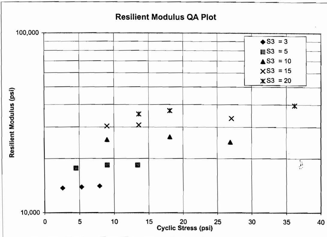
FIGURE 4.33 - Logarithmic Plot of Resilient Modulus (M<sub>R</sub>) vs Cyclic Stress (S<sub>C</sub>)
