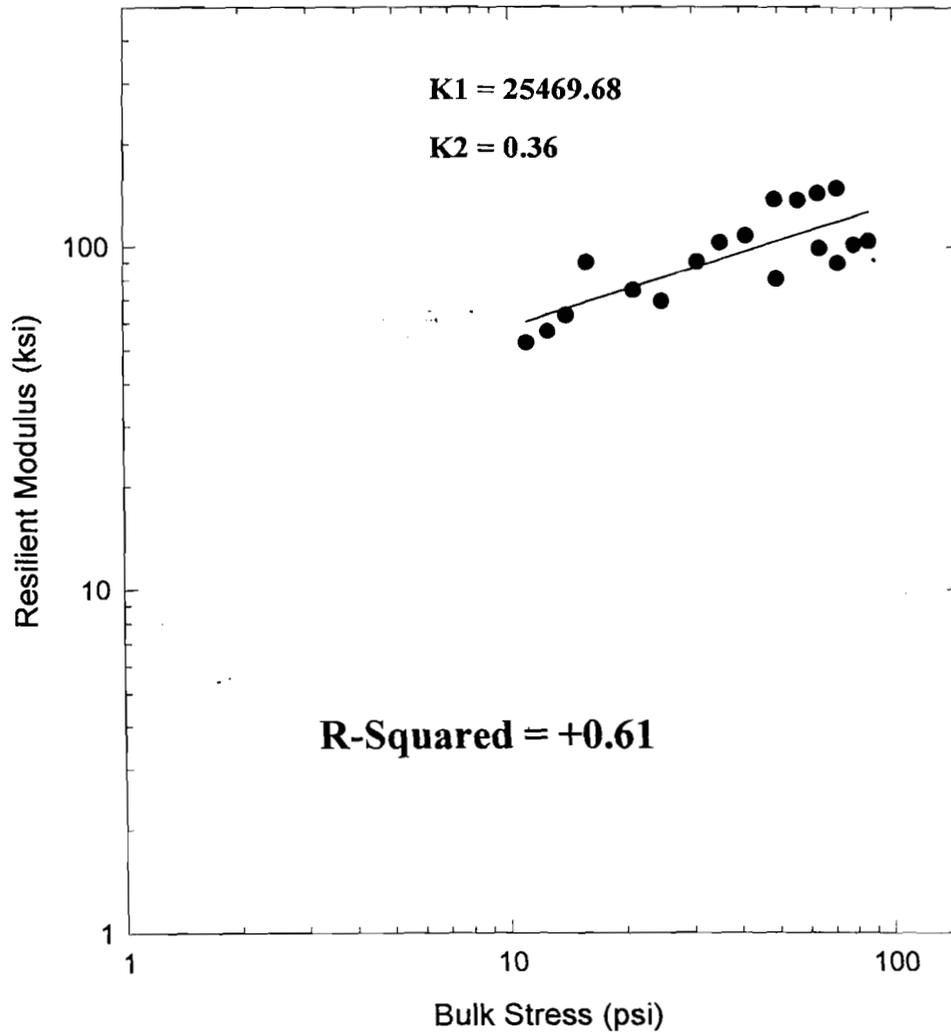
**Figure 5.16 Resilient Modulus Test Results for Massachusetts Milled Asphalt(RAP)/Processed Gravel(PG) Optimization Blend: 100(RAP)**
