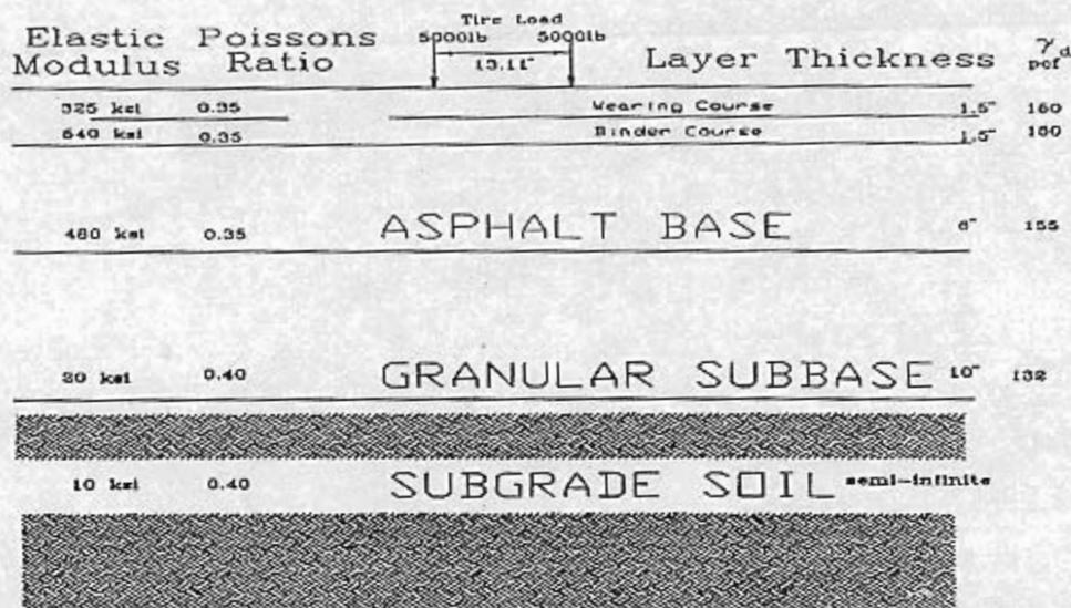
Figure 3.1 Typical Cross Section of Pavement Structure for the State of Connecticut
