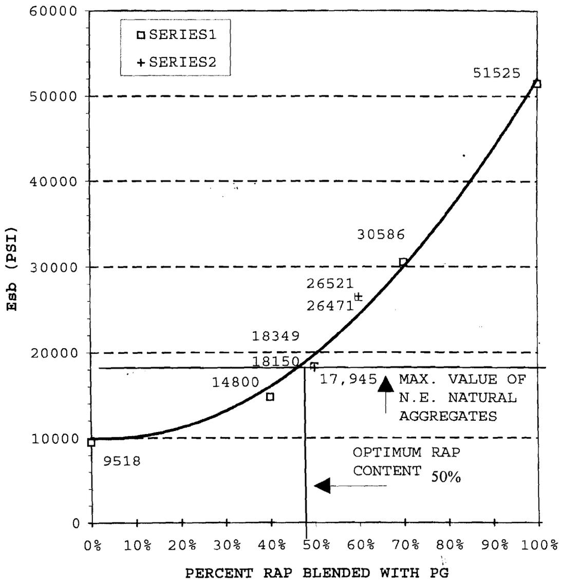
**Figure 5.26 Comparison of Lab. RAP Blends Resilient Modulus**
