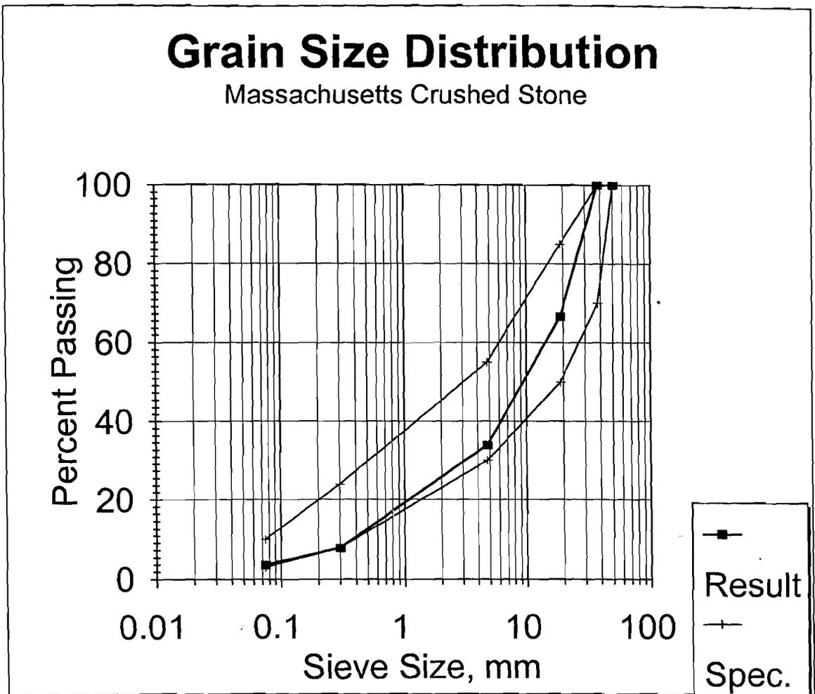
Figure 4.5 Massachusetts Crushed Stone Grain Size Distribution
