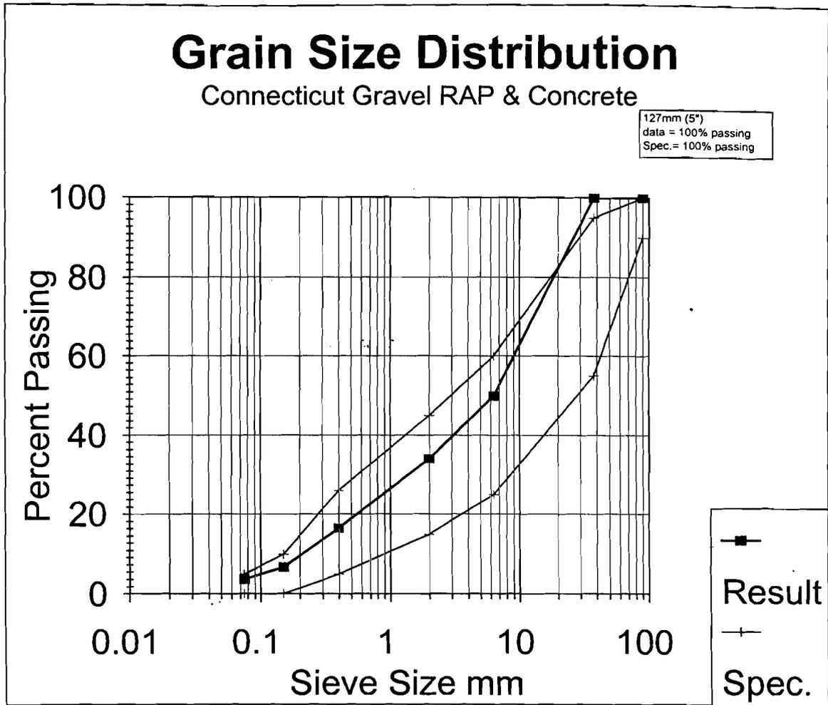
**Figure 5.1 Connecticut GRC Grain Size Distribution**
