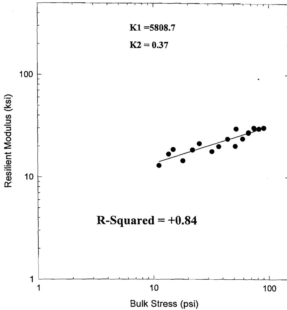
Figure 4.23 Results of Resilient Modulus Testing for Rhode Island Subbase (Route 2)
