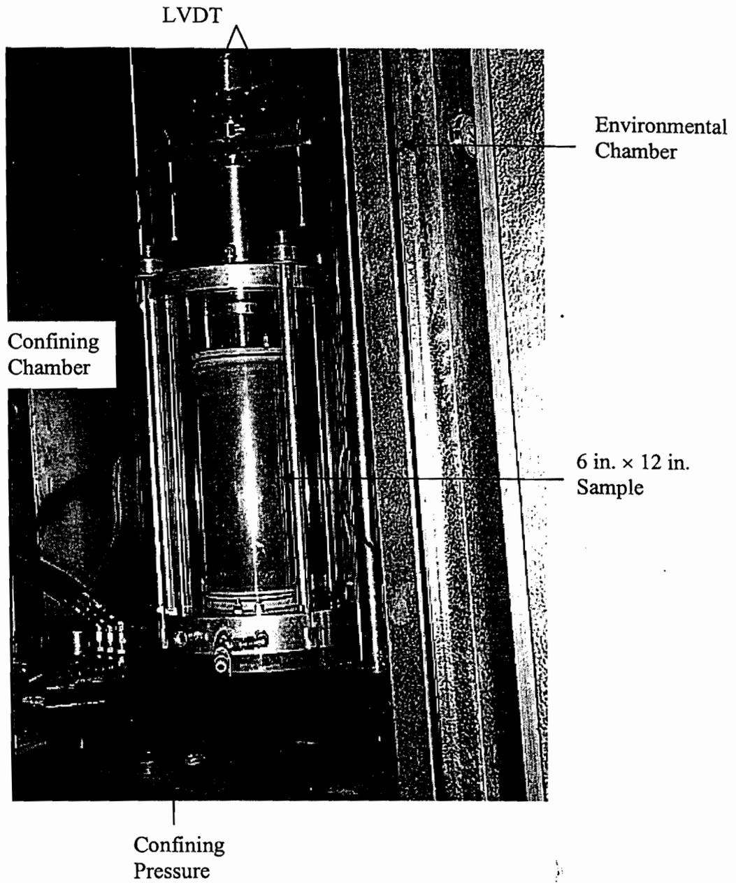
**Figure 4.28 Assembled Equipment of TP46**
