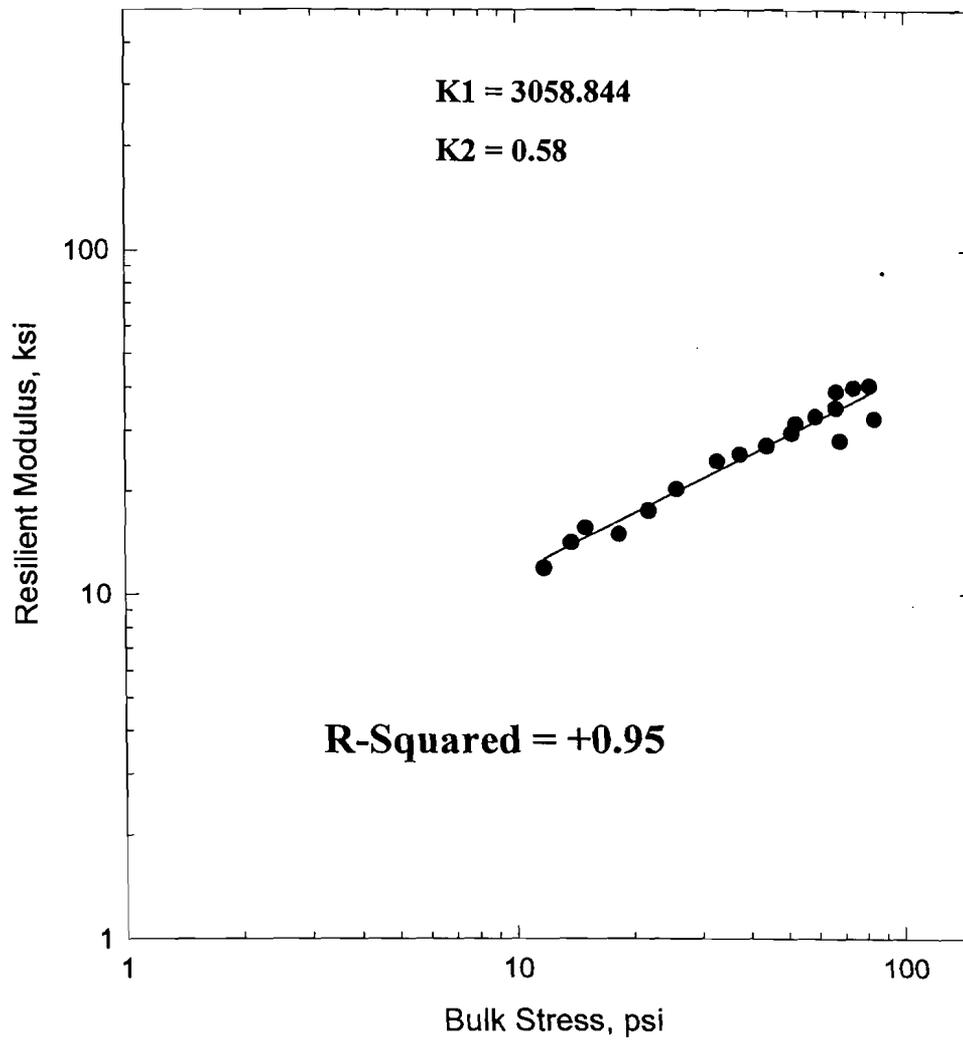
Figure 4.21 Results of Resilient Modulus Testing for Massachusetts Processed Gravel
