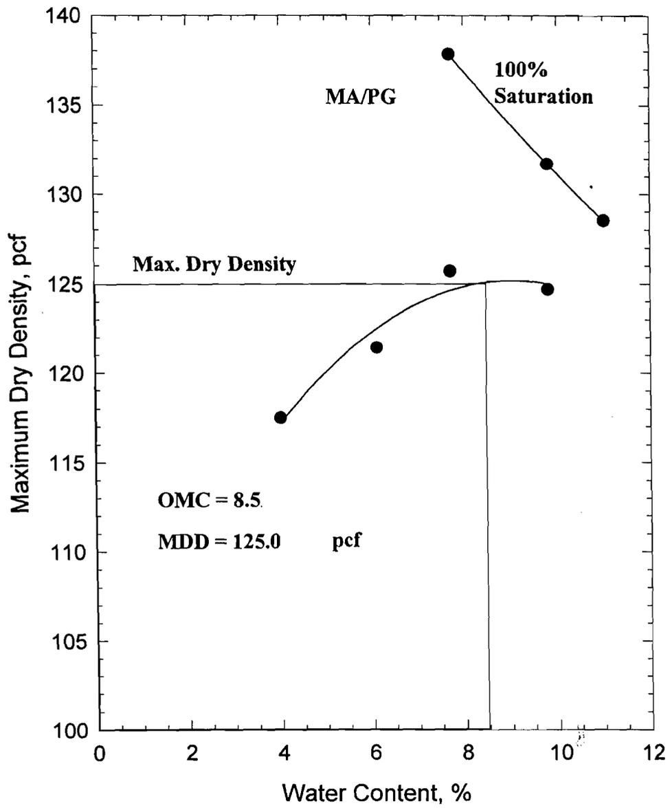
Figure 4.14 Massachusetts Processed Gravel Proctor Plot
