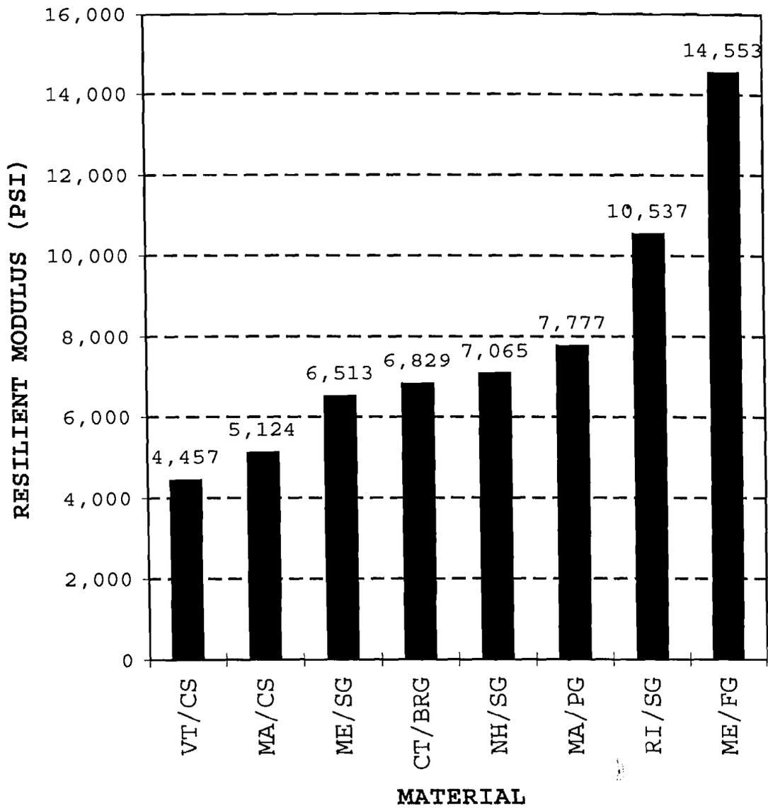
Figure 4.25 Comparison of  $E_{SB}$  with 5 psi Bulk Stress Assumed
