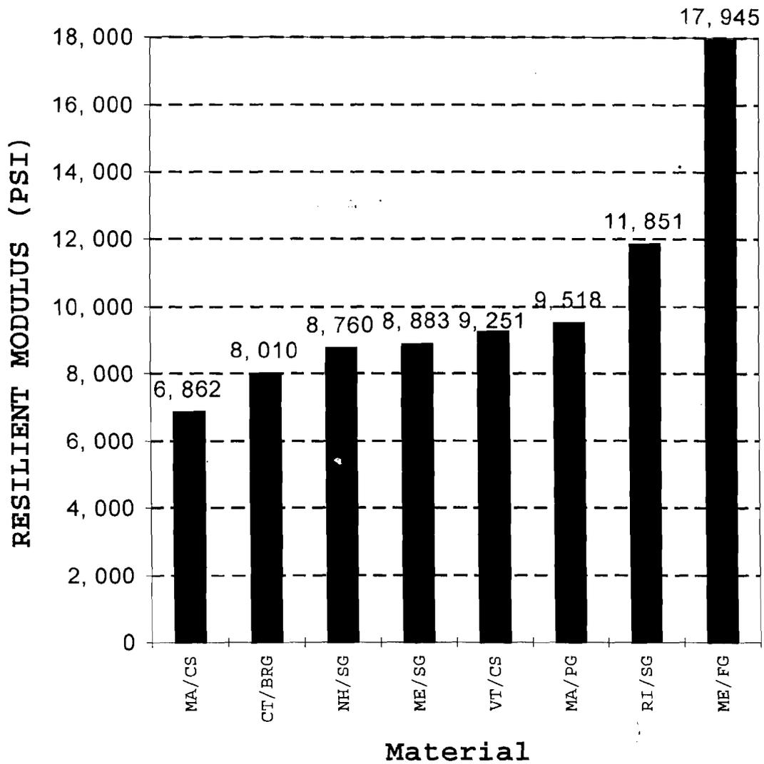
**Figure 4.44 Comparison of Resilient Moduli Determined by the AASHTO T292-91 Procedure for Granular Subbase Materials in New England**
