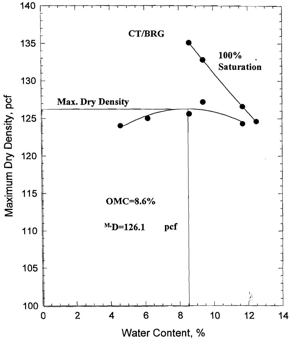
Figure 4.10 Connecticut Bank Run Gravel Proctor Plot
