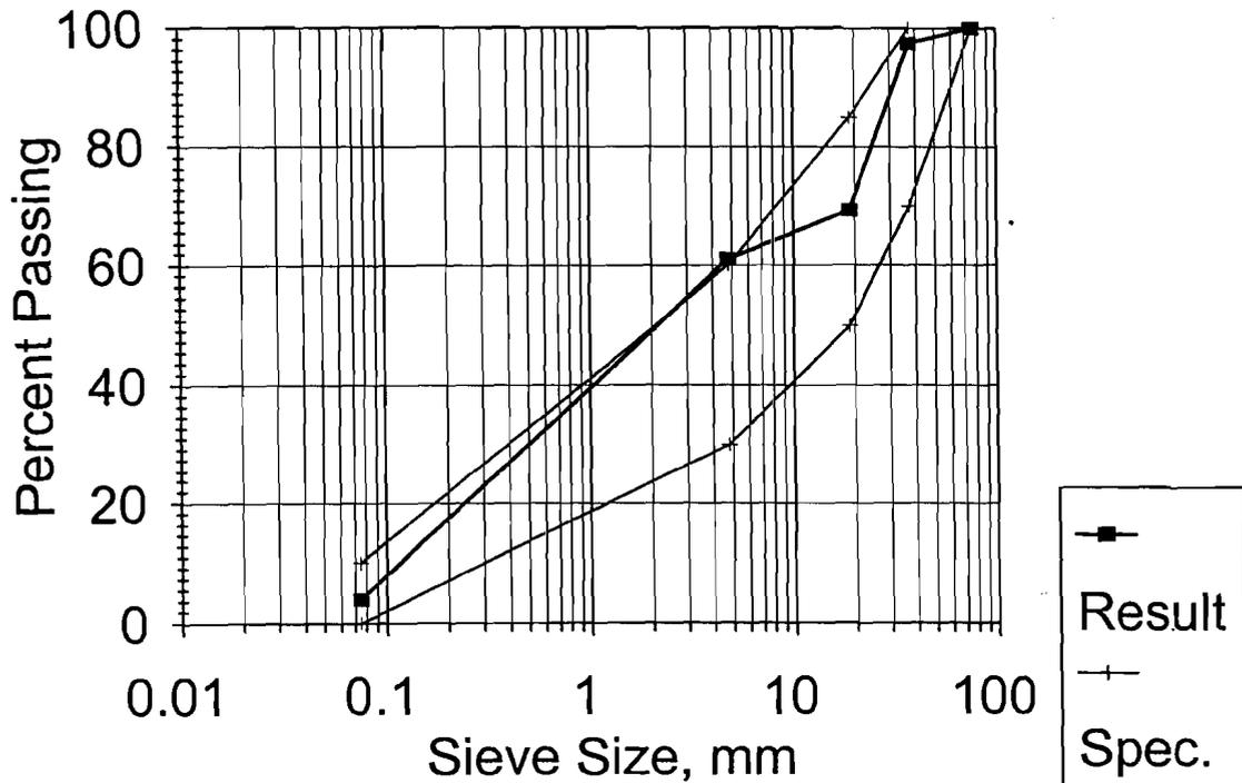
FIGURE 4.6 Massachusetts Processed Gravel Grain Size Distribution
