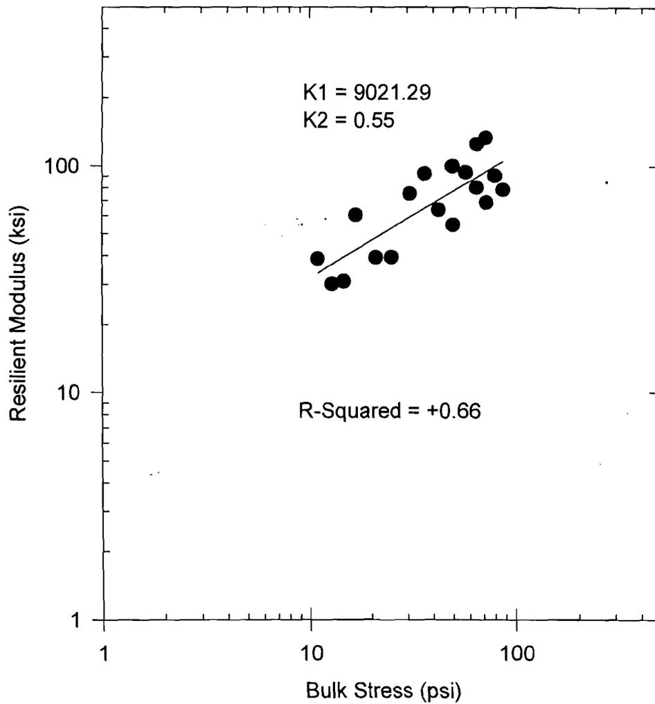
**Figure 5.14 Resilient Modulus Test Results for Massachusetts Milled Asphalt(RAP)/Processed Gravel(PG) Optimization Blend: 60(RAP)/40(PG)**
