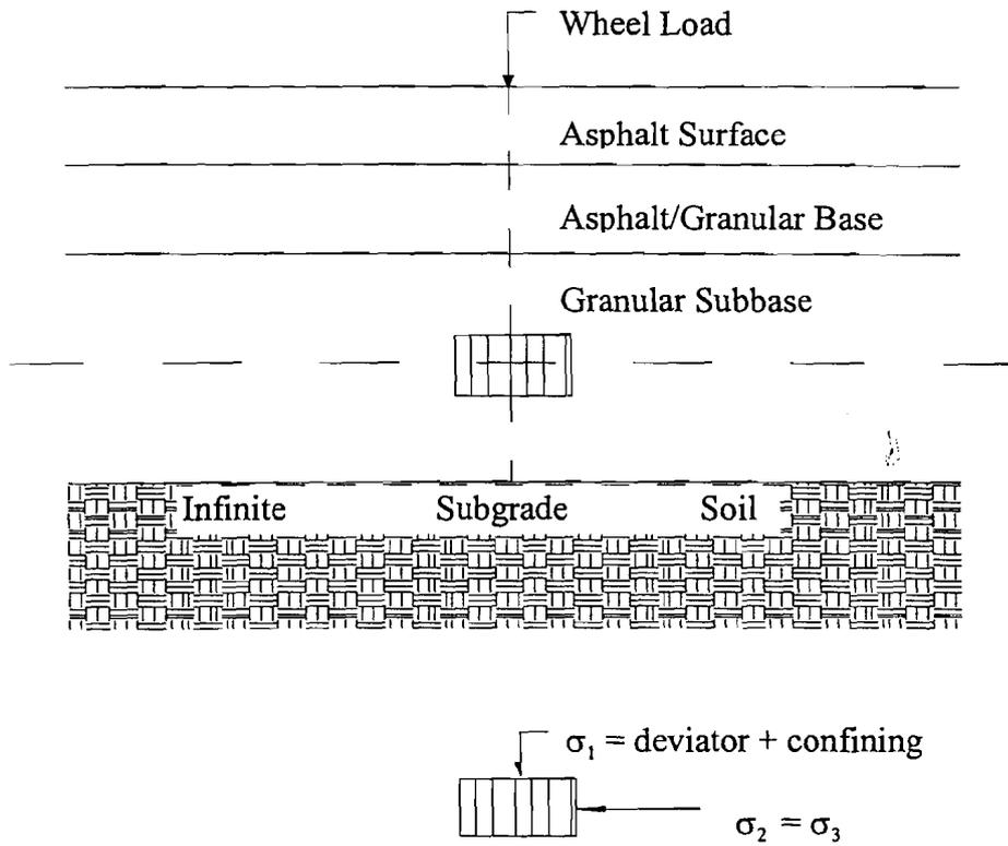
Figure 4.40 Experimental Bulk Stress and Field Condition
