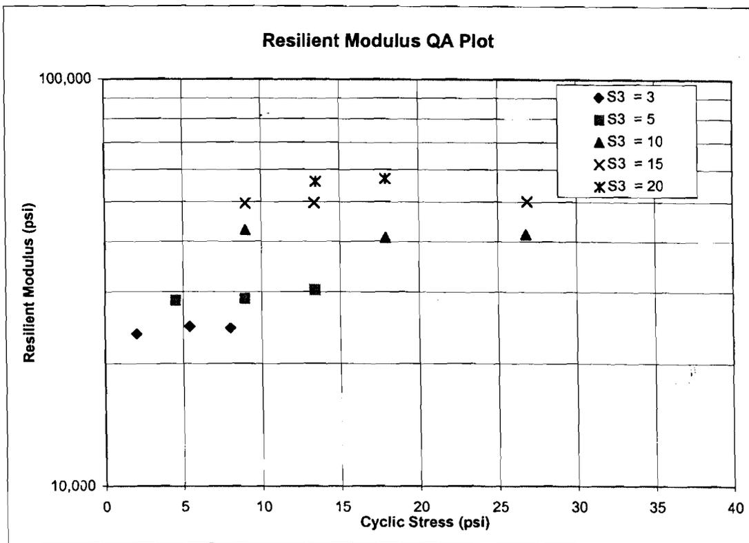
FIGURE 5.23 - Logarithmic Plot of Resilient Modulus ( $M_R$ ) vs Cyclic Stress ( $S_C$ )
