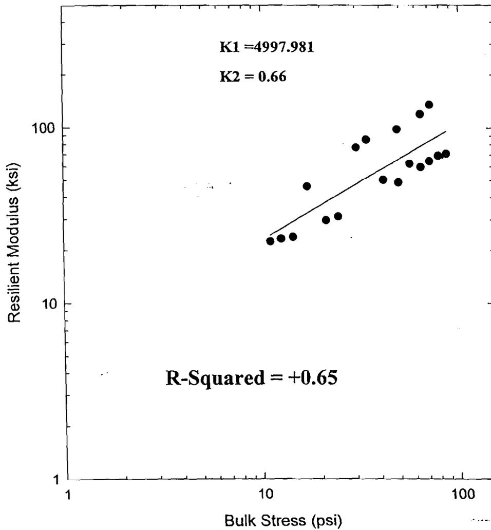
**Figure 5.13 Resilient Modulus Test Results for Massachusetts Milled Asphalt(RAP)/Processed Gravel(PG) Optimization Blend: 50(RAP)/50(PG)**
