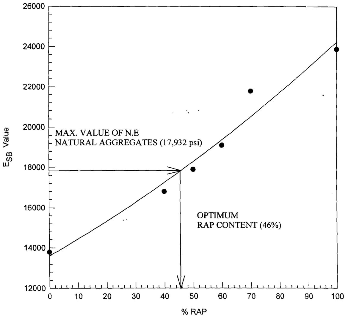
**Figure 5.27 Comparison of Lab. RAP Blends Resilient Modulus (AASHTO TP46)**
