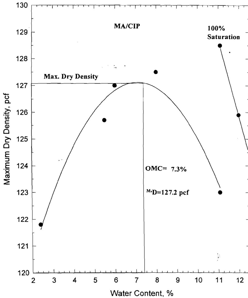
**Figure 5.4 Proctor Test Results for Massachusetts RAP**
