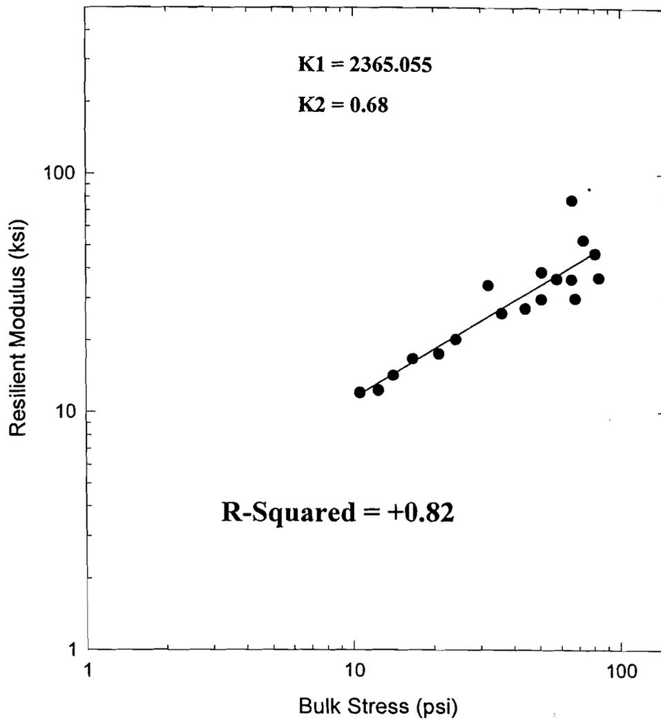
Figure 4.22 Results of Resilient Modulus Testing for New Hampshire Sandy Gravel
