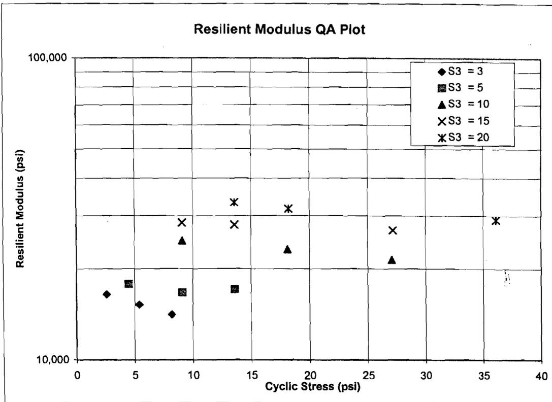
FIGURE 4.34 - Logarithmic Plot of Resilient Modulus ( $M_R$ ) vs Cyclic Stress ( $S_C$ )
