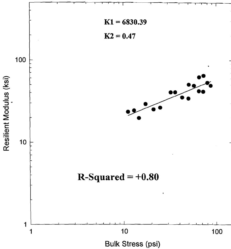
Figure 4.18 Results of Resilient Modulus Testing for Maine Frenchville Subbase
