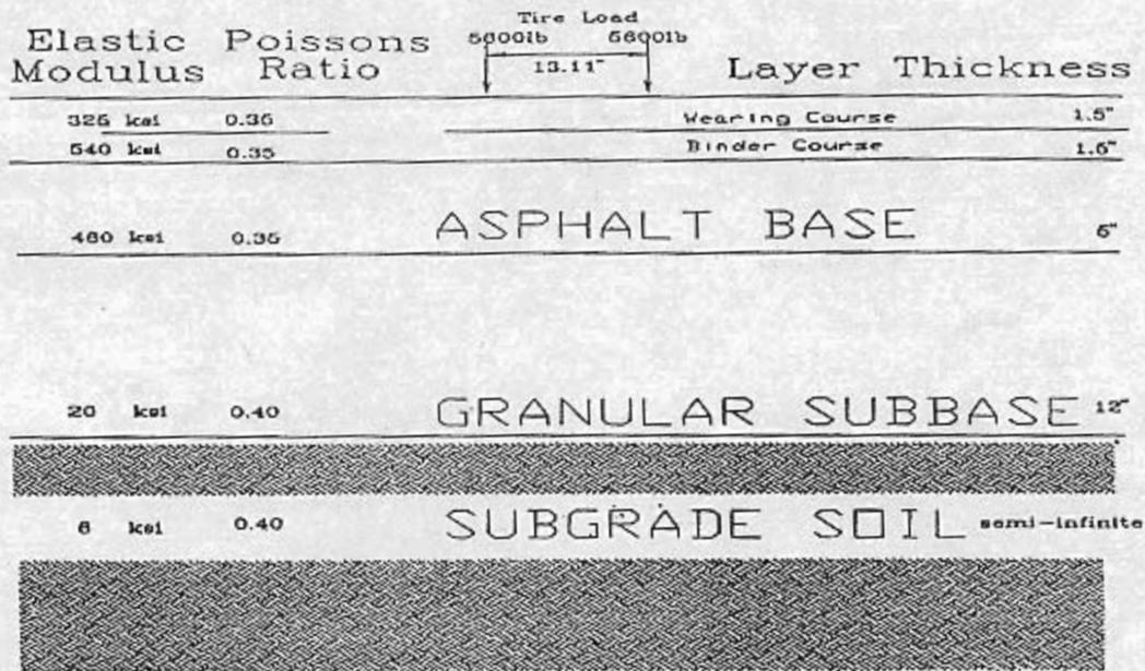
Figure 3.5 Typical Cross Section of Pavement Structure for the State of Rhode Island
