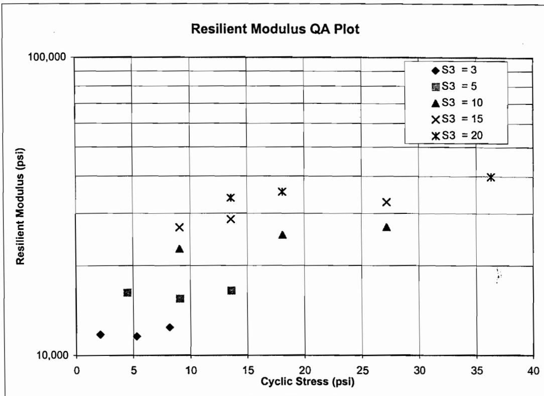
FIGURE 4.32 - Logarithmic Plot of Resilient Modulus ( $M_R$ ) vs Cyclic Stress ( $S_C$ )
