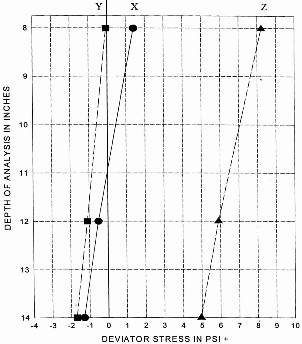
Figure 4.42 Deviator Stress in the X, Y and Z Planes as a Function of Depth for a Typical Pavement Cross Section on Rhode Island RT 2.
