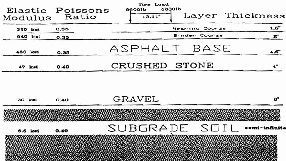
Figure 3.3 Typical Cross Section of Pavement Structure for the State of Massachusetts
