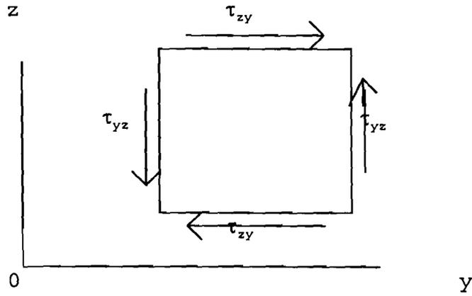
Figure 4.37 Shear Stresses on an Element
