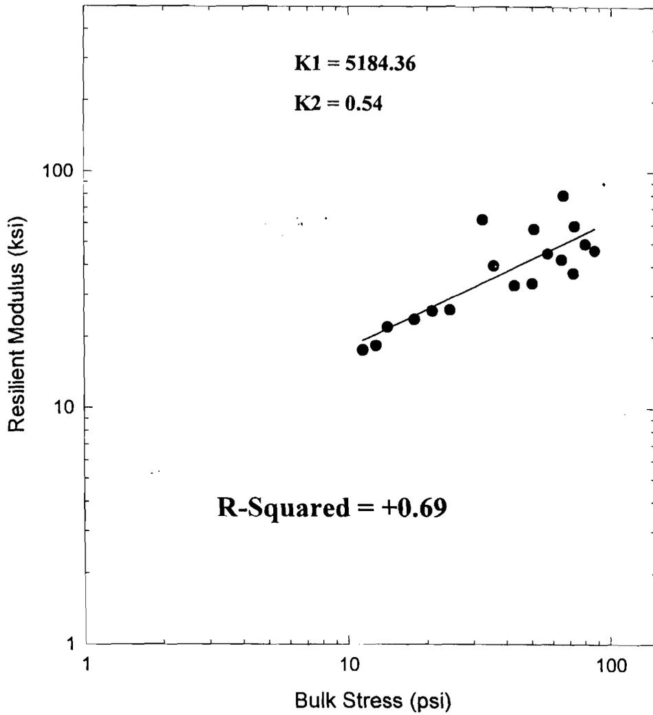
**Figure 5.10 Resilient Modulus Test Results for Connecticut
