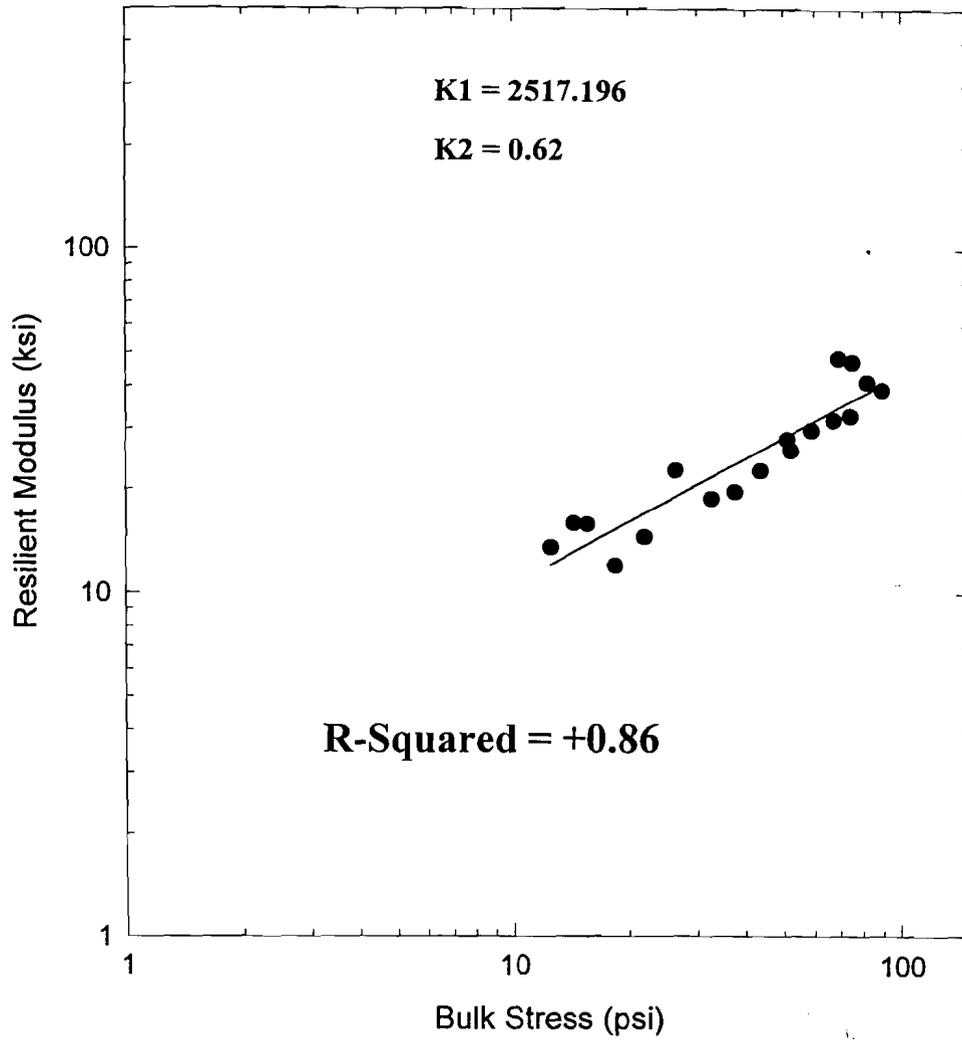
Figure 4.17 Results of Resilient Modulus Testing for Connecticut Bank Run Gravel
