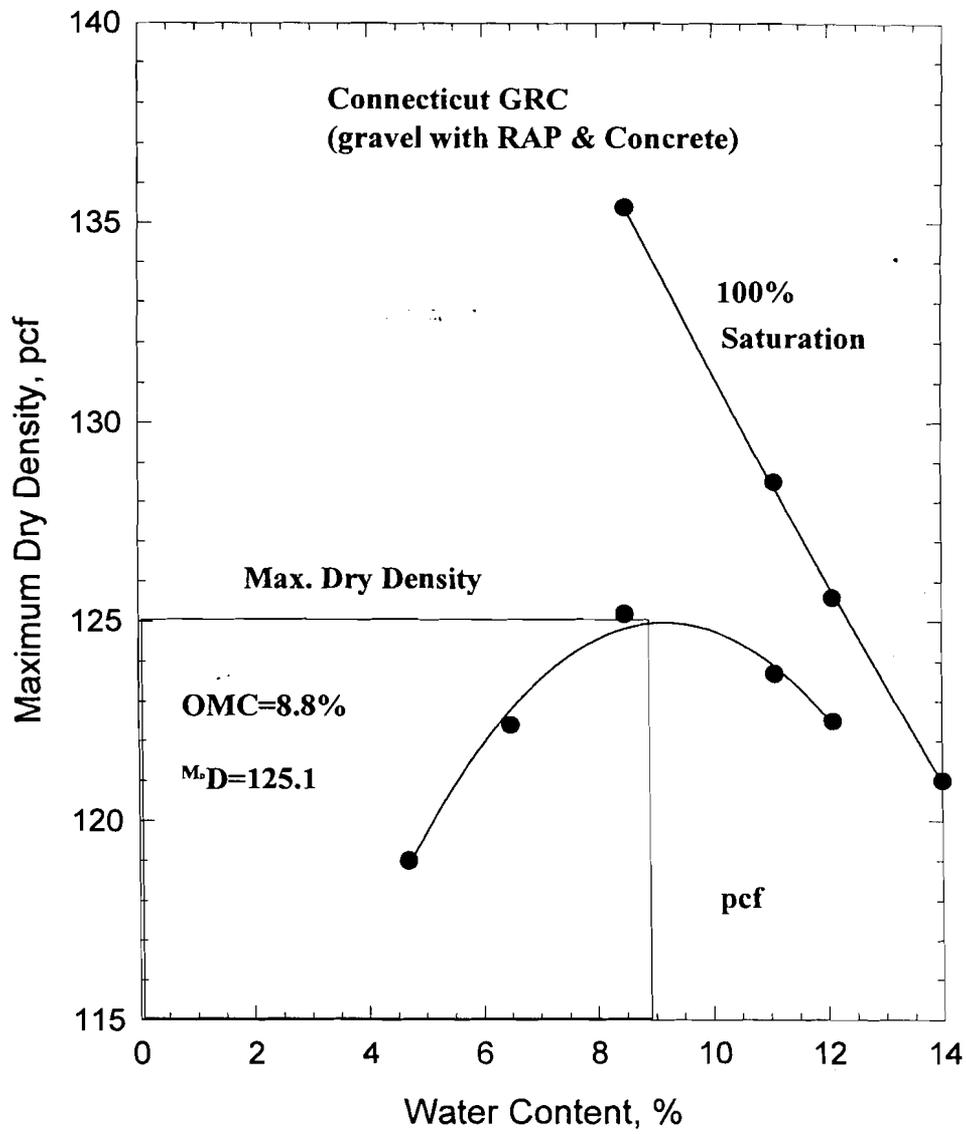
**Figure 5.3 Proctor Test Results for Connecticut GRC**
