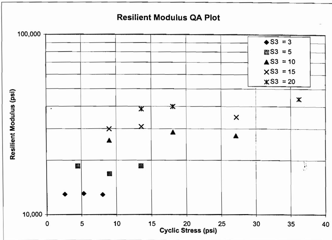
FIGURE 4.31 - Logarithmic Plot of Resilient Modulus ( $M_R$ ) vs Cyclic Stress ( $S_C$ )
