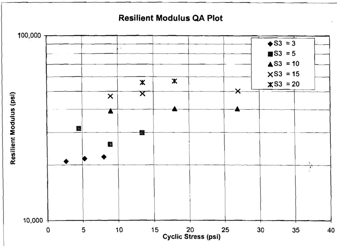
FIGURE 5.22 - Logarithmic Plot of Resilient Modulus ( $M_R$ ) vs Cyclic Stress ( $S_C$ )
