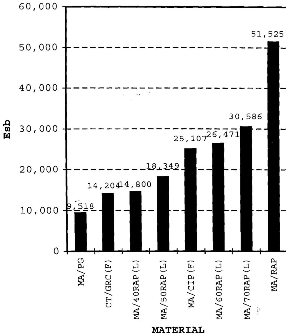
**Figure 5.24  $E_{s,b}$  Comparison for Subbase Materials with Reclaimed Materials, Bulk Stress Analyzed at Mid-depth**
