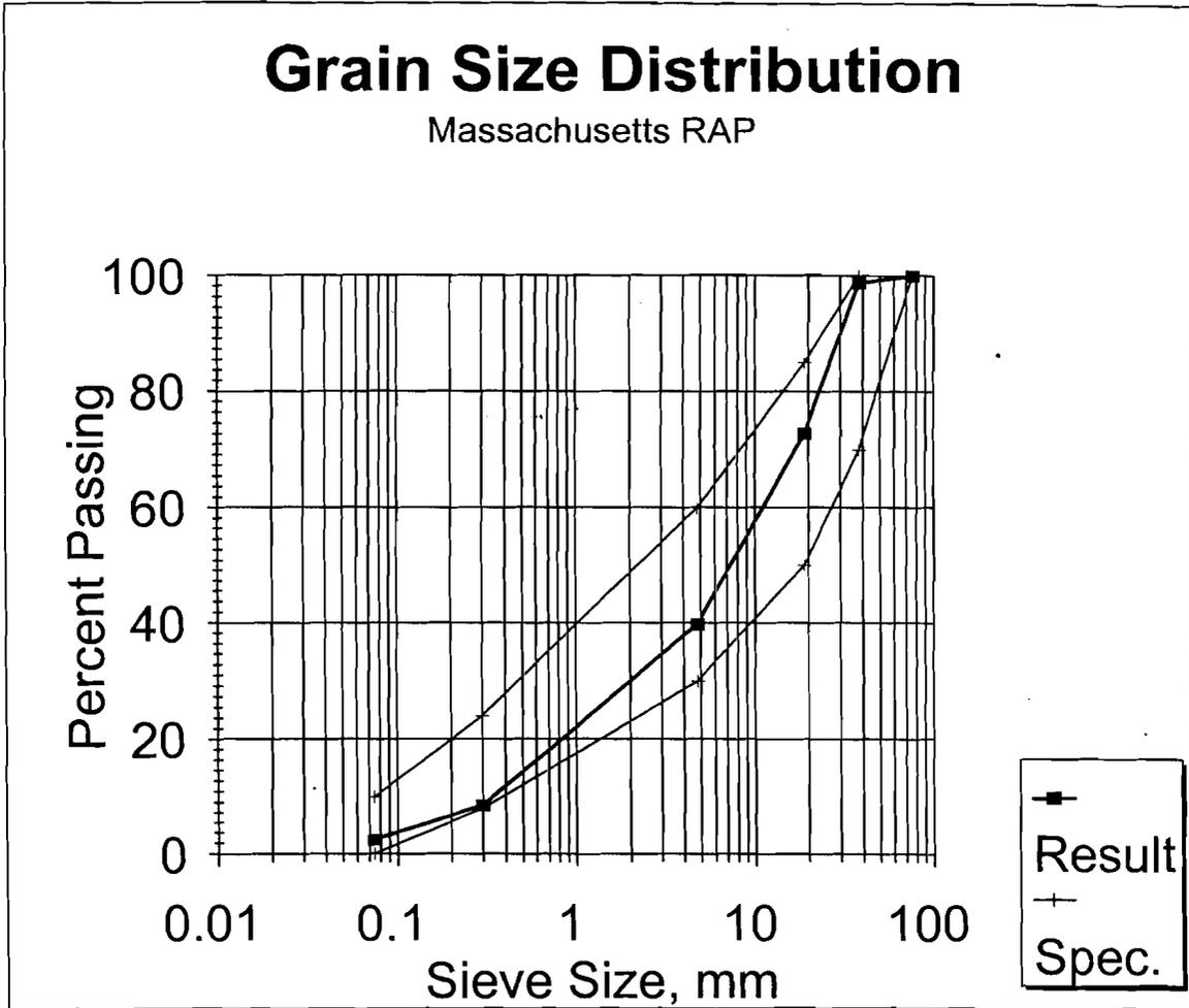
Figure 5.2 Massachusetts RAP Grain Size Distribution
