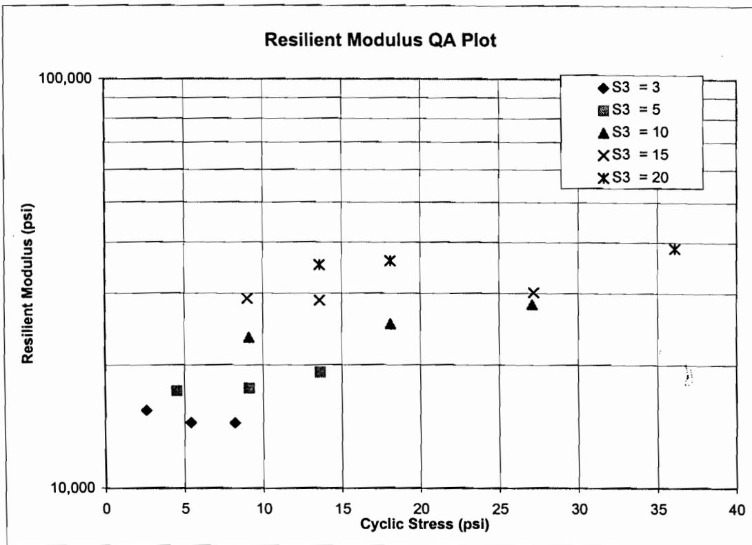
FIGURE 4.29 - Logarithmic Plot of Resilient Modulus ( $M_R$ ) vs Cyclic Stress ( $S_C$ )
