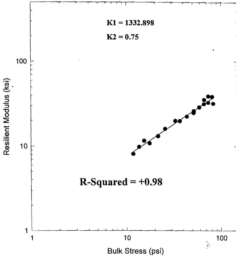
Figure 4.24 Results of Resilient Modulus Testing for Vermont Crushed Stone
