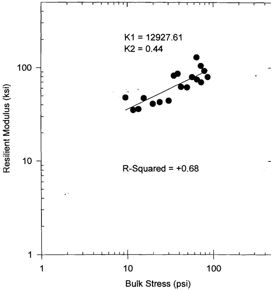
**Figure 5.15 Resilient Modulus Test Results for Massachusetts Milled Asphalt(RAP)/Processed Gravel(PG) Optimization Blend: 70(RAP)/30(PG)**
