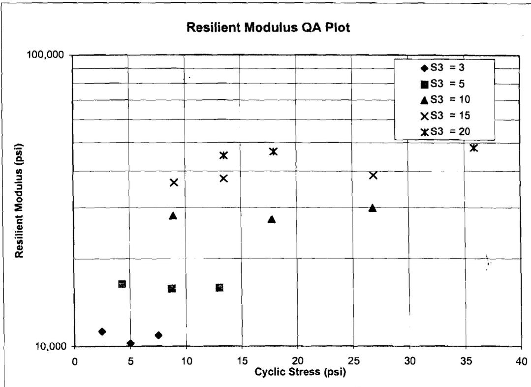
FIGURE 5.20 - Logarithmic Plot of Resilient Modulus ( $M_R$ ) vs Cyclic Stress ( $S_c$ )
