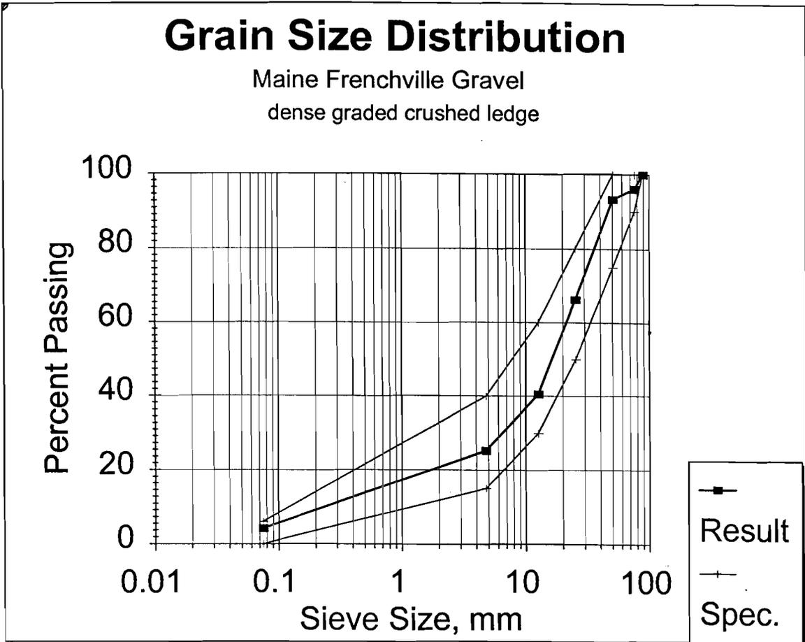
Figure 4.3 Maine Frenchville Gravel Bank Run Gravel Grain Size Distribution
