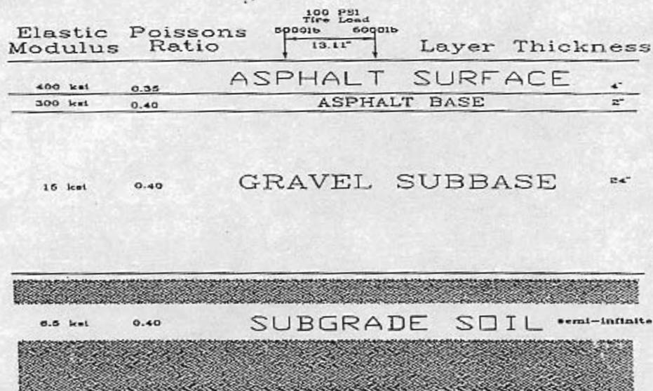
Figure 3.2 Typical Cross Section of Pavement Structure for the State of Maine
