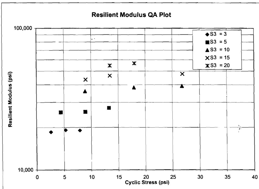
FIGURE 5.21 - Logarithmic Plot of Resilient Modulus ( $M_R$ ) vs Cyclic Stress ( $S_C$ )
