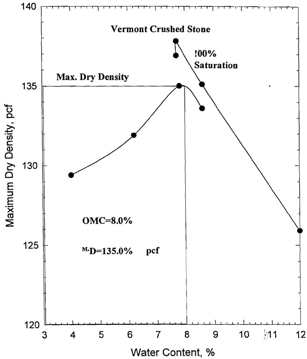
Figure 4.16 Vermont Crushed Stone Proctor Plot
