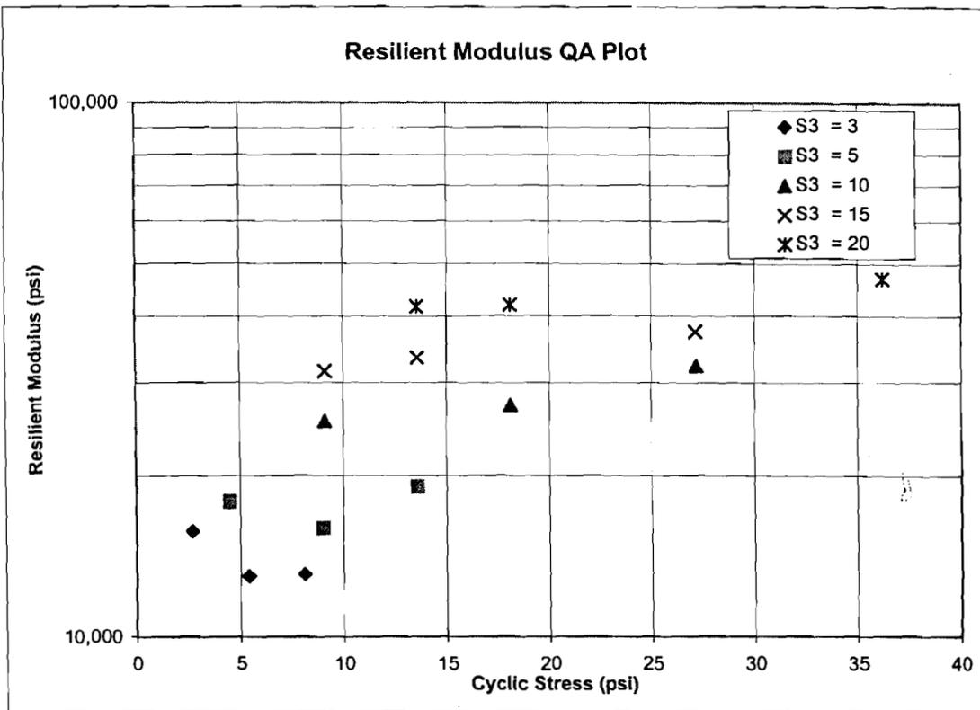
**FIGURE 4.36 - Logarithmic Plot of Resilient Modulus ( $M_R$ ) vs Cyclic Stress ( $S_C$ )**
