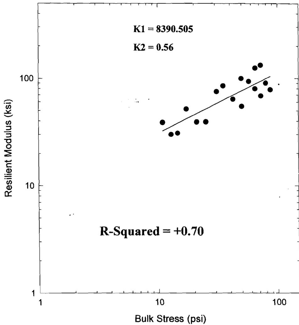
**Figure 5.11 Resilient Modulus Test results for
