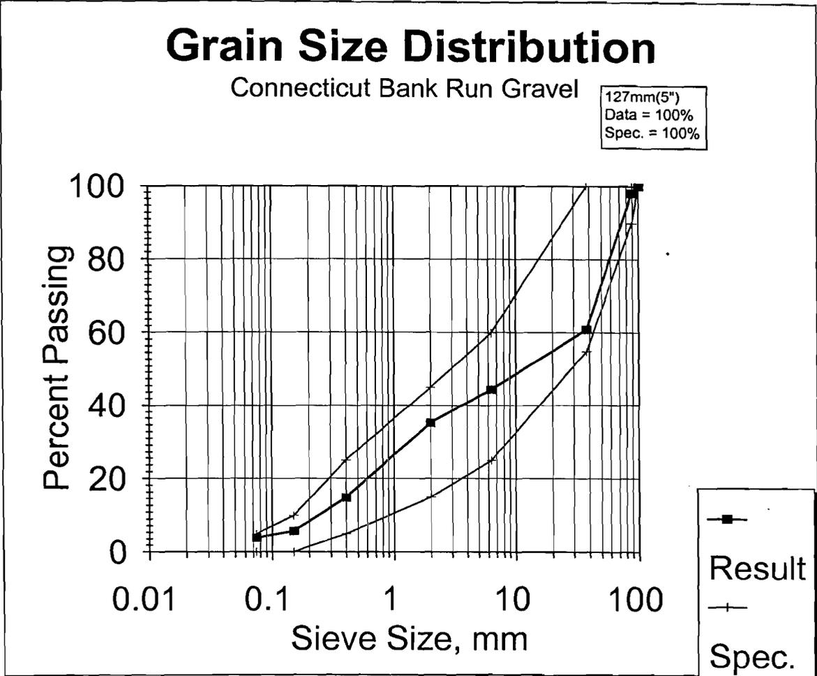
FIGURE 4.2 Connecticut Bank Run Gravel Grain Size Distribution
