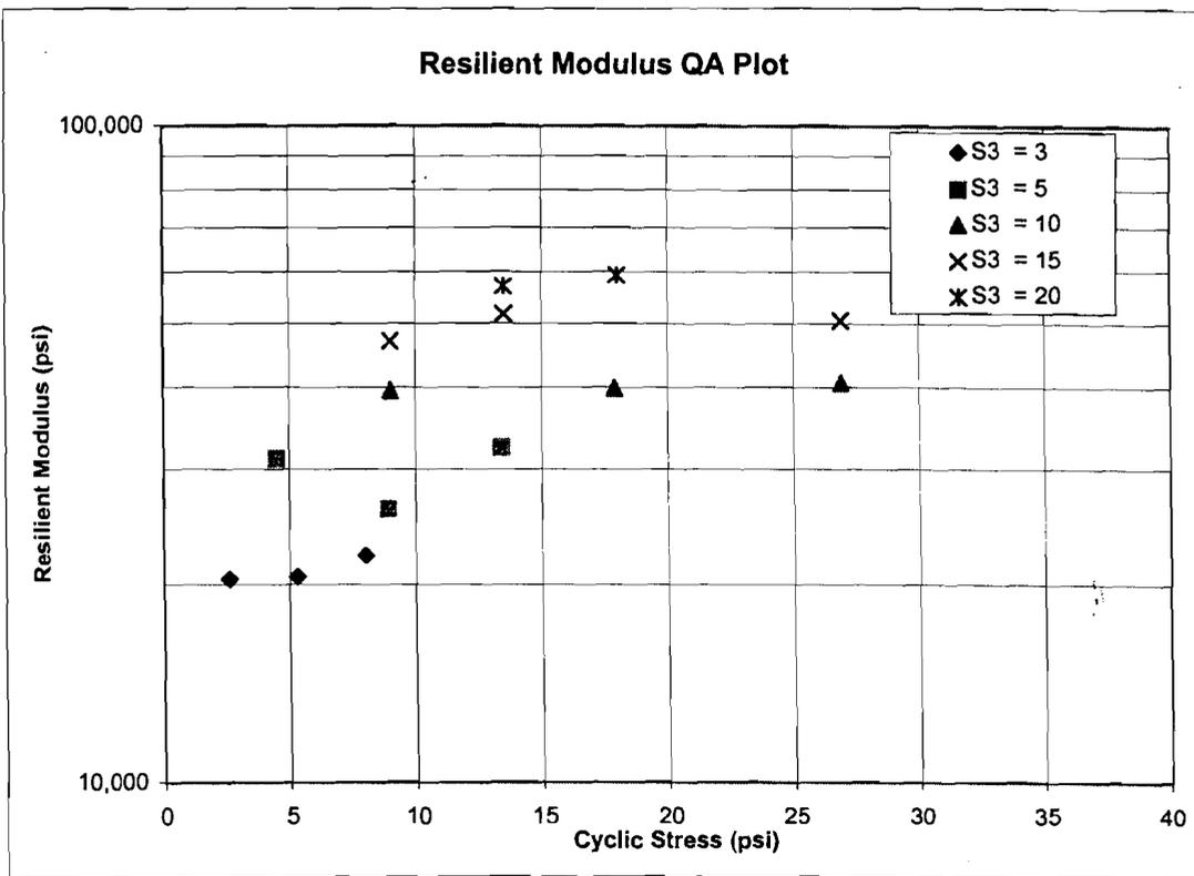
FIGURE 5.18 - Logarithmic Plot of Resilient Modulus ( $M_R$ ) vs Cyclic Stress ( $S_C$ )
