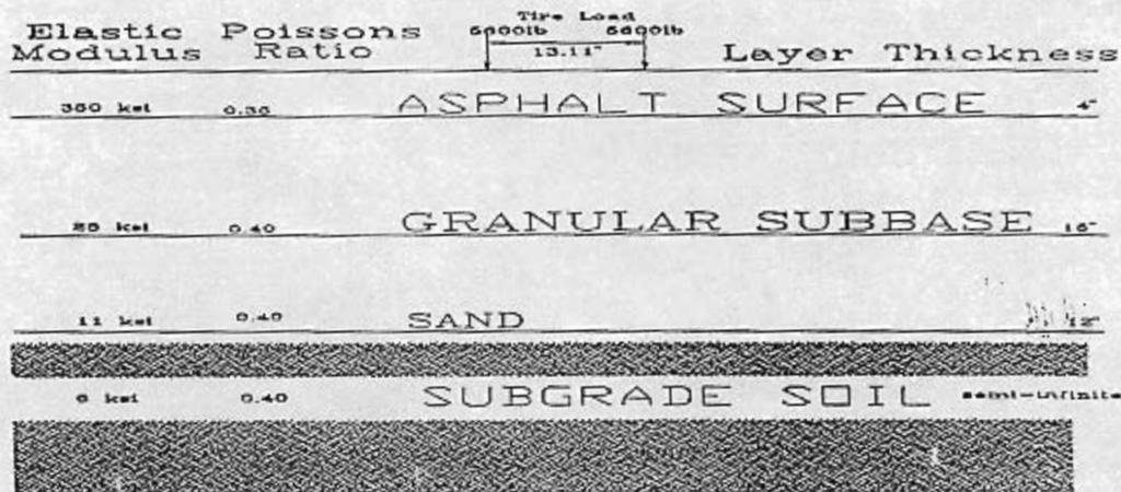
Figure 3.6 Typical Cross Section of Pavement Structure for the State of Vermont
