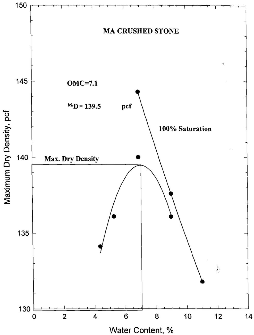
Figure 4.13 Massachusetts Crushed Stone Proctor Plot
