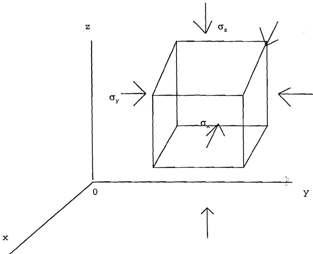
Figure 4.38 Principle Stresses on an Element
