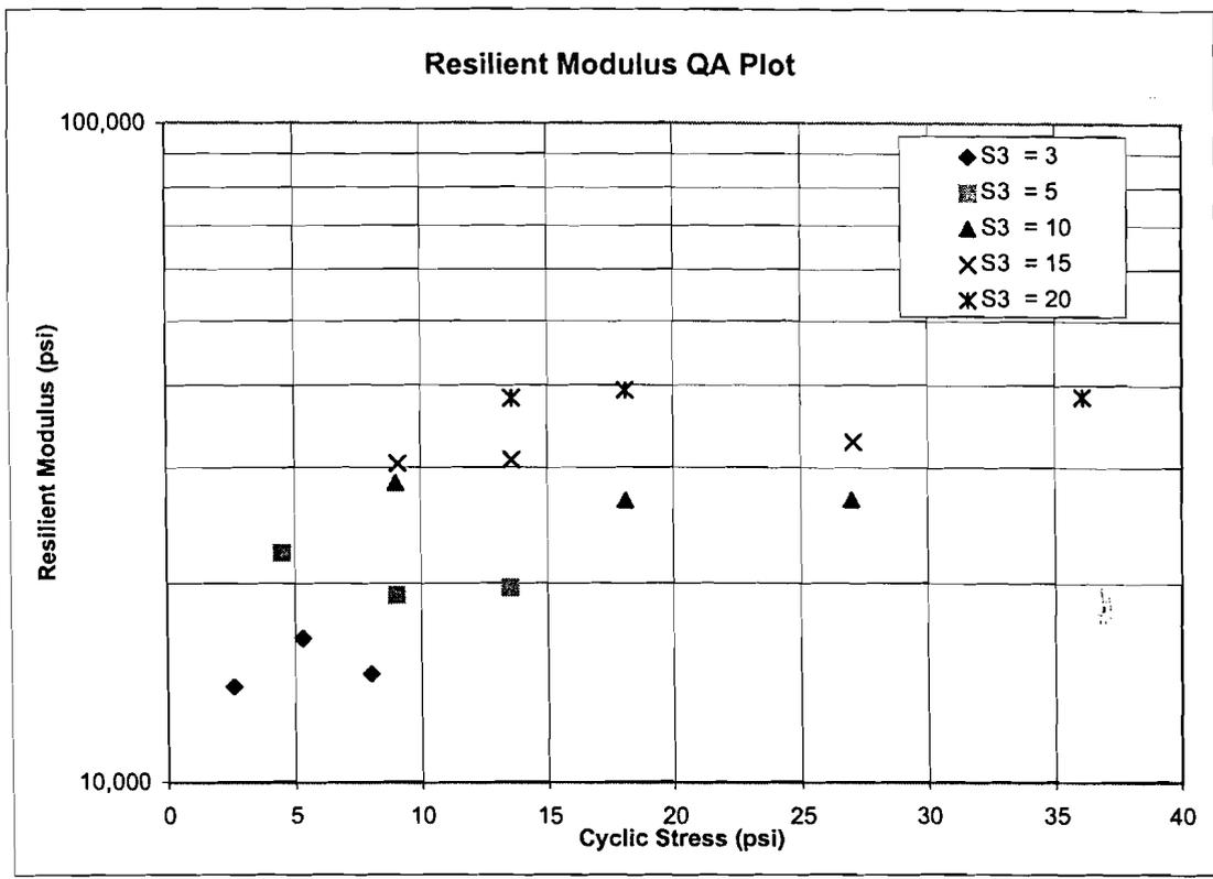
FIGURE 4.35 - Logarithmic Plot of Resilient Modulus ( $M_R$ ) vs Cyclic Stress ( $S_C$ )
