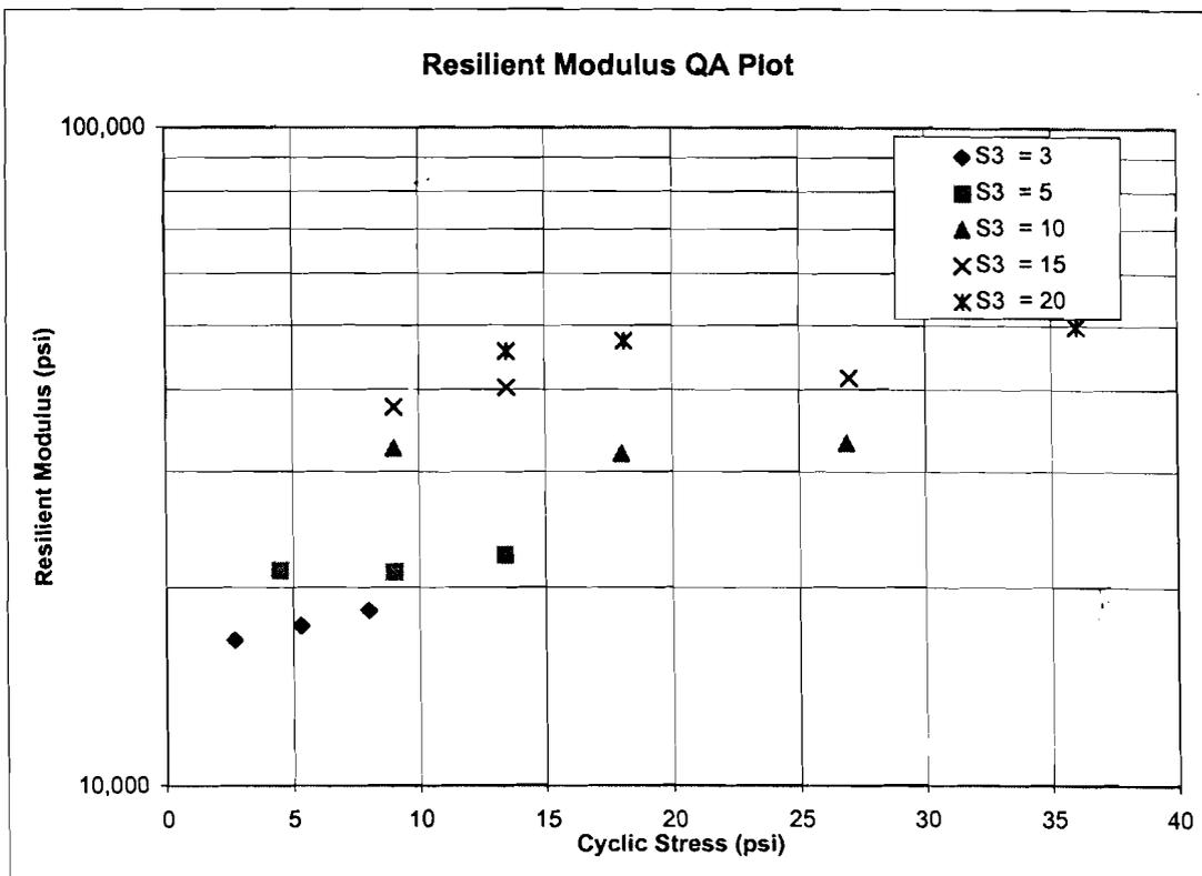
FIGURE 5.19 - Logarithmic Plot of Resilient Modulus ( $M_R$ ) vs Cyclic Stress ( $S_C$ )
