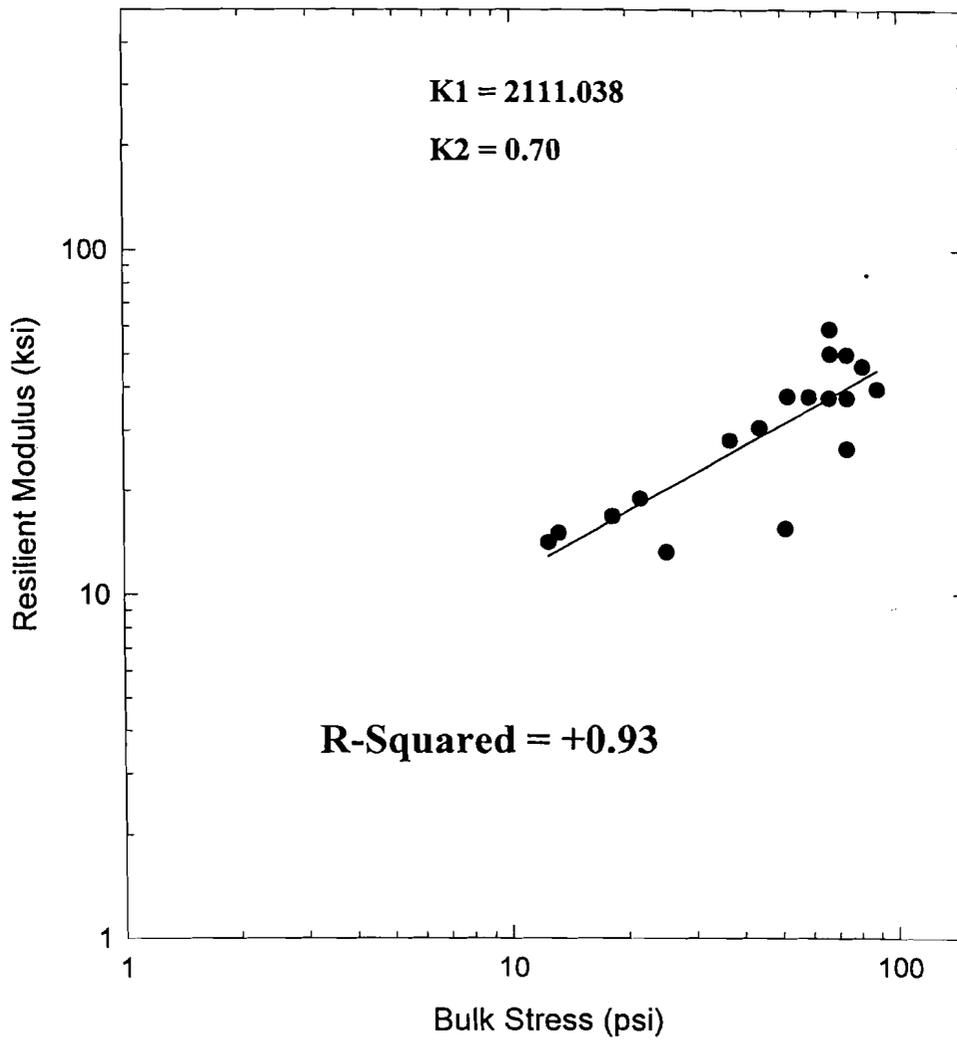
Figure 4.19 Results of Resilient Modulus Testing for Maine Sabbatus Subbase
