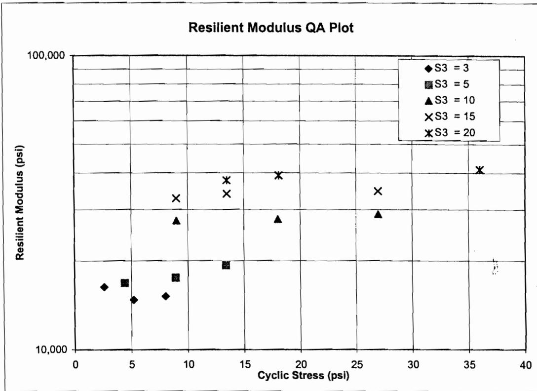
FIGURE 4-30 - Logarithmic Plot of Resilient Modulus ( $M_R$ ) vs Cyclic Stress ( $S_C$ )
