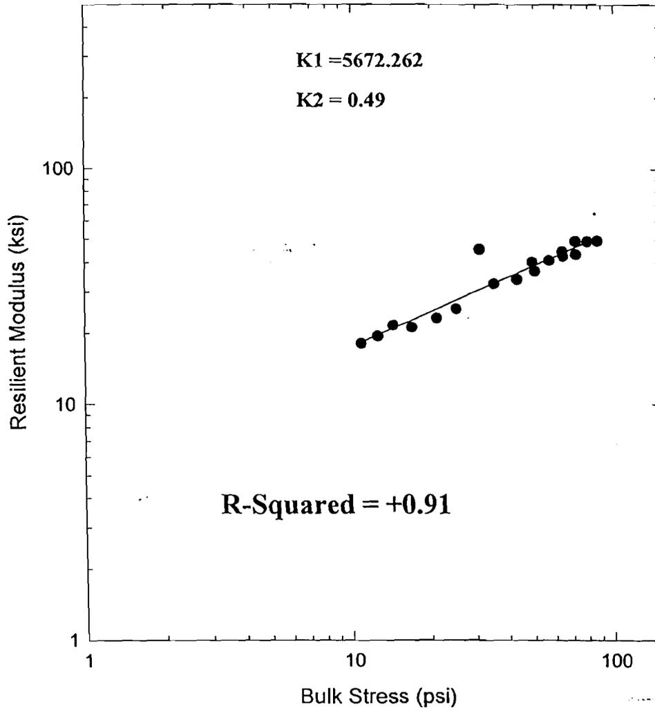
**Figure 5.12. Resilient Modulus Test Results for Massachusetts Milled Asphalt(RAP)/Processed Gravel(PG) Optimization Blend: 40(RAP)/60(PG)**
