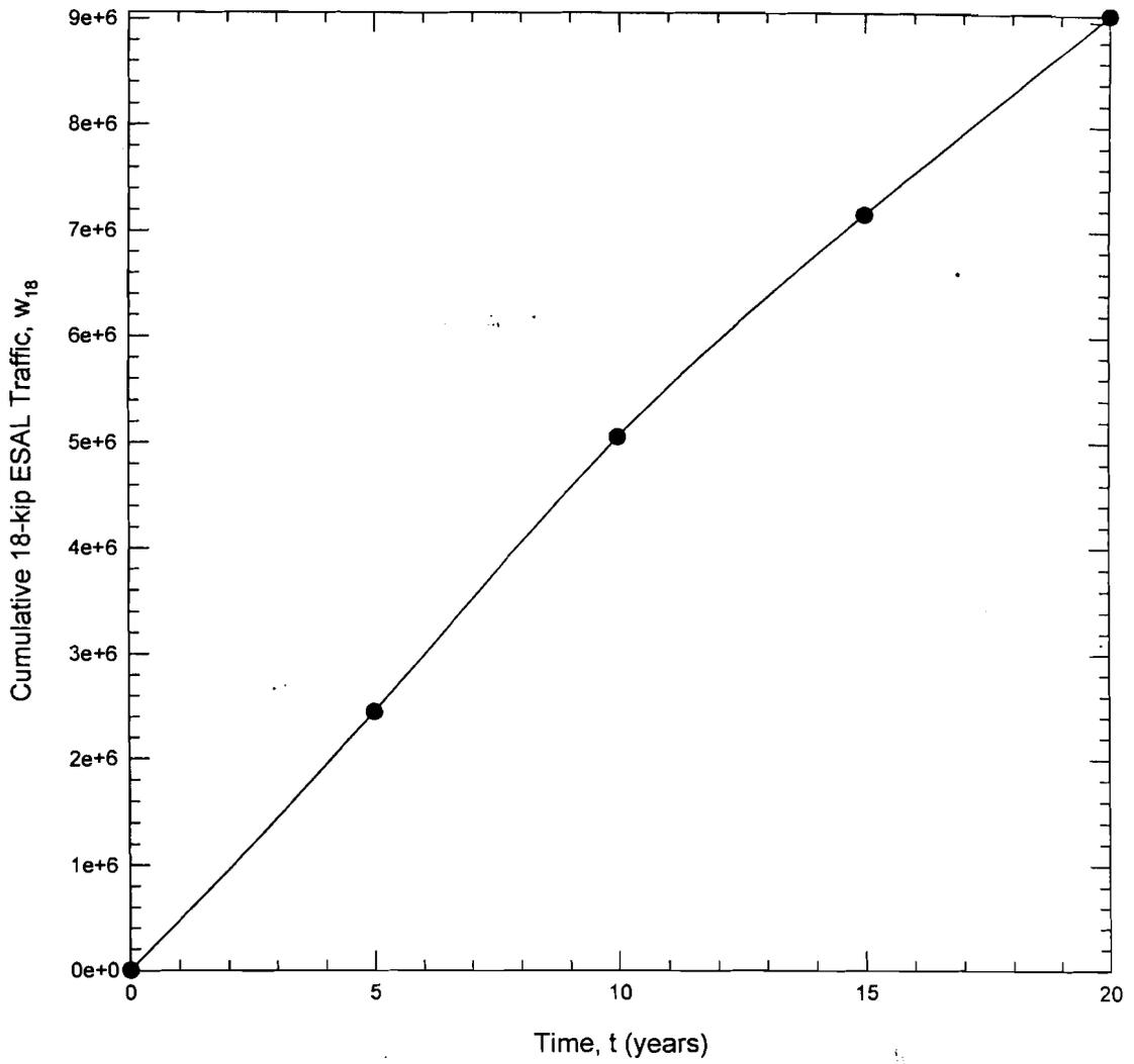
**Figure 4.45 Plot of Cumulative 18-kip ESAL Traffic Versus Time for the Pavement Structure of Rt. 2, RI**
