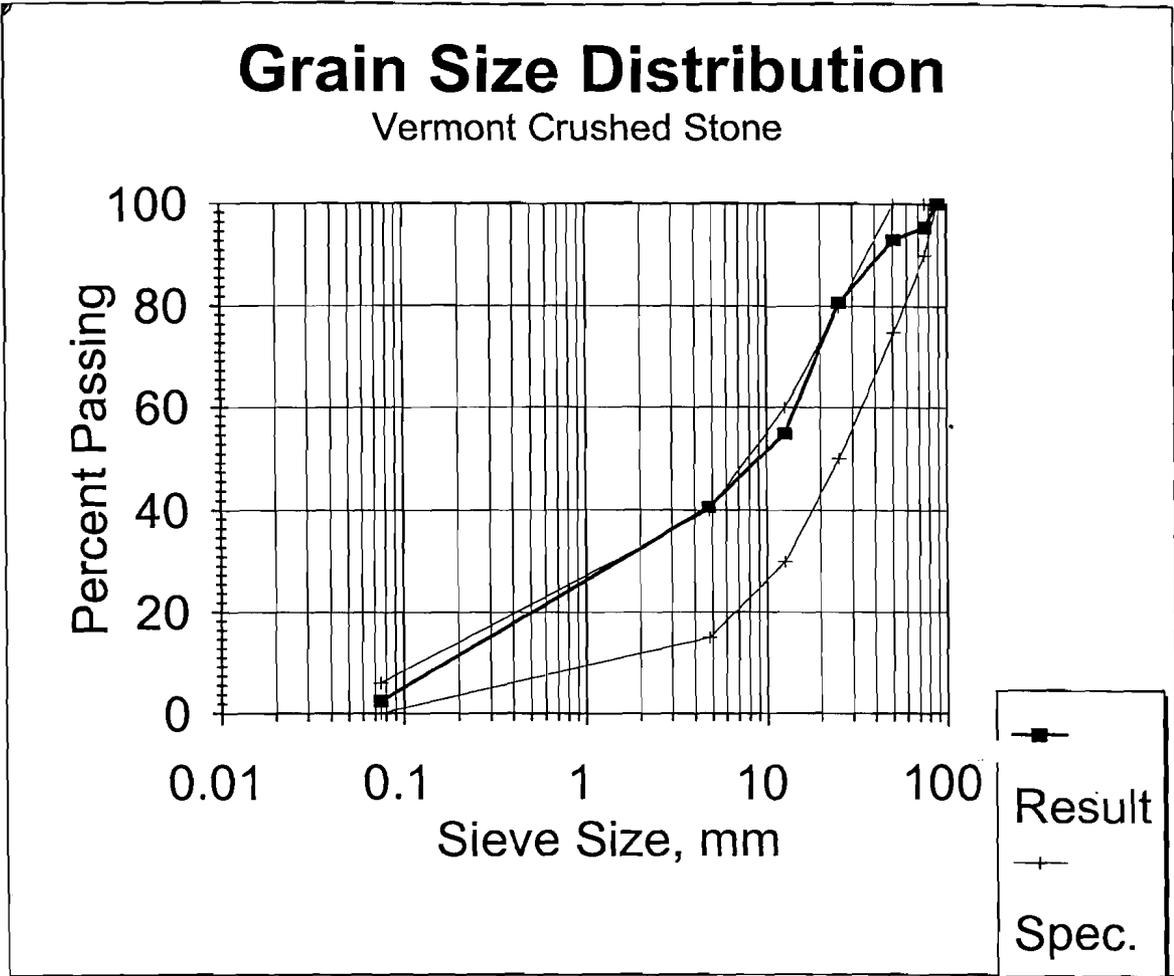
Figure 4.9 Vermont Crushed Stone Grain Size Distribution
