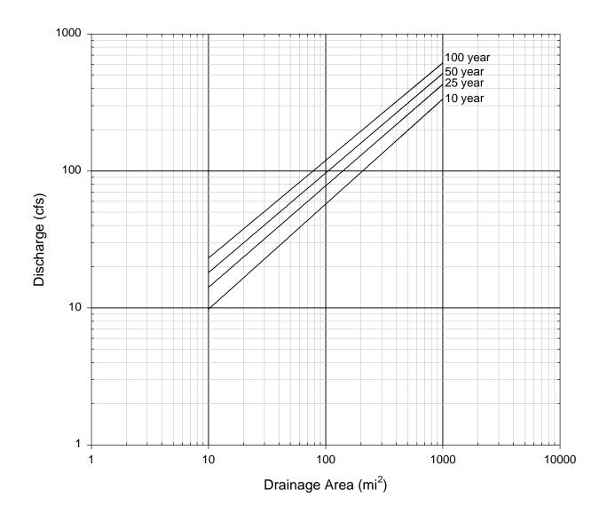
Figure 8. Discharge - drainage area functions for non-Berkshire gages in MA
