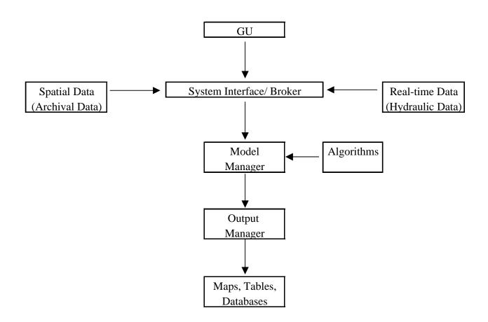
Figure 3. Proposed system architecture of spatial decision support system (SDSS) for scour monitoring
