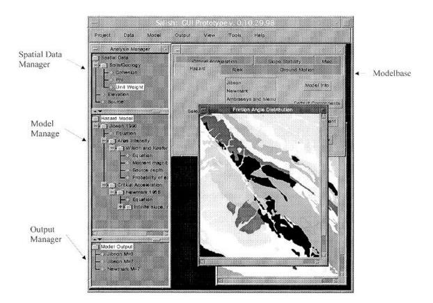
Figure 2. Conceptual prototype of spatial decision support system for seismic landslide analysis (from Miles and Ho, 1999a)
