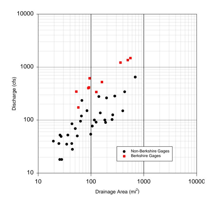
Figure B-3. Discharge vs. drainage area for active real-time stream gages in MA (50-year return period)
