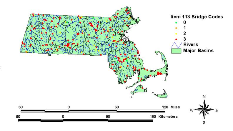
Figure 13. Multiple span, scour critical bridges in MA
