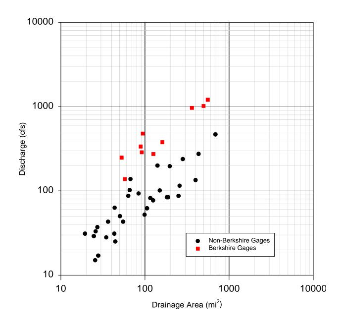
Figure B-1. Discharge vs. drainage area for active real-time stream gages in MA (25-year return period)
