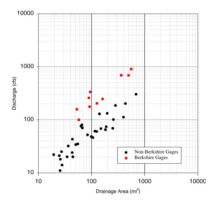
Figure 6. Discharge vs. drainage area for active real-time stream gages in MA (10-year return period)
