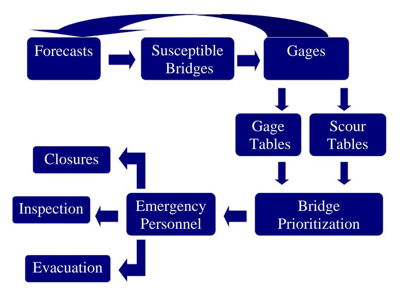
Figure 11. Flowchart of conceptual model for scour monitoring system
