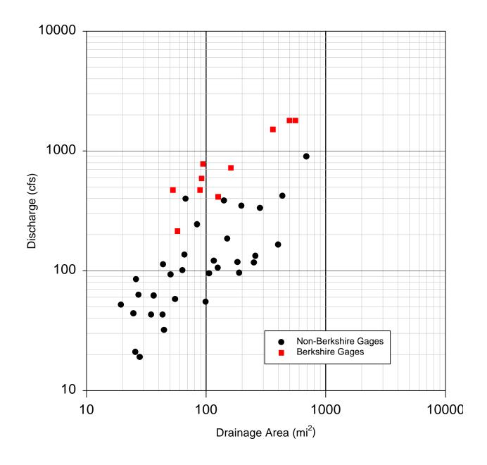
Figure B-5. Discharge vs. drainage area for active real-time stream gages in MA (100-year return period)
