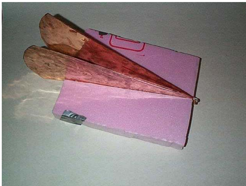
Figure 11.3 Photo of horn antenna before mounting and encasement.
