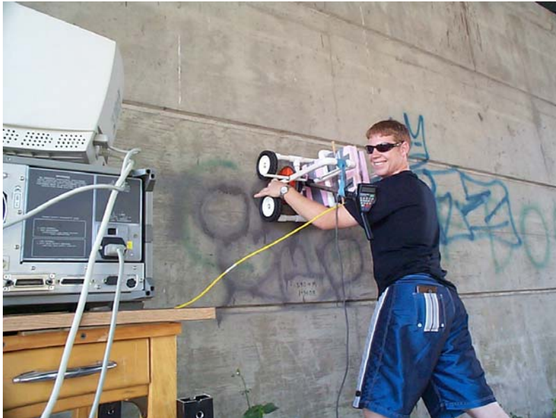
Figure 13.38. Test of handheld system on a retaining wall.
