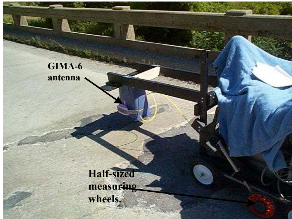
Figure 13.3 Second Bostwick Bridge, Shelburne, VT deck survey.
