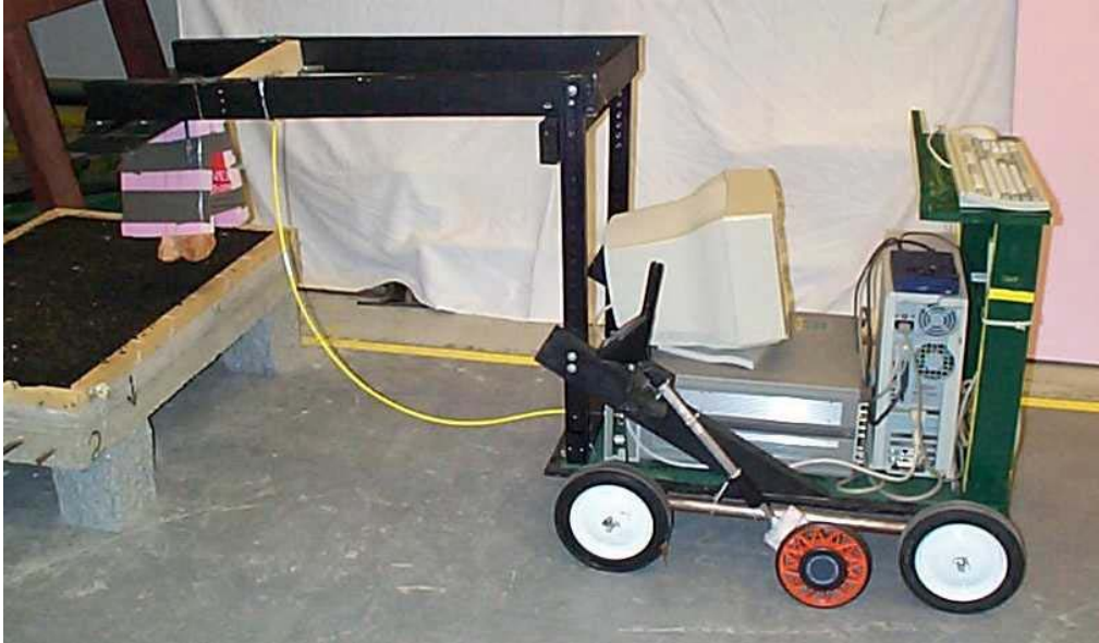
Figure 11.4 Picture of cart with GPR system.
