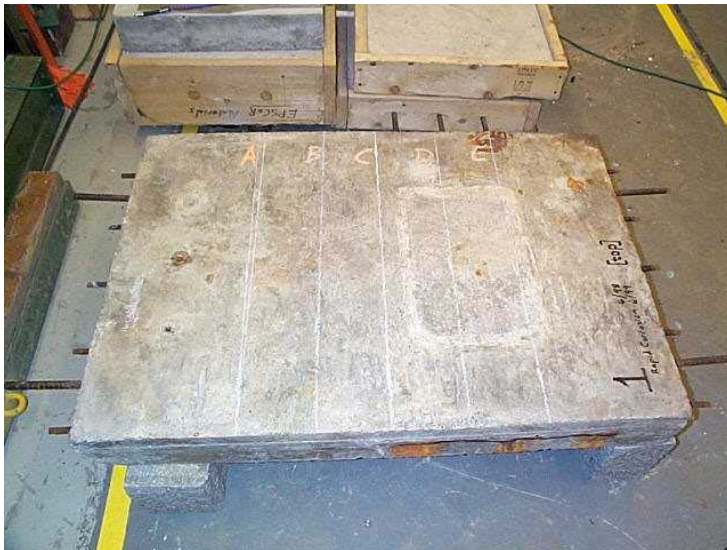
Figure 12.20 Top view of Slab 1 with scan lines drawn with chalk.
