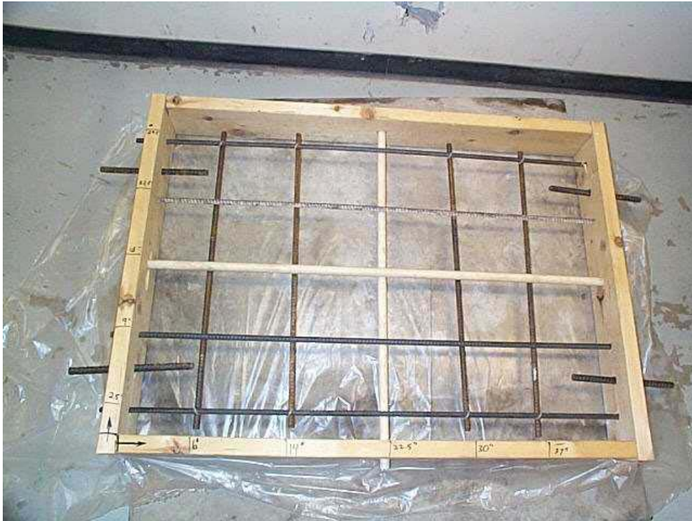
Figure 12.41 Picture of Slab 4 reinforcement including hollow tubes.
