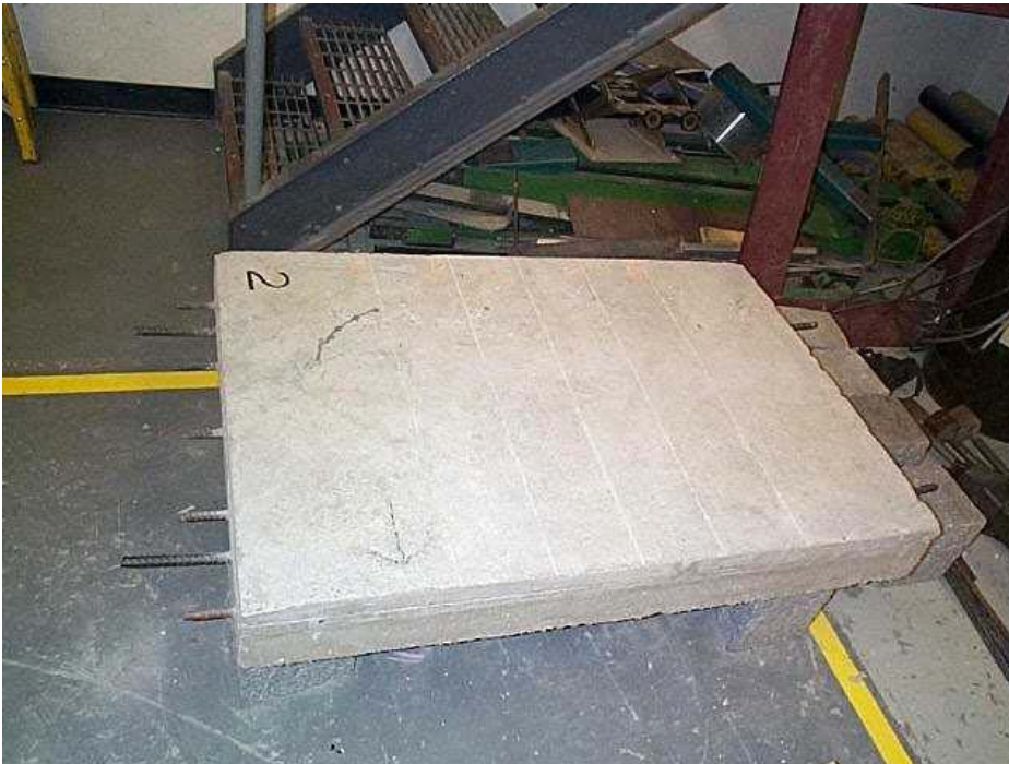
Figure 12.28 Picture of Slab 2 prior to the addition of a 38 mm thick layer of asphalt.
