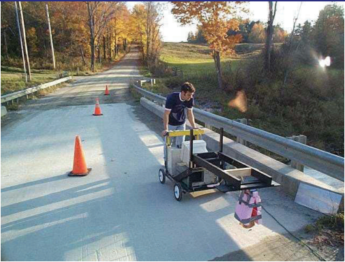
Examining the use of Ground Penetrating Radar for inspecting concrete bridge decks; University of Vermont - $224,901
