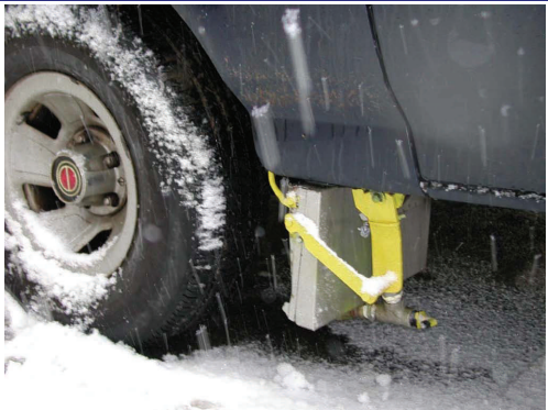
Development of a truck-mounted prototype for continuous measurement of roadway de-icing salt concentration; University of Connecticut - $187,336
