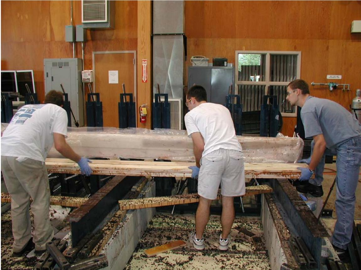
Figure 1: Guardrail Layup in Progress
