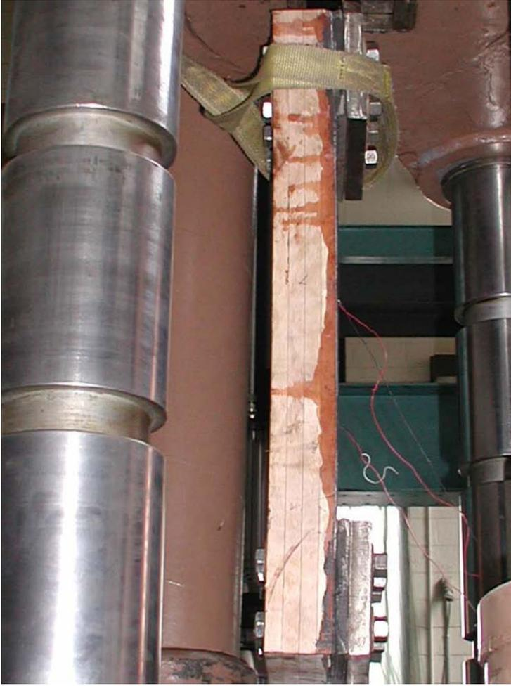
Figure 2: Rail Tension Splice Test
