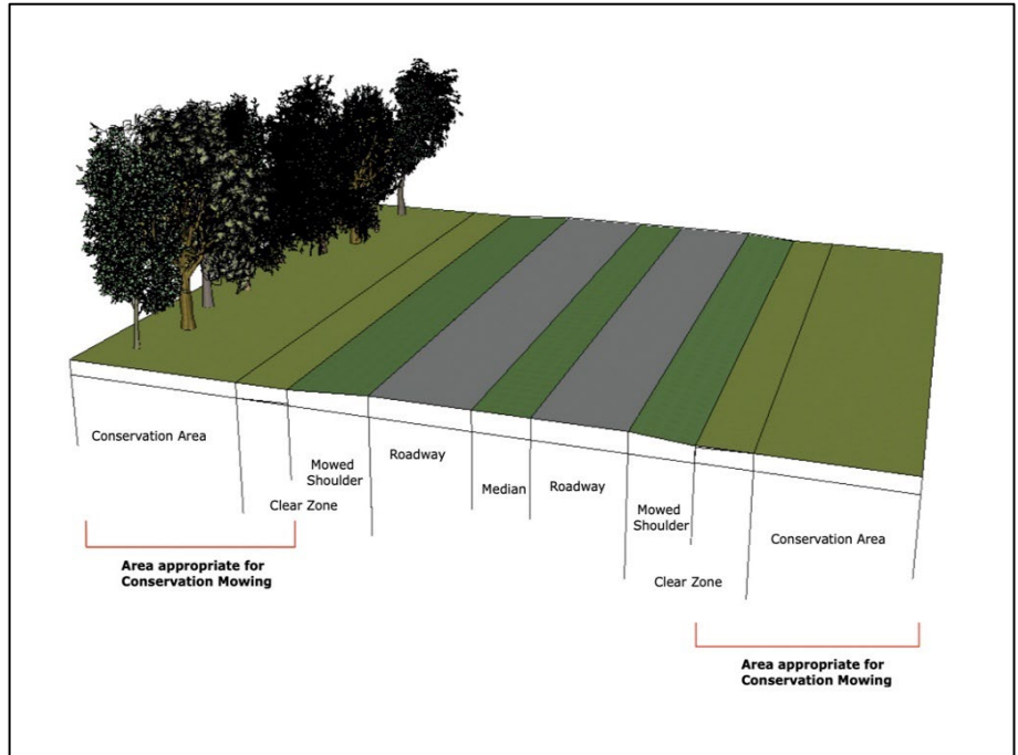
ROADWAY CROSS-SECTION – light green areas are appropriate for conservation mowing; dark green zones receive repeat mowing
