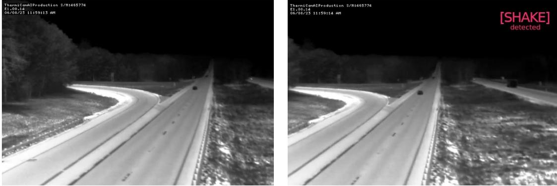
(a) Normal camera view. (b) Camera view change detected.
