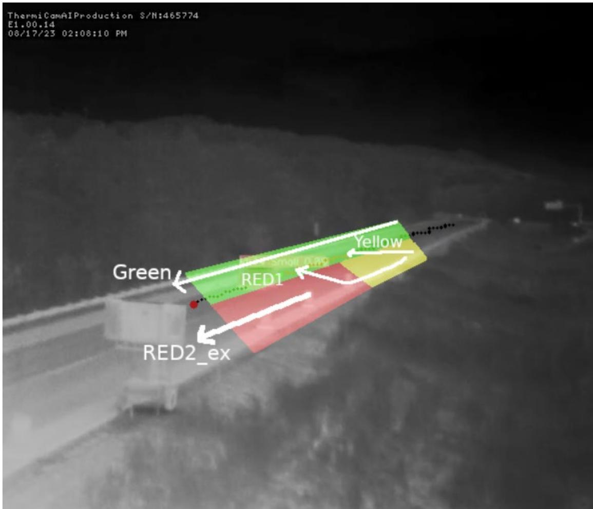
Figure 5-2. Work Zone Vehicle Trajectory Classification
