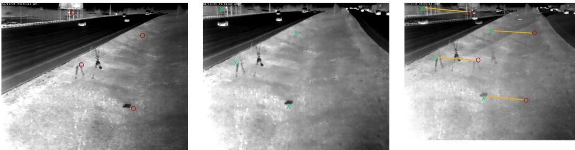
(a) Frame at time 9:01:41 AM: Points of interest (indicated by Os) identified in the initial frame. (b) Frame at time 9:01:42 AM: Points of interest (marked with Xs) detected in the subsequent frame. (c) Mapping Points of Interest: Yellow lines show the correspondence between Os and Xs.
