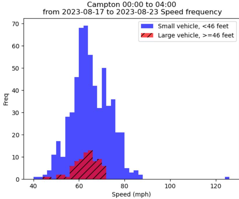
Figure 9-43. Average Speed vs. Frequency: Small vs. Large Vehicles at Campton 0 AM to 4 AM
