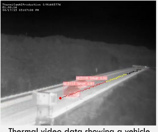
Thermal video data showing a vehicle merging at the last moment while approaching a work zone in Campton, NH
