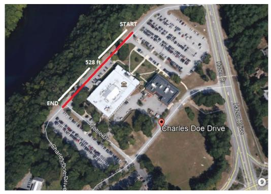
Figure 9. Photo. Medium-rough IRI site at Hazen Drive, Concord, NH, next to NHDOT office.
