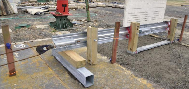
**Figure 291. Test set-up for measuring force-deflection response of a standard two-post guardrail end-terminal anchor.**
