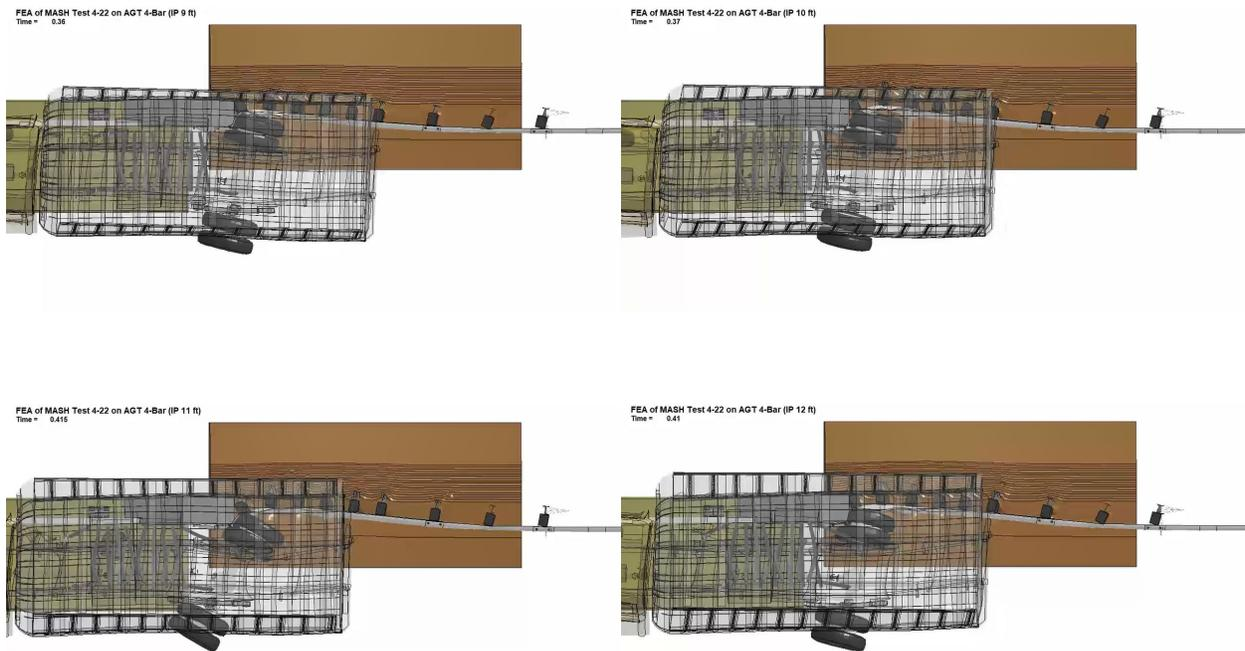
**Figure 342. Overhead images with transparent cargo-box showing the interaction of the rear wheel set and the concrete buttress.**
