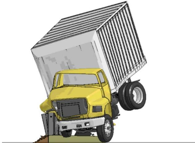
**Figure 359. Working width for Test 4-22 on MaineDOT transition.**
