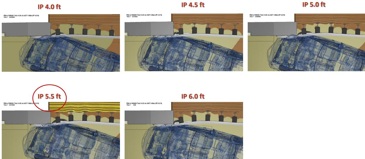
Figure 293. Results of the Test 4-20 simulations showing the deformation and position of the vehicle just before the tire impacted against the buttruss for each case.
