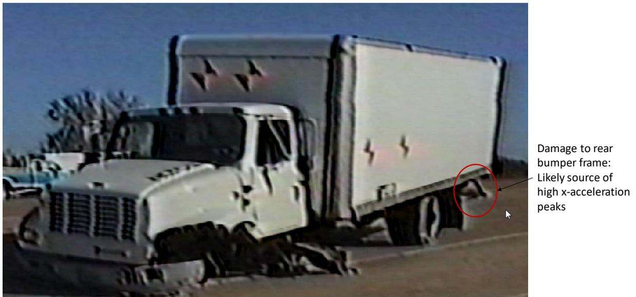
**Figure 79. Post-test photo of vehicle damages.**
