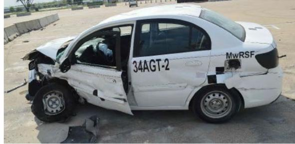
**Figure 316. Comparison of vehicle damage for FEA (MaineDOT transition) and full-scale test (MwRSF transition).**
