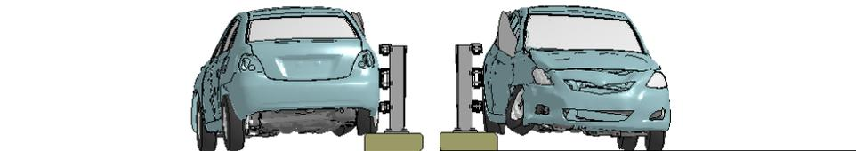
**Figure J-2. Sequential views from analysis of MASH Test 4-10 for NETC 3-Bar bridge rail from upstream and downstream viewpoints.**
