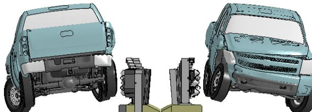
**Figure O-2. [Continued] Sequential views from analysis of MASH Test 4-21 for AGT 3-Bar transition from upstream and downstream viewpoints.**
