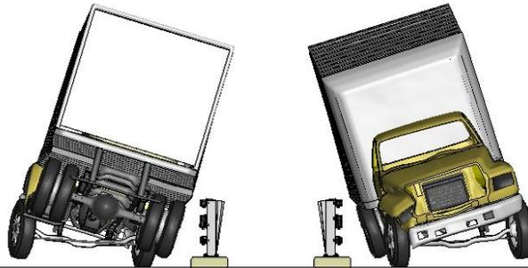
**Figure K-2. [Continued] Sequential views from analysis of MASH Test 4-12 for NETC 3-Bar bridge rail from upstream and downstream viewpoints – Case 1.**
