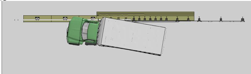
**Figure P-1. Sequential views from analysis of MASH Test 4-22 for AGT 3-Bar transition from an overhead viewpoint.**
