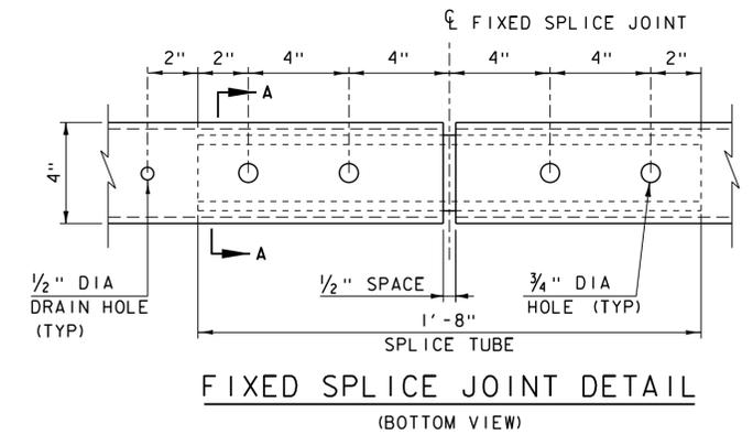
FIXED SPLICE JOINT DETAIL (BOTTOM VIEW)
