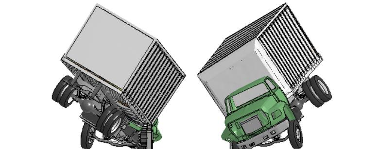
**Figure P-2. [Continued] Sequential views from analysis of MASH Test 4-22 for AGT 3-Bar transition from upstream and downstream viewpoints.**
