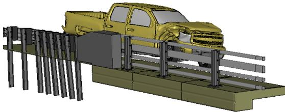
**Figure U-3. [Continued] Sequential views from analysis of MASH Test 4-21 for AGT 4-Bar bridge rail from an oblique viewpoint.**
