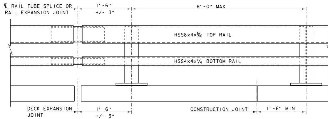
BRIDGE RAILING ELEVATION
