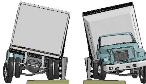
**Figure S-2. [Continued] Sequential views from analysis of MASH Test 4-12 for NETC 4-Bar bridge rail from upstream and downstream viewpoints.**
