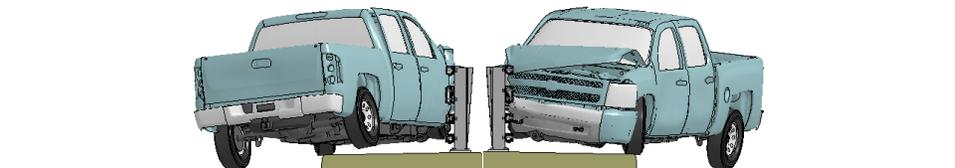
**Figure R-2. Sequential views from analysis of MASH Test 4-11 for NETC 4-Bar bridge rail from upstream and downstream viewpoints.**
