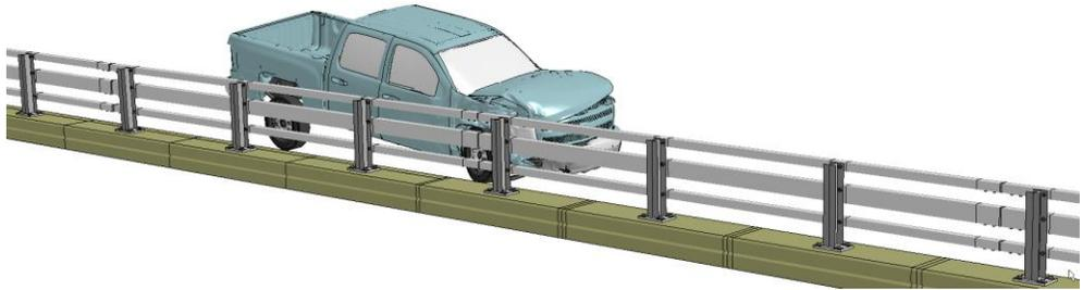
**Figure K-3. [Continued] Sequential views from analysis of MASH Test 4-11 for NETC 3-Bar bridge rail from from an oblique viewpoint.**
