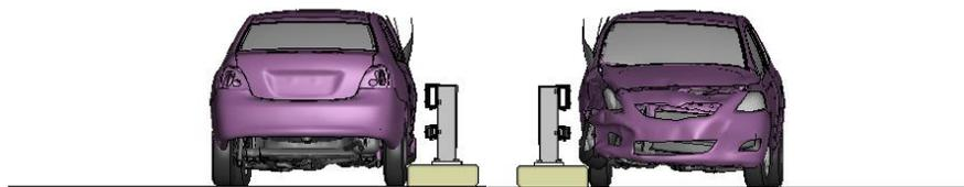
**Figure W-2. Sequential views from analysis of MASH Test 3-10 for NETC 2-Bar bridge rail from upstream and downstream viewpoints.**
