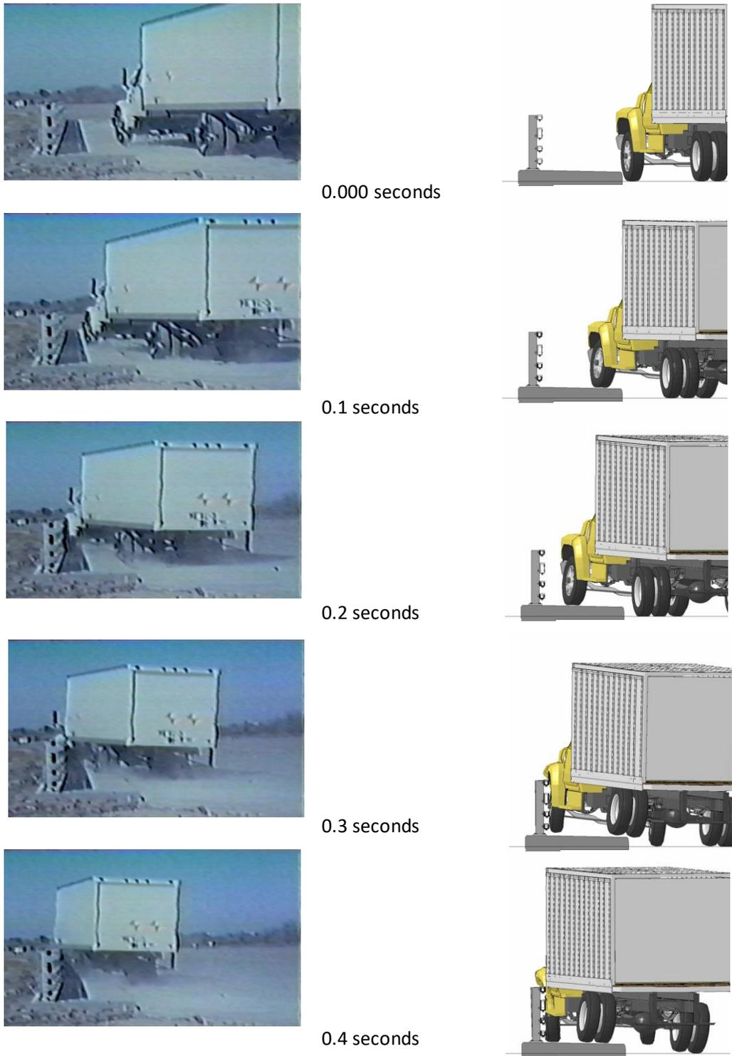
**Figure 1. Sequential views from FEA and Test NETC-3 from a upstream view point.**
