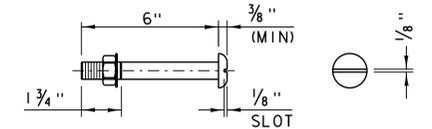
3/4" DIA A449 (TYPE 1) ROUND HEAD BOLT (WITH WASHER AND PREVAILING TORQUE TYPE LOCK NUT) (SEE NOTE #8) ONLY FULL DIAMETER BODY BOLTS WILL BE ALLOWED.
