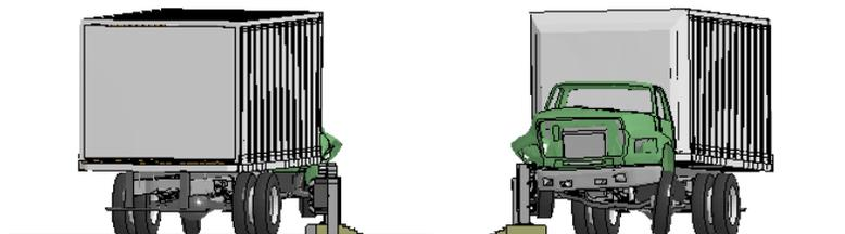
**Figure P-2. Sequential views from analysis of MASH Test 4-22 for AGT 3-Bar transition from upstream and downstream viewpoints.**
