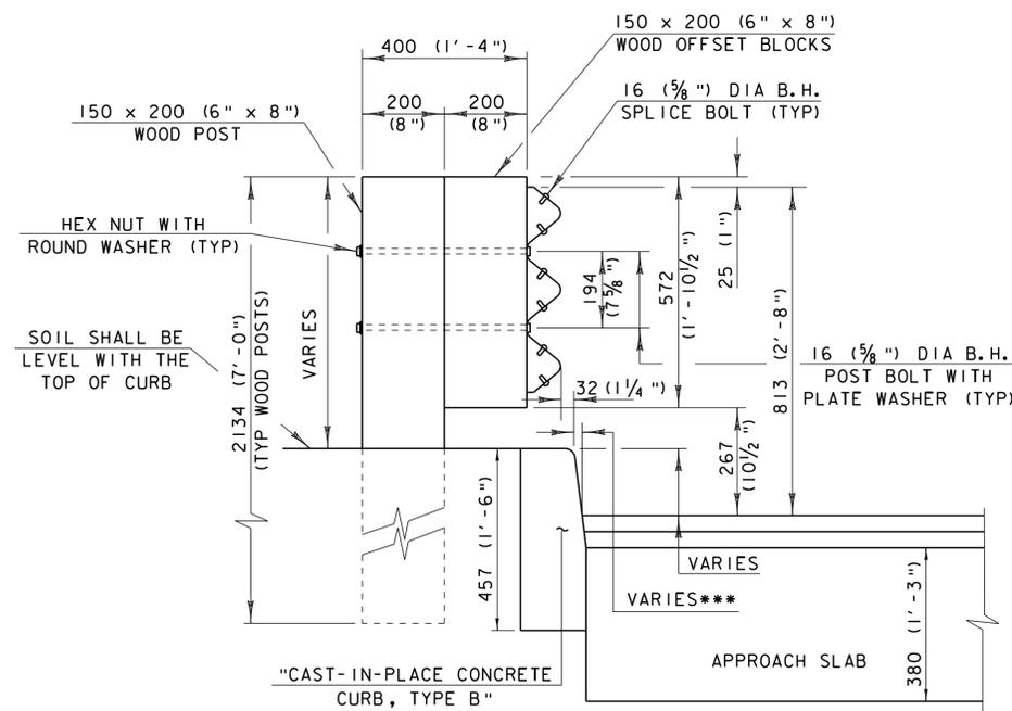
\*\*\* CHANGE SLOPE FROM 25 (1") IN 300 (12") AT BRIDGE TO 25 (1") IN 150 (6") PER STANDARD C-10 OVER A DISTANCE OF 3050 (10' - 0")
