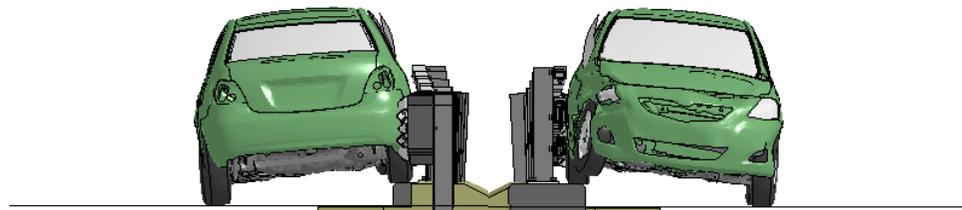
**Figure N-2. Sequential views from analysis of MASH Test 4-20 for AGT 3-Bar transition from upstream and downstream viewpoints.**
