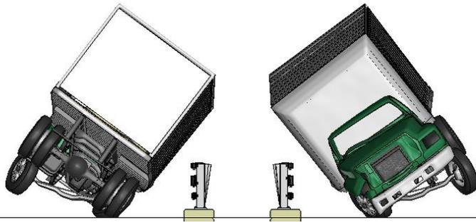
**Figure M-2. [Continued] Sequential views from analysis of MASH Test 4-12 for NETC 3-Bar bridge rail from upstream and downstream viewpoints – Case 2.**
