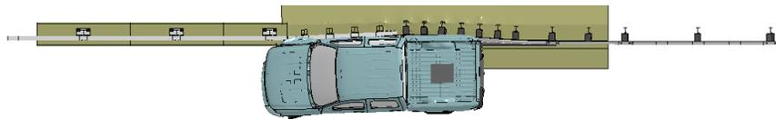
**Figure O-1. Sequential views from analysis of MASH Test 4-21 for AGT 3-Bar transition from an overhead viewpoint.**
