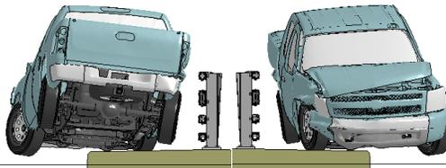
**Figure R-2. [Continued] Sequential views from analysis of MASH Test 4-11 for NETC 4-Bar bridge rail from upstream and downstream viewpoints.**
