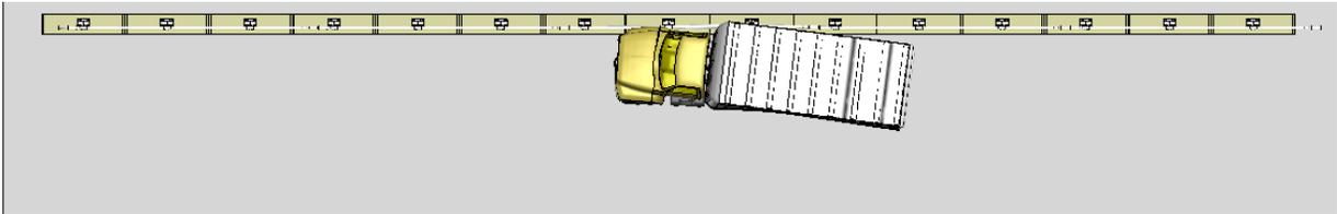
**Figure L-1. Sequential views from analysis of MASH Test 4-12 for NETC 3-Bar bridge rail from an overhead viewpoint – Case 1.**
