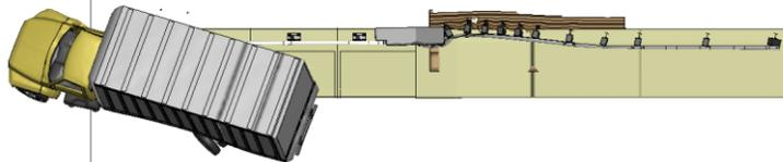
**Figure V-1. [Continued] Sequential views from analysis of MASH Test 4-22 for AGT 4-Bar bridge rail from an overhead viewpoint.**
