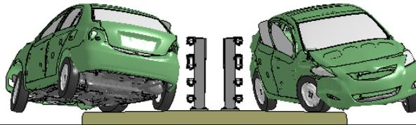
**Figure Q-2. [Continued] Sequential views from analysis of MASH Test 4-10 for NETC 4-Bar bridge rail from upstream and downstream viewpoints.**
