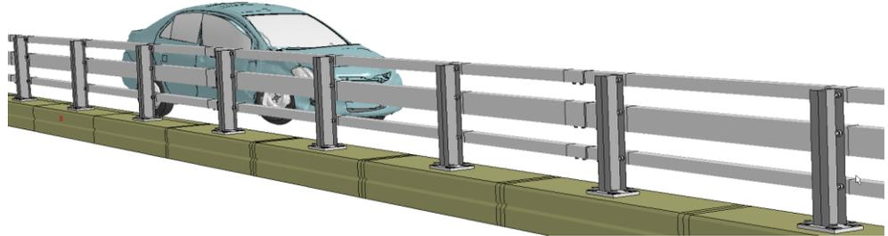
**Figure J-3. [Continued] Sequential views from analysis of MASH Test 4-10 for NETC 3-Bar bridge rail from from an oblique viewpoint.**
