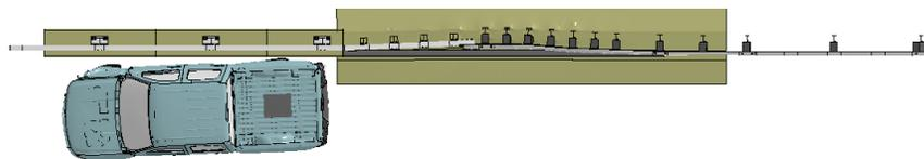
**Figure O-1. [Continued] Sequential views from analysis of MASH Test 4-21 for AGT 3-Bar transition from an overhead viewpoint.**
