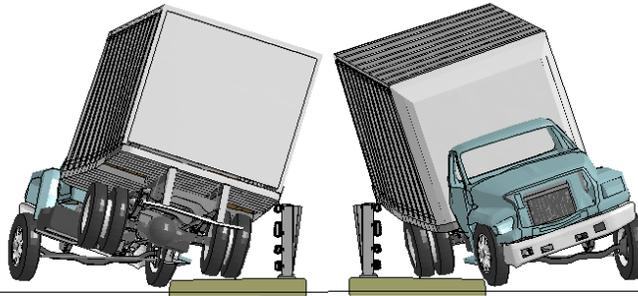
**Figure S-2. [Continued] Sequential views from analysis of MASH Test 4-12 for NETC 4-Bar bridge rail from upstream and downstream viewpoints.**
