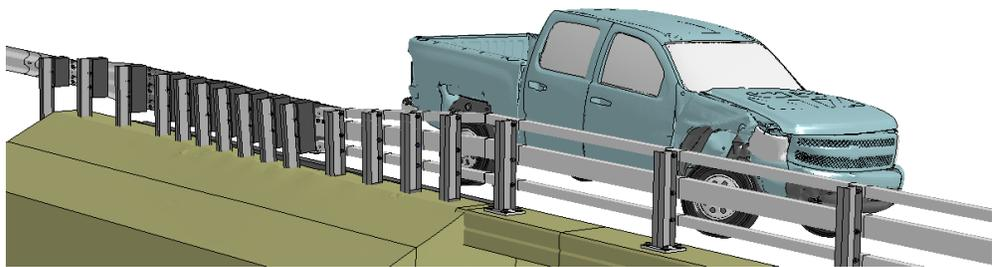
**Figure O-3. [Continued] Sequential views from analysis of MASH Test 4-21 for AGT 3-Bar transition from from an oblique viewpoint.**
