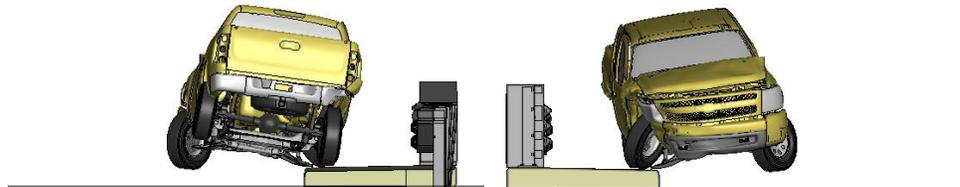
**Figure U-2. [Continued] Sequential views from analysis of MASH Test 4-21 for AGT 4-Bar bridge rail from upstream and downstream viewpoints.**
