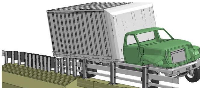
**Figure P-3. [Continued] Sequential views from analysis of MASH Test 4-22 for AGT 3-Bar transition from an oblique viewpoint.**
