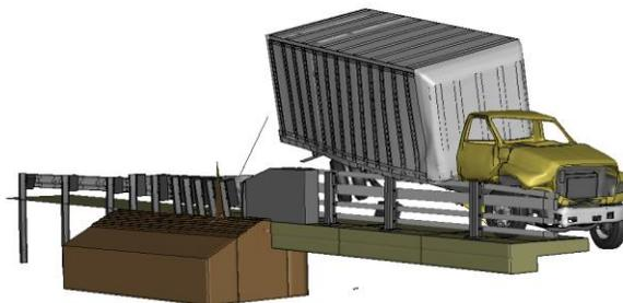
**Figure V-3. [Continued] Sequential views from analysis of MASH Test 4-22 for AGT 4-Bar bridge rail from an oblique viewpoint.**
