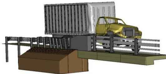
**Figure V-3. [Continued] Sequential views from analysis of MASH Test 4-22 for AGT 4-
