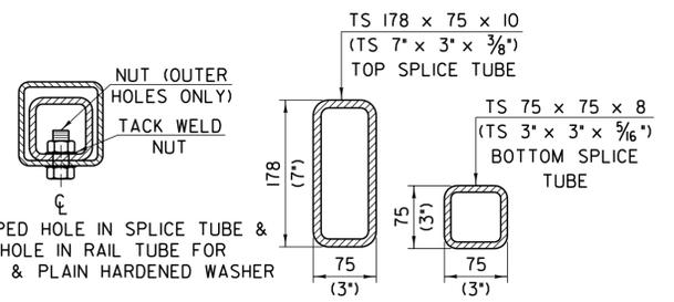
**RAIL TUBE SPLICE SECTION**
