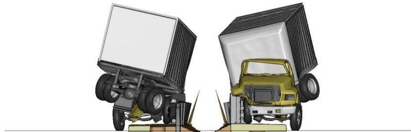
**Figure V-2. [Continued] Sequential views from analysis of MASH Test 4-22 for AGT 4-Bar bridge rail from upstream and downstream viewpoints.**
