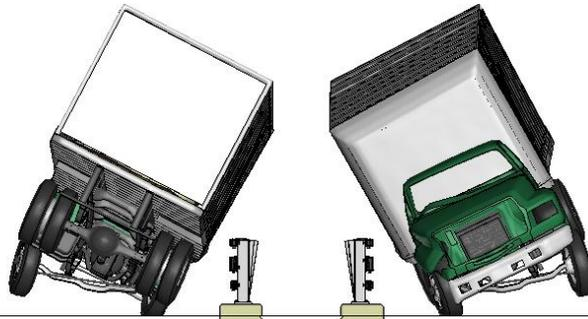
**Figure M-2. [Continued] Sequential views from analysis of MASH Test 4-12 for NETC 3-Bar bridge rail from upstream and downstream viewpoints – Case 2.**
