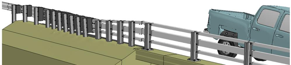
**Figure O-3. [Continued] Sequential views from analysis of MASH Test 4-21 for AGT 3-Bar transition from an oblique viewpoint.**
