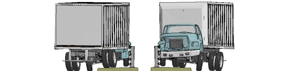
**Figure S-2. [Continued] Sequential views from analysis of MASH Test 4-12 for NETC 4-Bar bridge rail from upstream and downstream viewpoints.**
