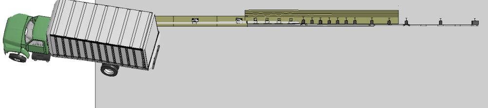
**Figure P-1. [Continued] Sequential views from analysis of MASH Test 4-22 for AGT 3-Bar transition from an overhead viewpoint.**
