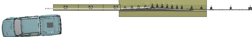
**Figure O-1. [Continued] Sequential views from analysis of MASH Test 4-21 for AGT 3-Bar transition from an overhead viewpoint.**
