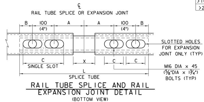
**RAIL TUBE SPLICE AND RAIL EXPANSION JOINT DETAIL (BOTTOM VIEW)**
