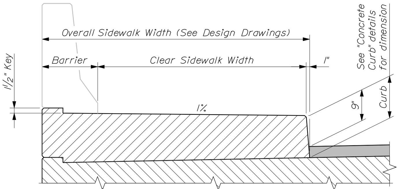
~ WITH PERMANENT CONCRETE BARRIER ~
