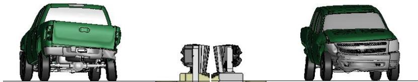
**Figure Z-2. [Continued] Sequential views from analysis of MASH Test 3-21 for AGT 2-Bar bridge rail from upstream and downstream viewpoints.**
