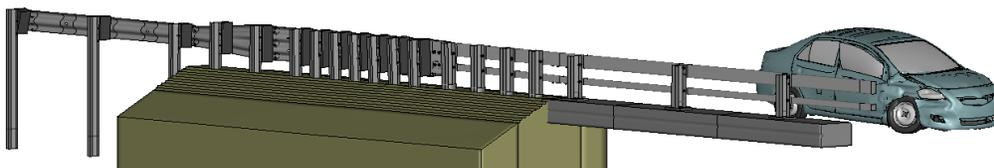
**Figure Y-3. [Continued] Sequential views from analysis of MASH Test 3-20 for AGT 2-Bar bridge rail from an oblique viewpoint.**
