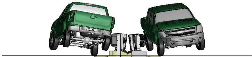
**Figure Z-2. [Continued] Sequential views from analysis of MASH Test 3-21 for AGT 2-Bar bridge rail from upstream and downstream viewpoints.**
