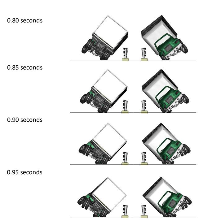
Figure M-2. [Continued] Sequential views from analysis of MASH Test 4-12 for NETC 3-Bar bridge rail from upstream and downstream viewpoints – Case 2.
