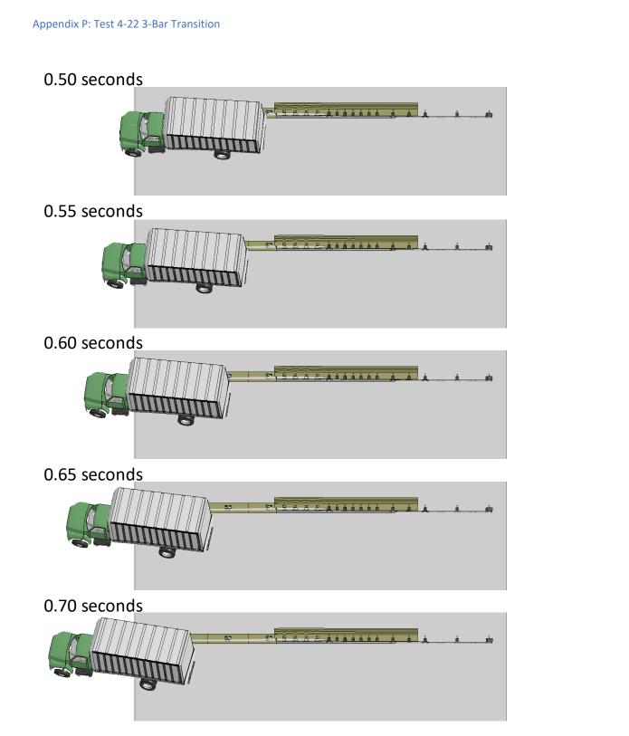
Figure P-1. [Continued] Sequential views from analysis of MASH Test 4-22 for AGT 3-Bar transition from an overhead viewpoint.
