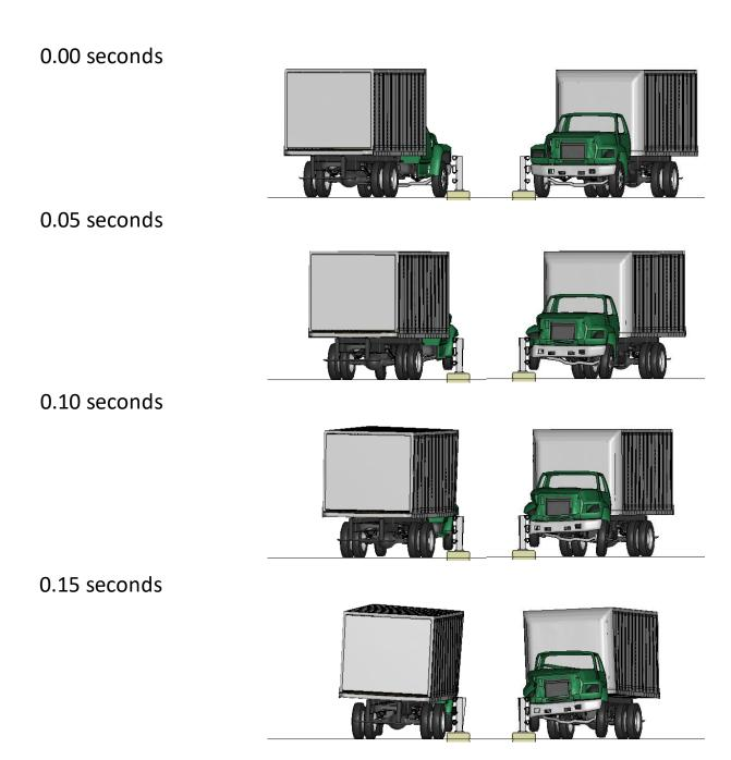
Figure M-2. Sequential views from analysis of MASH Test 4-12 for NETC 3-Bar bridge rail from upstream and downstream viewpoints – Case 2.
