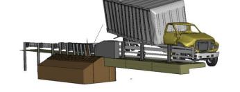
Figure V-3. [Continued] Sequential views from analysis of MASH Test 4-22 for AGT 4-Bar bridge rail from an oblique viewpoint.
