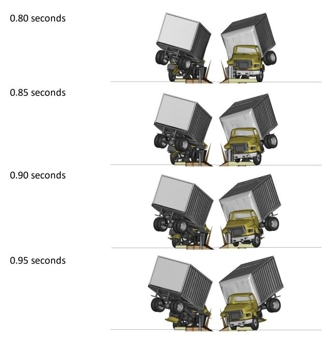
Figure V-2. [Continued] Sequential views from analysis of MASH Test 4-22 for AGT 4-Bar bridge rail from upstream and downstream viewpoints.
