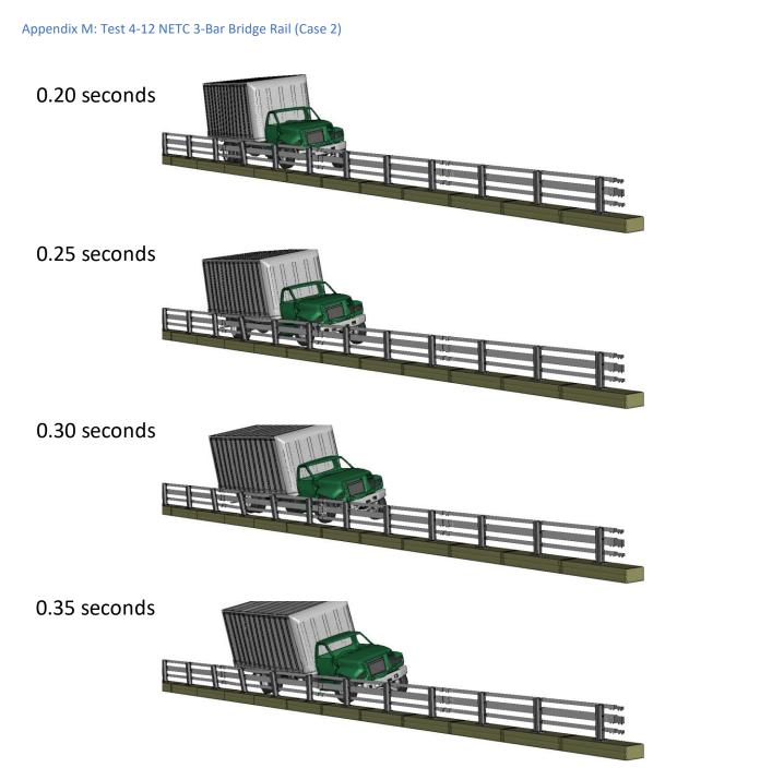
Figure M-3. [Continued] Sequential views from analysis of MASH Test 4-12 for NETC 3-Bar bridge rail from an oblique viewpoint – Case 2.
