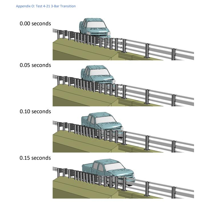
Figure O-3. Sequential views from analysis of MASH Test 4-21 for AGT 3-Bar transition from an oblique viewpoint.
