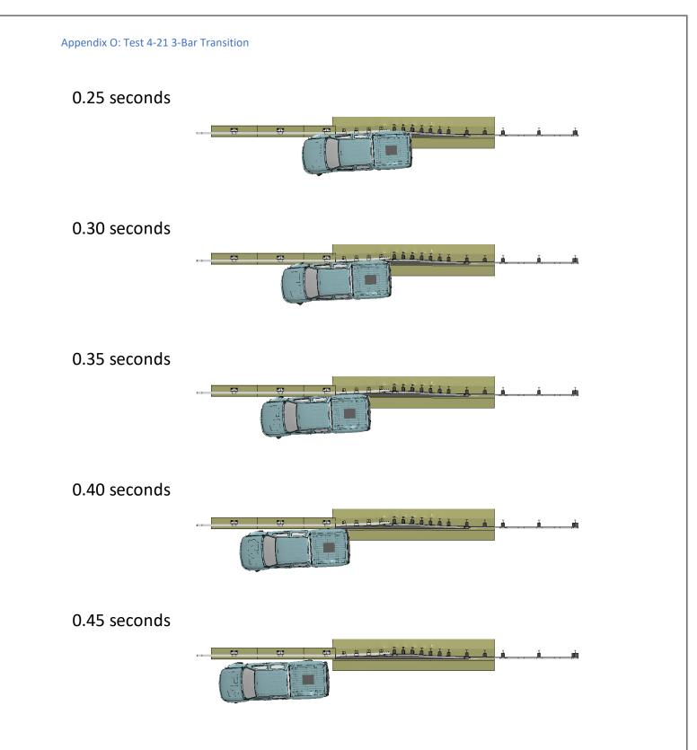
Figure O-1. [Continued] Sequential views from analysis of MASH Test 4-21 for AGT 3-Bar transition from an overhead viewpoint.
