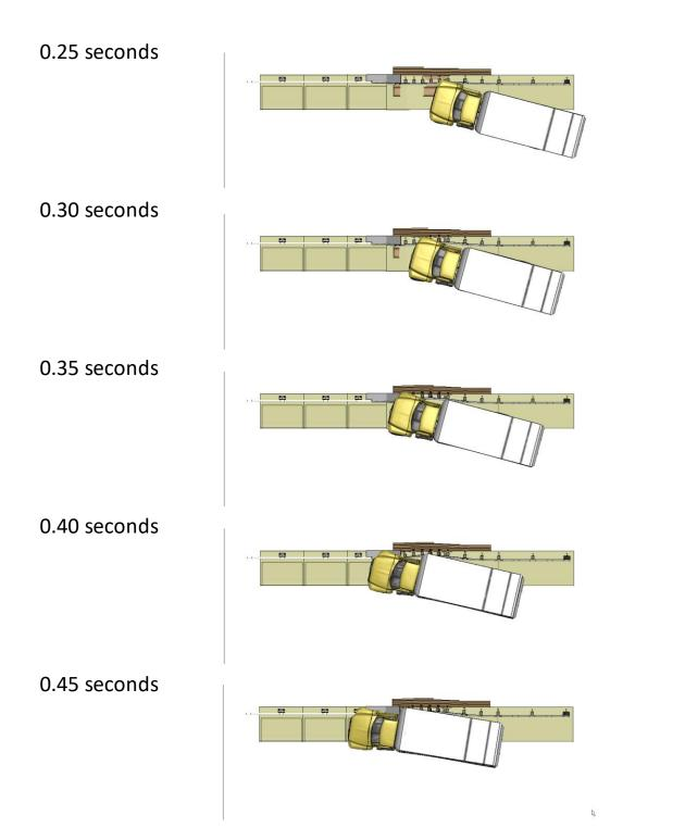
Figure V-1. [Continued] Sequential views from analysis of MASH Test 4-22 for AGT 4-Bar bridge rail from an overhead viewpoint.
