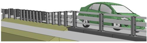
Figure N-3. [Continued] Sequential views from analysis of MASH Test 4-20 for AGT 3-Bar transition from an oblique viewpoint.
