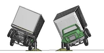
Figure P-2. [Continued] Sequential views from analysis of MASH Test 4-22 for AGT 3-Bar transition from upstream and downstream viewpoints.
