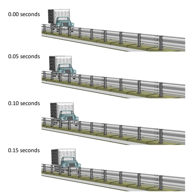
Figure S-3. Sequential views from analysis of MASH Test 4-12 for NETC 4-Bar bridge rail from an oblique viewpoint.
