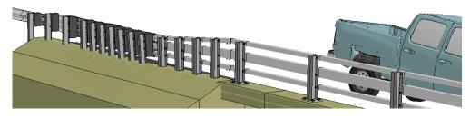
Figure O-3. [Continued] Sequential views from analysis of MASH Test 4-21 for AGT 3-Bar transition from an oblique viewpoint.
