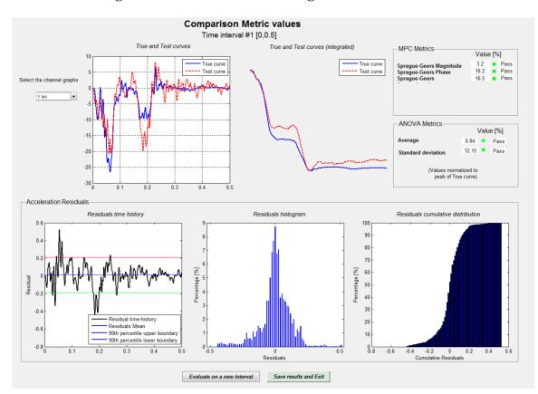
Figure 2c: RSVVP Results – Lateral Acceleration
