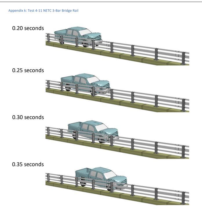
Figure K-3. [Continued] Sequential views from analysis of MASH Test 4-11 for NETC 3-Bar bridge rail from from an oblique viewpoint.
