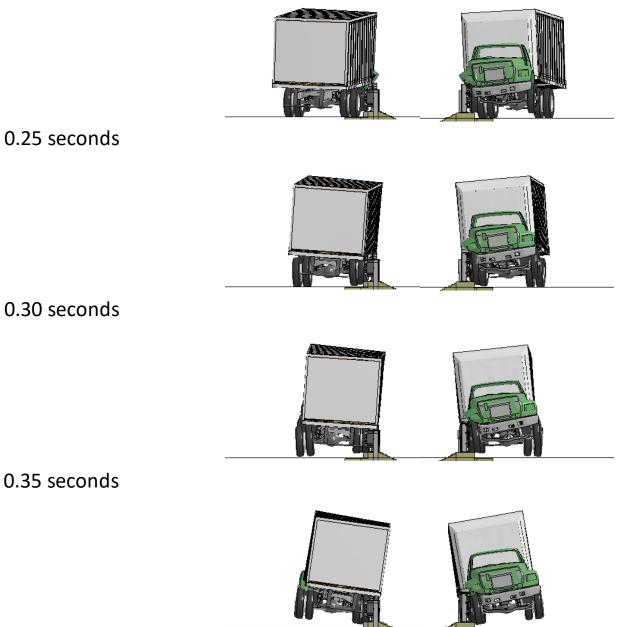
Figure P-2. [Continued] Sequential views from analysis of MASH Test 4-22 for AGT 3-Bar transition from upstream and downstream viewpoints.
