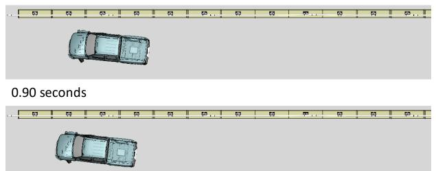
Figure X-1. [Continued] Sequential views from analysis of MASH Test 3-11 for NETC 2-Bar bridge rail from an overhead viewpoint.
