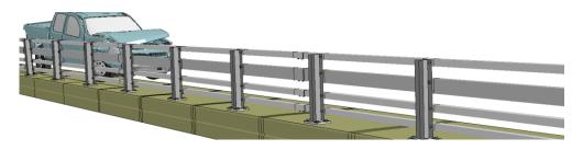
Figure R-3. [Continued] Sequential views from analysis of MASH Test 4-11 for NETC 4-Bar bridge rail from from an oblique viewpoint.
