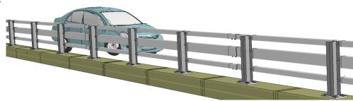
Figure J-3. [Continued] Sequential views from analysis of MASH Test 4-10 for NETC 3-Bar bridge rail from from an oblique viewpoint.
