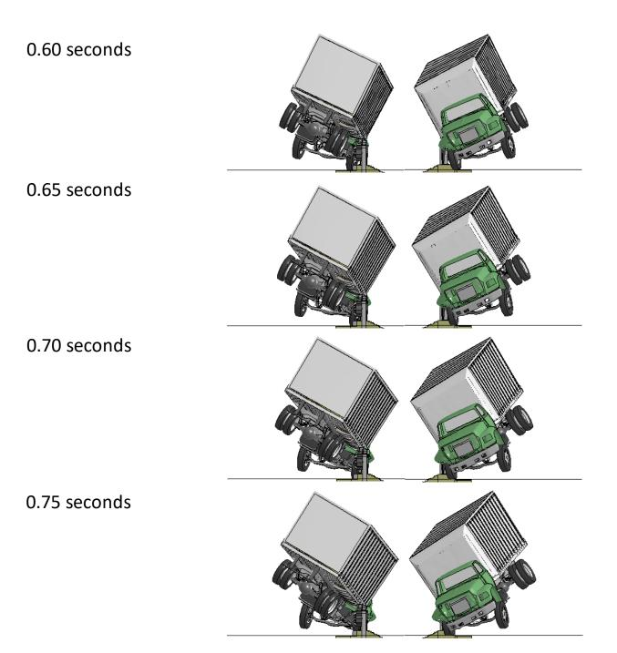
Figure P-2. [Continued] Sequential views from analysis of MASH Test 4-22 for AGT 3-Bar transition from upstream and downstream viewpoints.
