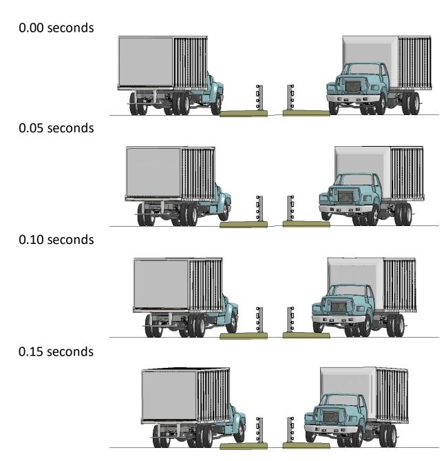
Figure S-2. Sequential views from analysis of MASH Test 4-12 for NETC 4-Bar bridge rail from upstream and downstream viewpoints.
