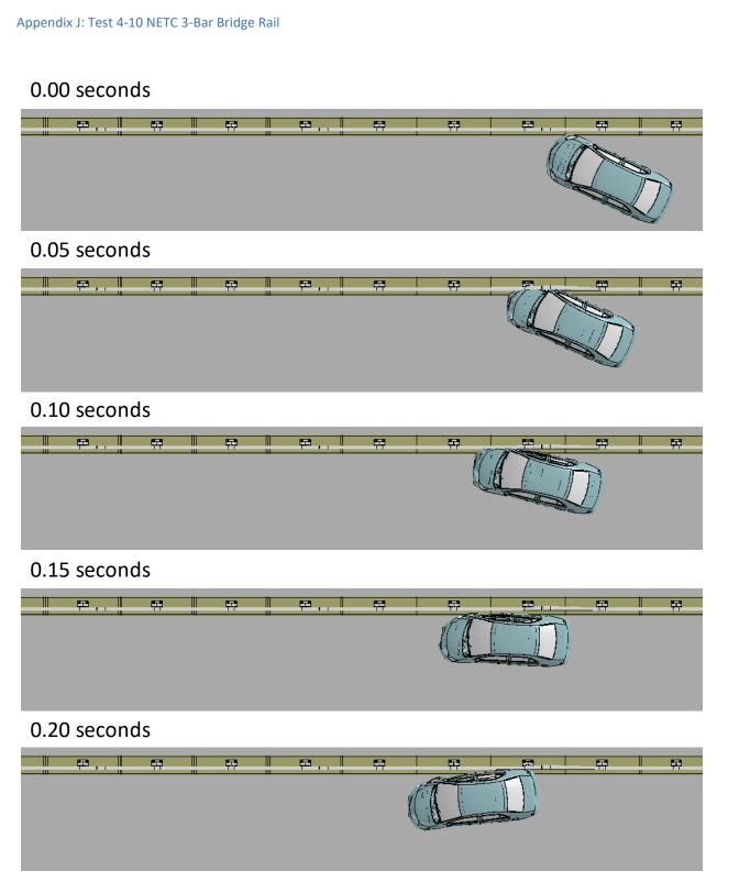
Figure J-1. Sequential views from analysis of MASH Test 4-10 for NETC 3-Bar bridge rail from an overhead viewpoint.
