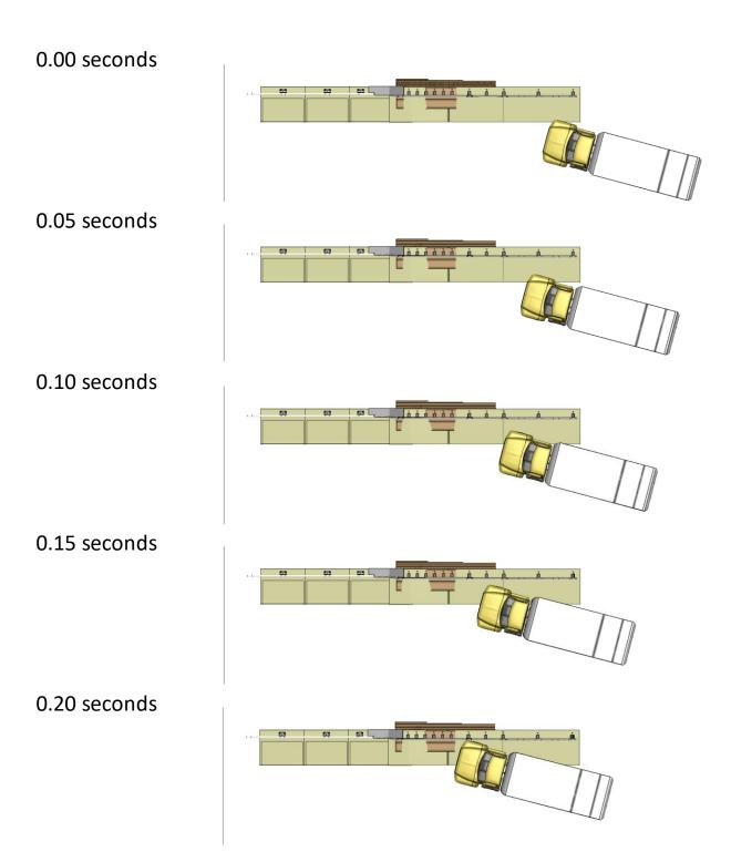
Figure V-1. Sequential views from analysis of MASH Test 4-22 for AGT 4-Bar bridge rail from an overhead viewpoint.
