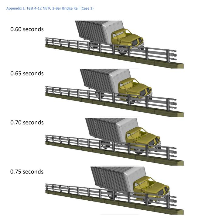
Figure K-3. [Continued] Sequential views from analysis of MASH Test 4-12 for NETC 3-Bar bridge rail from an oblique viewpoint – Case 1. Sequential Views for Test 4-12 on
