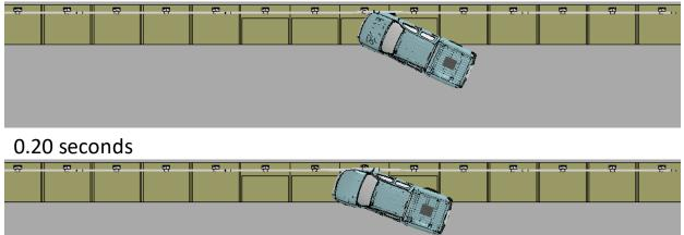
Figure R-1. Sequential views from analysis of MASH Test 4-11 for NETC 4-Bar bridge rail from an overhead viewpoint.
