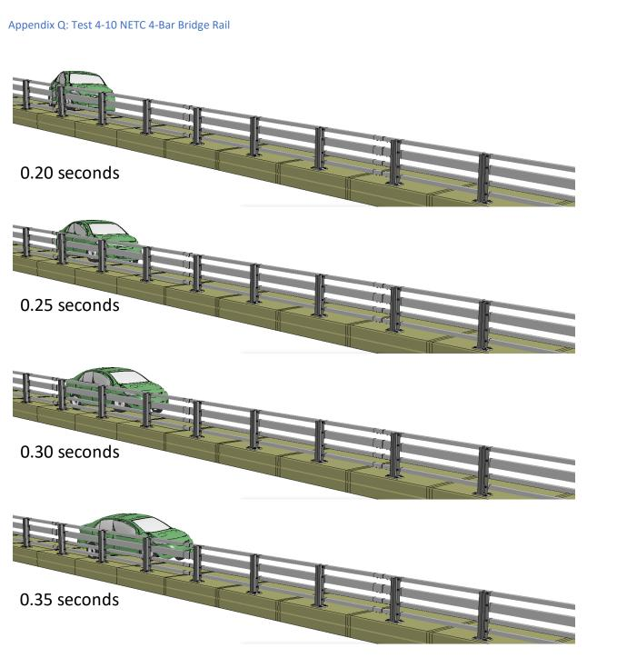
Figure Q-3. [Continued] Sequential views from analysis of MASH Test 4-10 for NETC 4-Bar bridge rail from from an oblique viewpoint.
