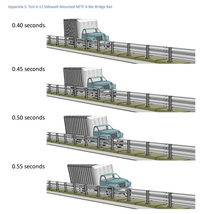
Figure S-3. [Continued] Sequential views from analysis of MASH Test 4-12 for NETC 4-Bar bridge rail from an oblique viewpoint.
