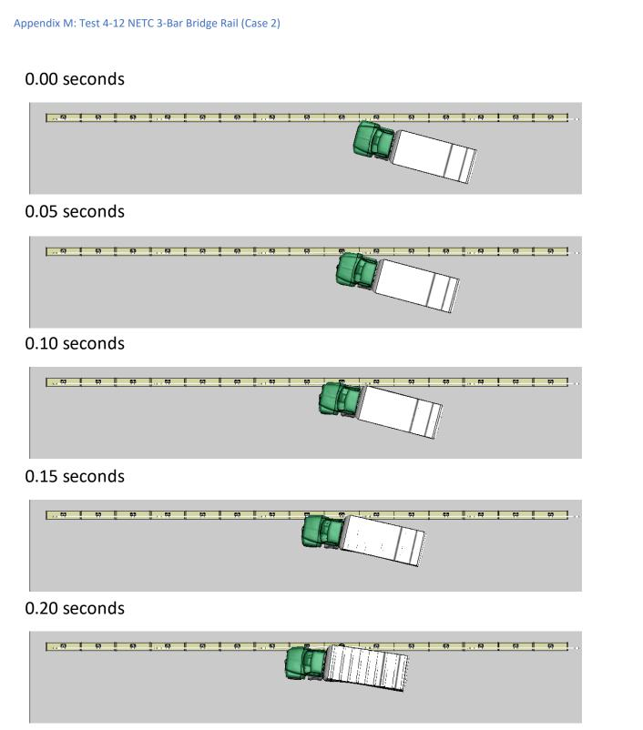
Figure M-1. Sequential views from analysis of MASH Test 4-12 for NETC 3-Bar bridge rail from an overhead viewpoint – Case 2.
