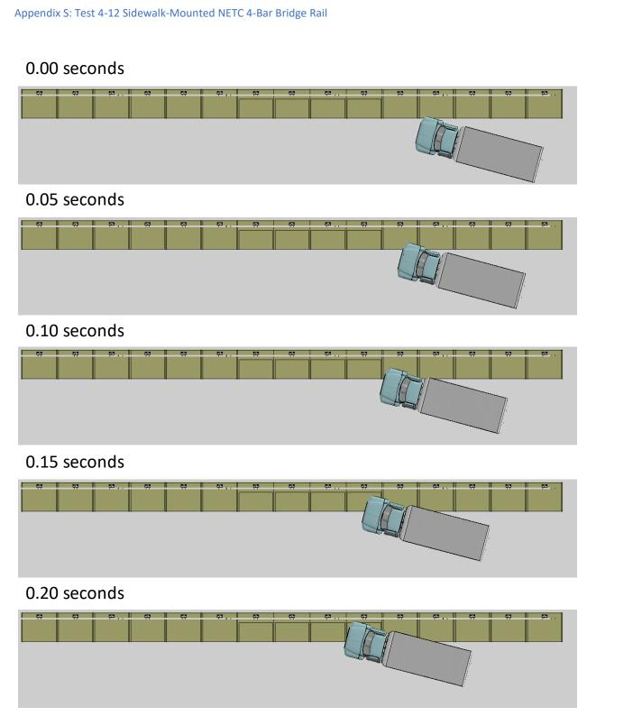
Figure S-1. Sequential views from analysis of MASH Test 4-12 for NETC 4-Bar bridge rail from an overhead viewpoint.
