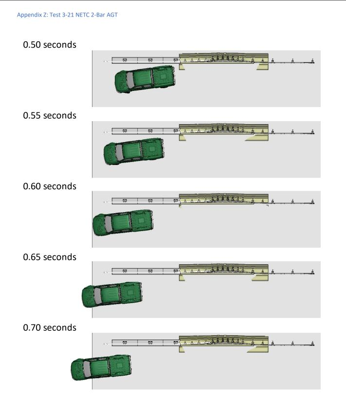
Figure Z-1. [Continued] Sequential views from analysis of MASH Test 3-21 for AGT 2-Bar bridge rail from an overhead viewpoint.
