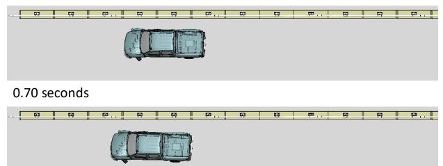
Figure X-1. [Continued] Sequential views from analysis of MASH Test 3-11 for NETC 2-Bar bridge rail from an overhead viewpoint.
