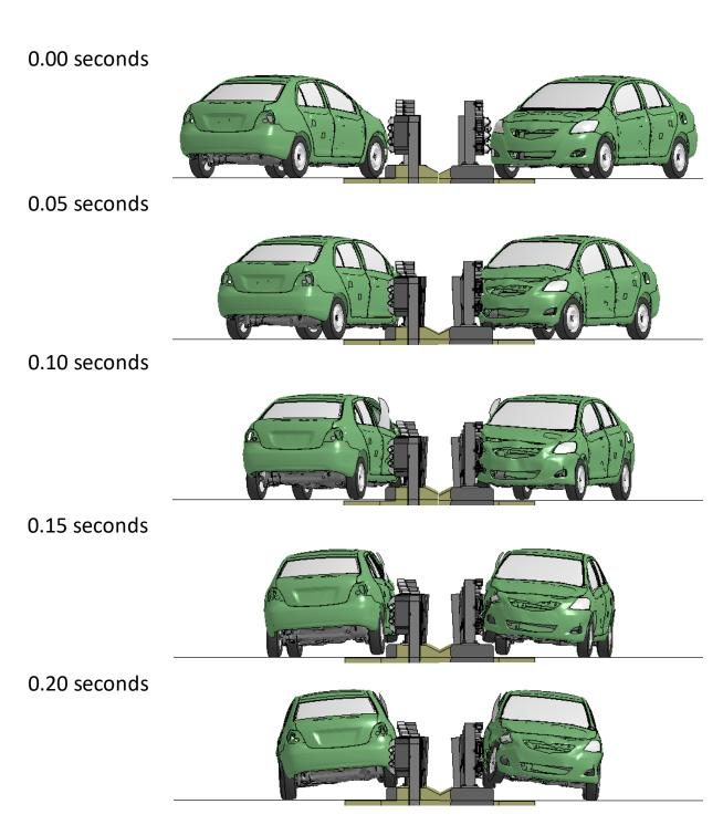
Figure N-2. Sequential views from analysis of MASH Test 4-20 for AGT 3-Bar transition from upstream and downstream viewpoints.
