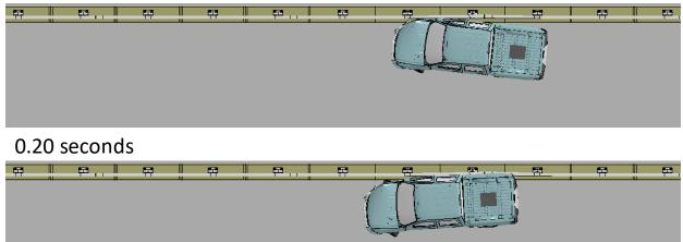
Figure K-1. Sequential views from analysis of MASH Test 4-11 for NETC 3-Bar bridge rail from an overhead viewpoint.
