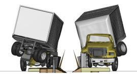
Figure V-2. [Continued] Sequential views from analysis of MASH Test 4-22 for AGT 4-Bar bridge rail from upstream and downstream viewpoints.
