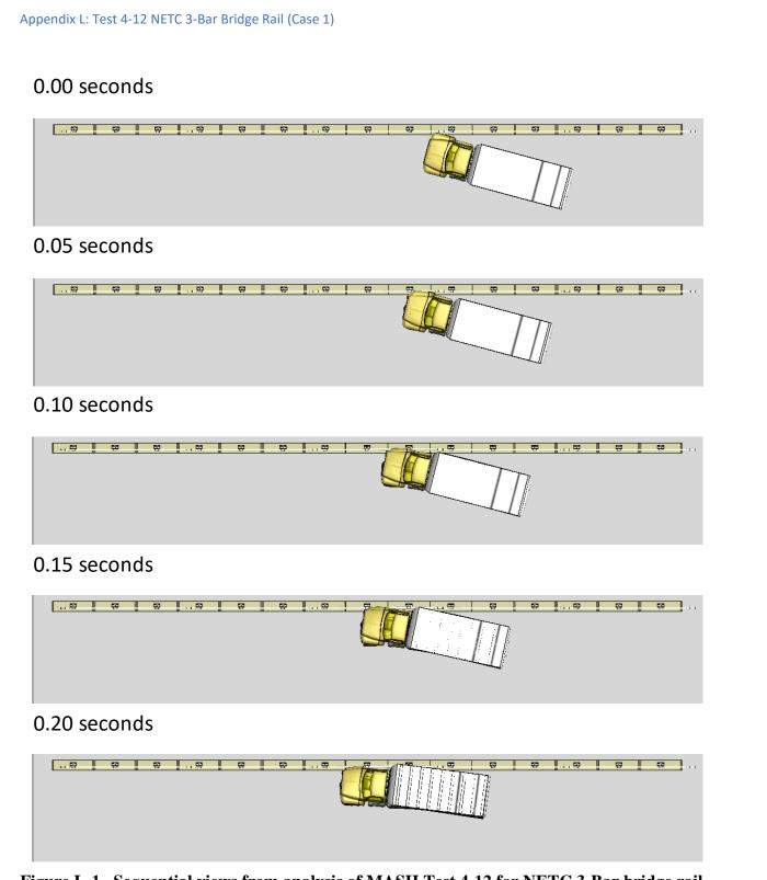
Figure L-1. Sequential views from analysis of MASH Test 4-12 for NETC 3-Bar bridge rail from an overhead viewpoint – Case 1.
