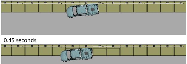
Figure R-1. [Continued] Sequential views from analysis of MASH Test 4-11 for NETC 4-Bar bridge rail from an overhead viewpoint.
