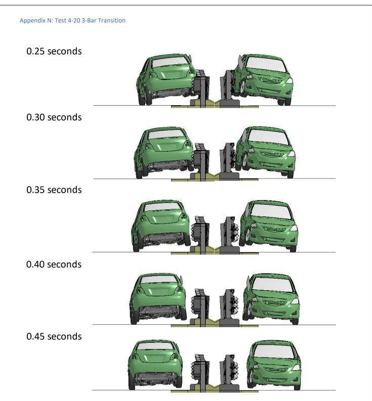
Figure N-2. [Continued] Sequential views from analysis of MASH Test 4-20 for AGT 3-Bar transition from upstream and downstream viewpoints.
