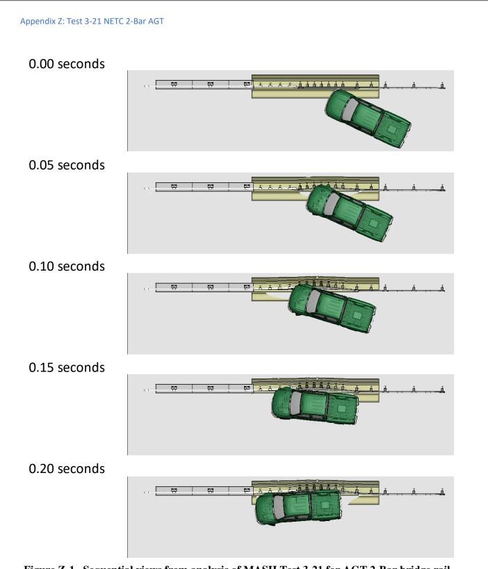
Figure Z-1. Sequential views from analysis of MASH Test 3-21 for AGT 2-Bar bridge rail from an overhead viewpoint.
