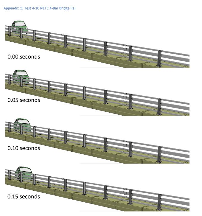
Figure Q-3. Sequential views from analysis of MASH Test 4-10 for NETC 4-Bar bridge rail from an oblique viewpoint.
