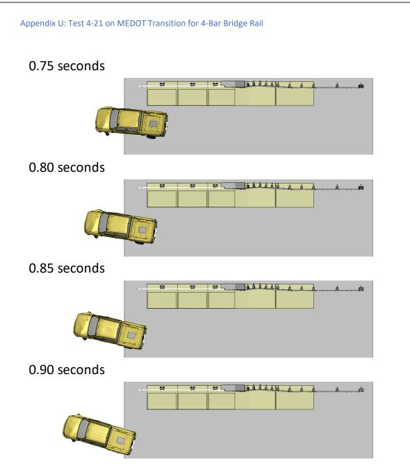
Figure U-1. [Continued] Sequential views from analysis of MASH Test 4-21 for AGT 4-Bar bridge rail from an overhead viewpoint.
