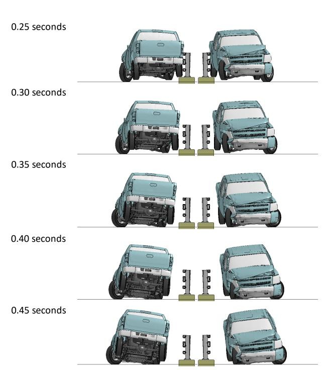
Figure K-2. [Continued] Sequential views from analysis of MASH Test 4-11 for NETC 3-Bar bridge rail from upstream and downstream viewpoints.
