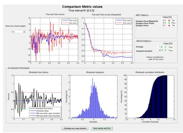
Figure 2e: RSVVP Results – Roll Angle
