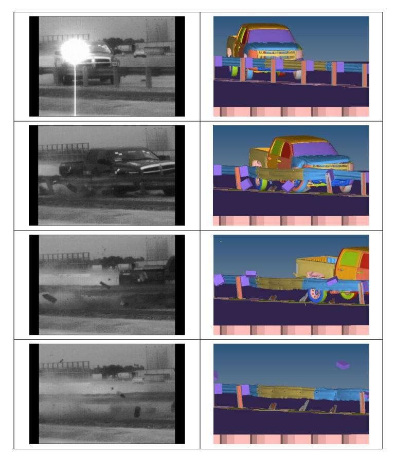
Figure 6b: Sequential Comparisons – Rear View
