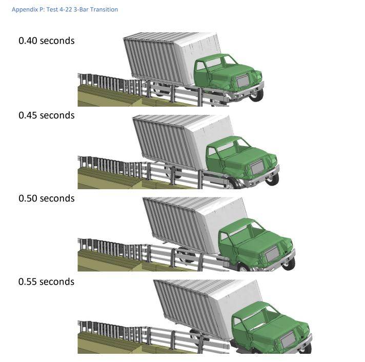
Figure P-3. [Continued] Sequential views from analysis of MASH Test 4-22 for AGT 3-Bar transition from an oblique viewpoint.
