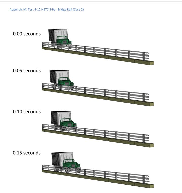
Figure M-3. Sequential views from analysis of MASH Test 4-12 for NETC 3-Bar bridge rail from an oblique viewpoint – Case 2.
