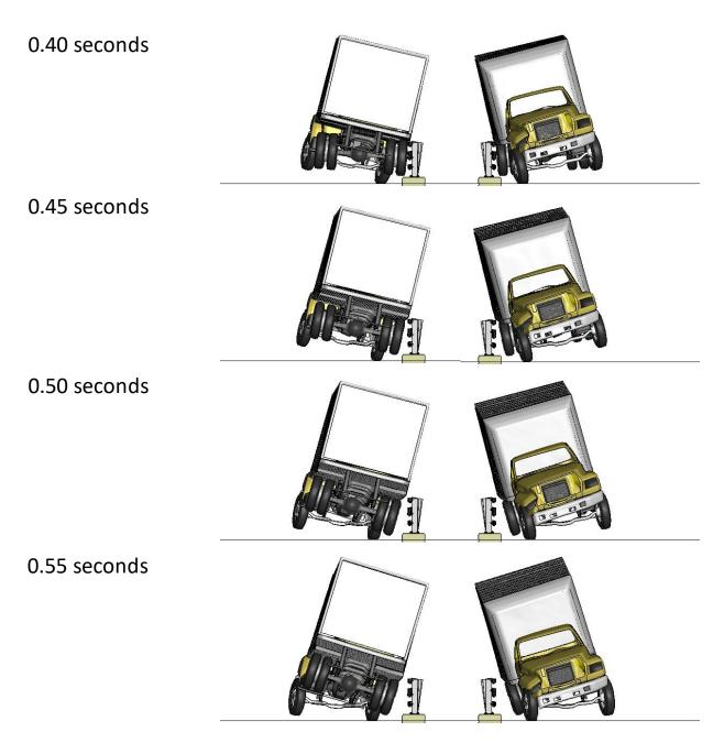
Figure K-2. [Continued] Sequential views from analysis of MASH Test 4-12 for NETC 3-Bar bridge rail from upstream and downstream viewpoints – Case 1.
