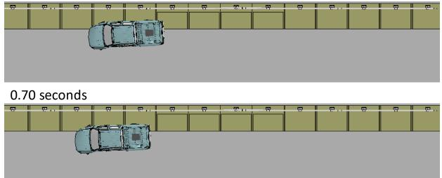
Figure R-1. [Continued] Sequential views from analysis of MASH Test 4-11 for NETC 4-Bar bridge rail from an overhead viewpoint.
