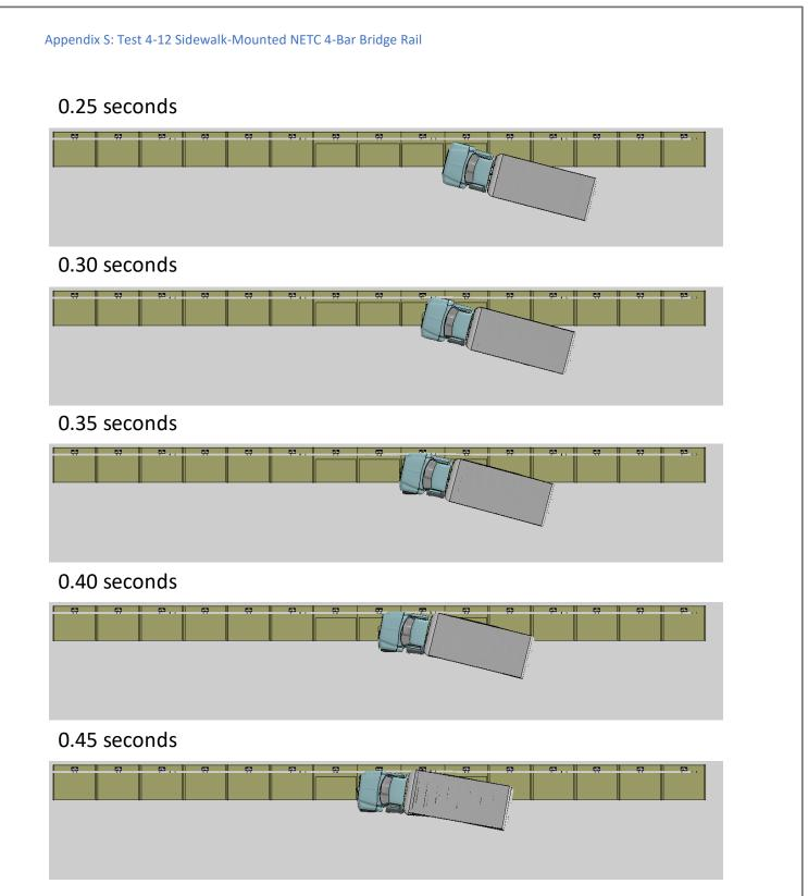
Figure S-1. [Continued] Sequential views from analysis of MASH Test 4-12 for NETC 4-Bar bridge rail from an overhead viewpoint.
