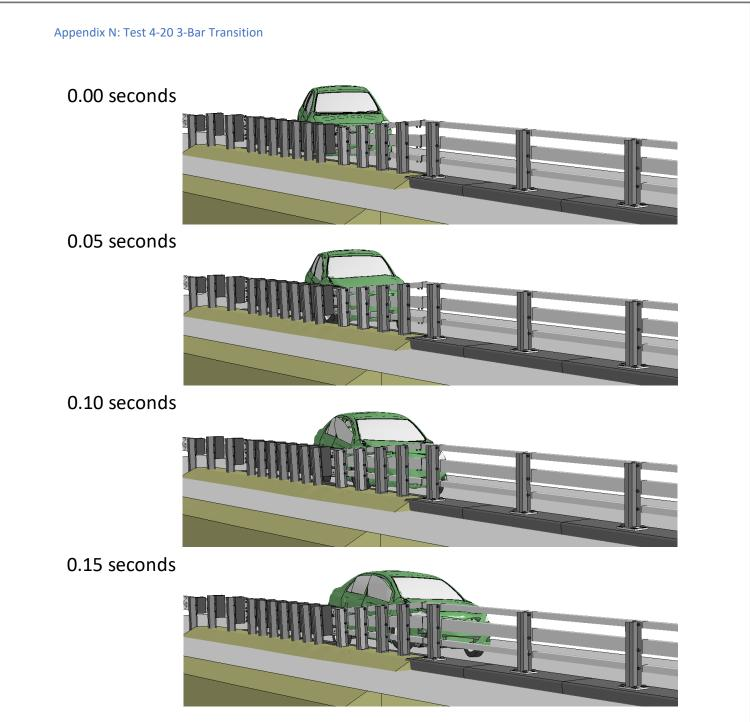
Figure N-3. Sequential views from analysis of MASH Test 4-20 for AGT 3-Bar transition from an oblique viewpoint.
