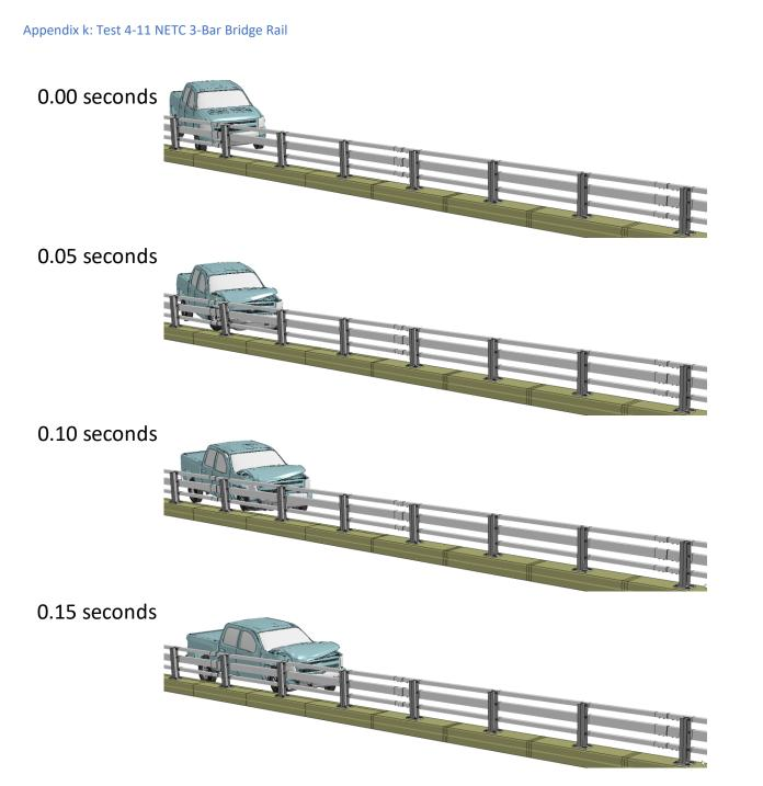
Figure K-3. Sequential views from analysis of MASH Test 4-11 for NETC 3-Bar bridge rail from an oblique viewpoint.
