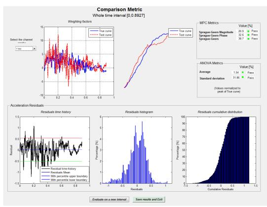
Figure 2c: RSVVP Results – Lateral Acceleration
