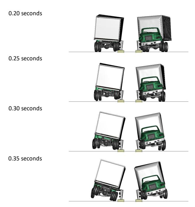
Figure M-2. [Continued] Sequential views from analysis of MASH Test 4-12 for NETC 3-Bar bridge rail from upstream and downstream viewpoints – Case 2.
