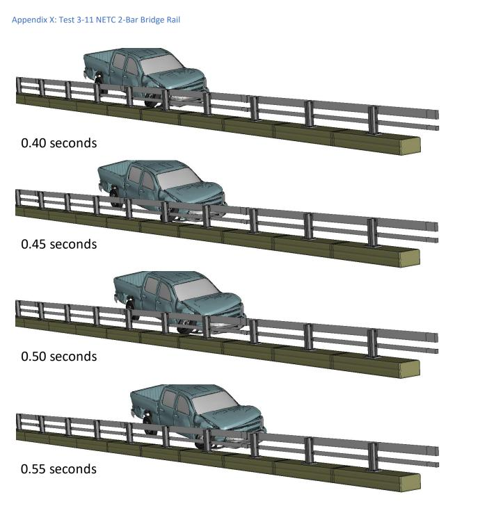
Figure X-3. [Continued] Sequential views from analysis of MASH Test 3-11 for NETC 2-Bar bridge rail from an oblique viewpoint.
