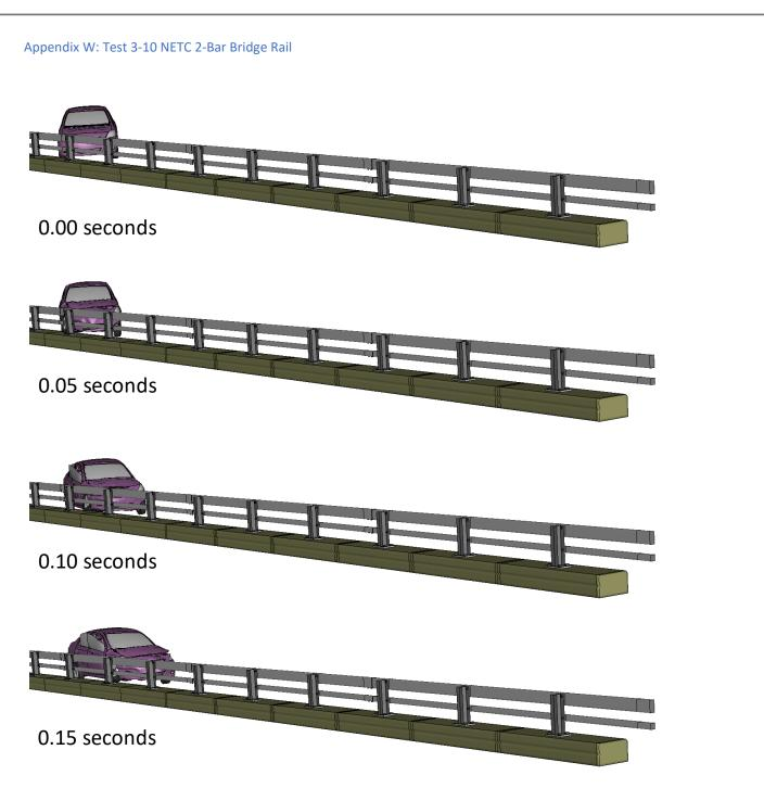
Figure W-3. Sequential views from analysis of MASH Test 3-10 for NETC 2-Bar bridge rail from an oblique viewpoint.
