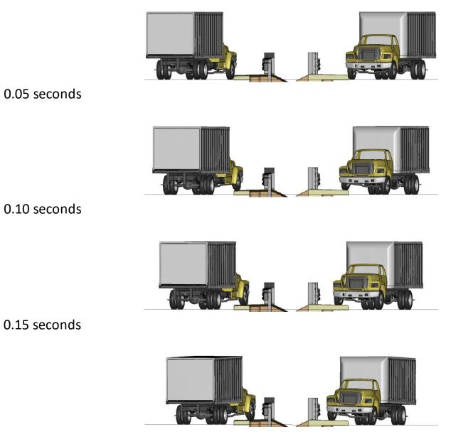
Figure V-2. Sequential views from analysis of MASH Test 4-22 for AGT 4-Bar bridge rail from upstream and downstream viewpoints.
