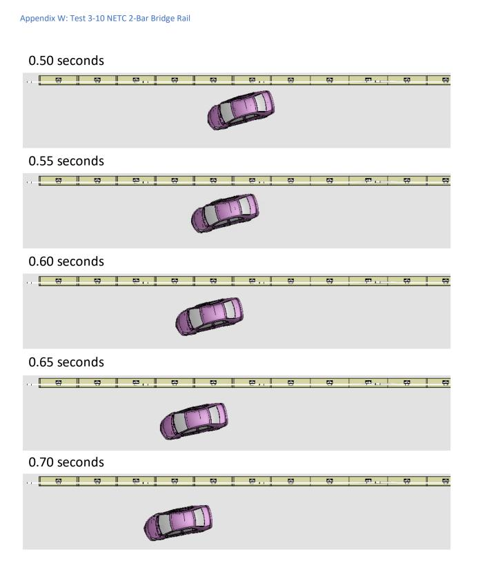
Figure W-1. [Continued] Sequential views from analysis of MASH Test 3-10 for NETC 2-Bar bridge rail from an overhead viewpoint.
