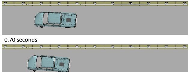
Figure K-1. [Continued] Sequential views from analysis of MASH Test 4-11 for NETC 3-Bar bridge rail from an overhead viewpoint.
