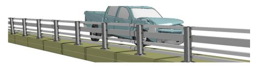
Figure R-3. [Continued] Sequential views from analysis of MASH Test 4-11 for NETC 4-Bar bridge rail from an oblique viewpoint.
