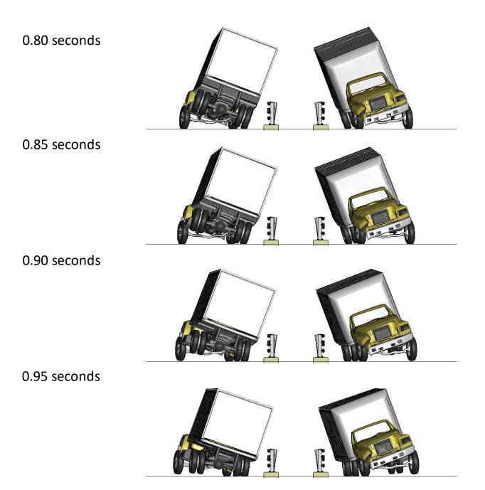
Figure K-2. [Continued] Sequential views from analysis of MASH Test 4-12 for NETC 3-Bar bridge rail from upstream and downstream viewpoints – Case 1.
