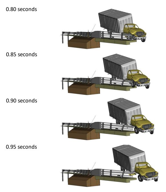
Figure V-3. [Continued] Sequential views from analysis of MASH Test 4-22 for AGT 4-Bar bridge rail from an oblique viewpoint.
