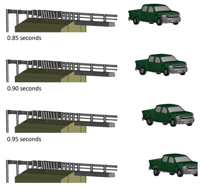
Figure Z-3. [Continued] Sequential views from analysis of MASH Test 3-21 for AGT 2-Bar bridge rail from an oblique viewpoint.
