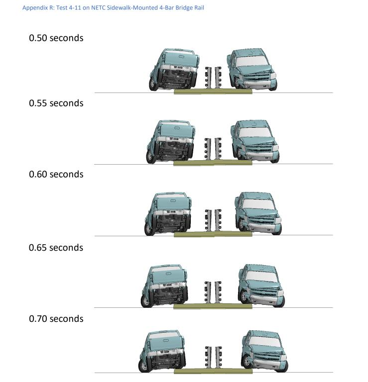
Figure R-2. [Continued] Sequential views from analysis of MASH Test 4-11 for NETC 4-Bar bridge rail from upstream and downstream viewpoints.
