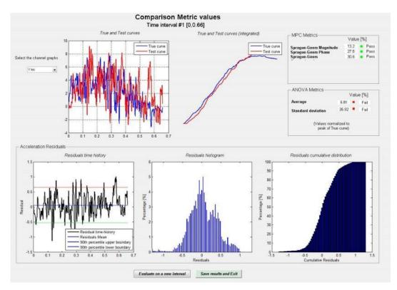
Figure 2c: RSVVP Results – Lateral Acceleration
