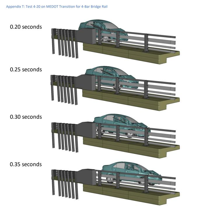
Figure T-3. [Continued] Sequential views from analysis of MASH Test 4-20 for AGT 4-Bar bridge rail from an oblique viewpoint.
