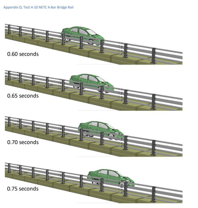
Figure Q-3. [Continued] Sequential views from analysis of MASH Test 4-10 for NETC 4-Bar bridge rail from an oblique viewpoint.
