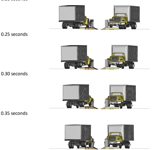
Figure V-2. [Continued] Sequential views from analysis of MASH Test 4-22 for AGT 4-Bar bridge rail from upstream and downstream viewpoints.
