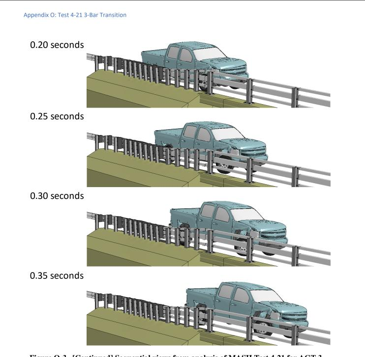
Figure O-3. [Continued] Sequential views from analysis of MASH Test 4-21 for AGT 3-Bar transition from from an oblique viewpoint.
