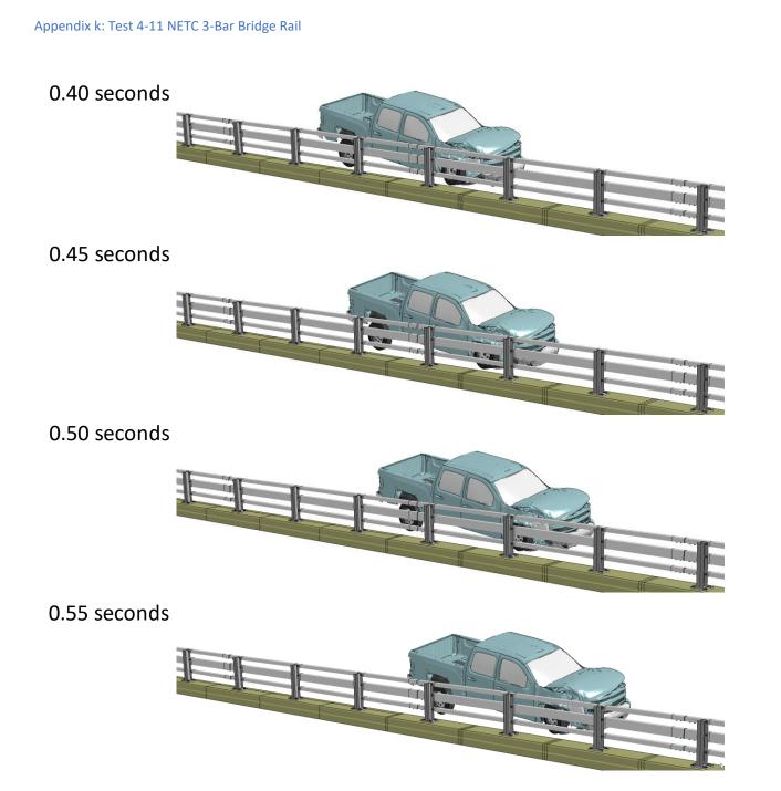
Figure K-3. [Continued] Sequential views from analysis of MASH Test 4-11 for NETC 3-Bar bridge rail from an oblique viewpoint.
