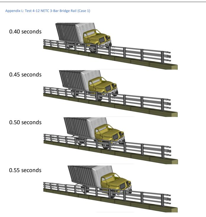
Figure K-3. [Continued] Sequential views from analysis of MASH Test 4-12 for NETC 3-Bar bridge rail from an oblique viewpoint – Case 1.
