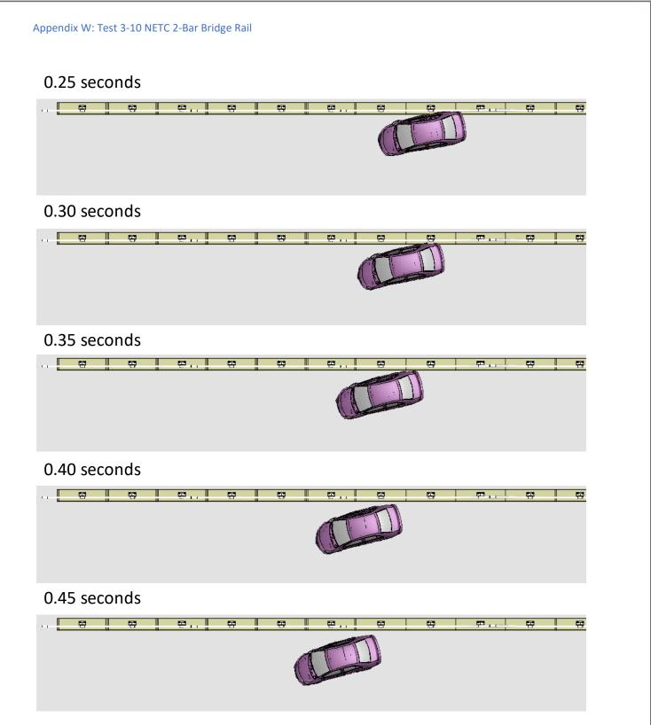
Figure W-1. [Continued] Sequential views from analysis of MASH Test 3-10 for NETC 2-Bar bridge rail from an overhead viewpoint.
