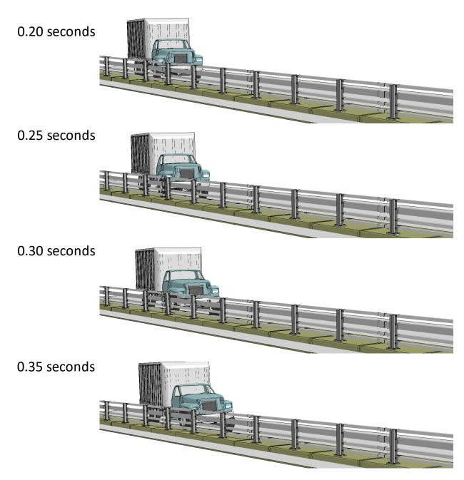
Figure S-3. [Continued] Sequential views from analysis of MASH Test 4-12 for NETC 4-Bar bridge rail from an oblique viewpoint.
