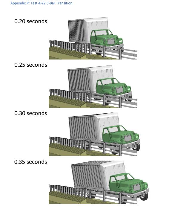
Figure P-3. [Continued] Sequential views from analysis of MASH Test 4-22 for AGT 3-Bar transition from an oblique viewpoint.
