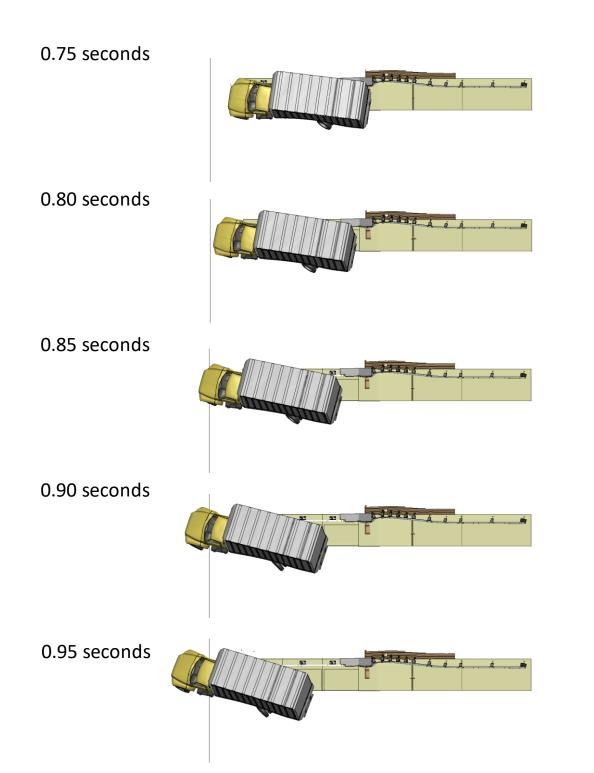
Figure V-1. [Continued] Sequential views from analysis of MASH Test 4-22 for AGT 4-Bar bridge rail from an overhead viewpoint.
