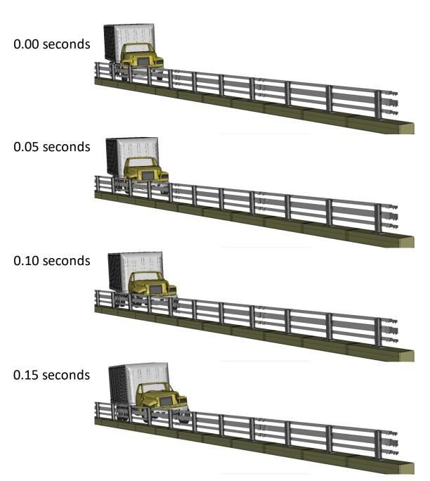
Figure K-3. Sequential views from analysis of MASH Test 4-12 for NETC 3-Bar bridge rail from an oblique viewpoint – Case 1.
