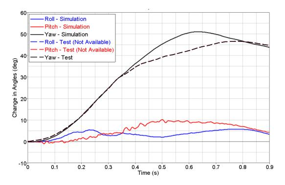
Figure 4: Change in Vehicle Angle
