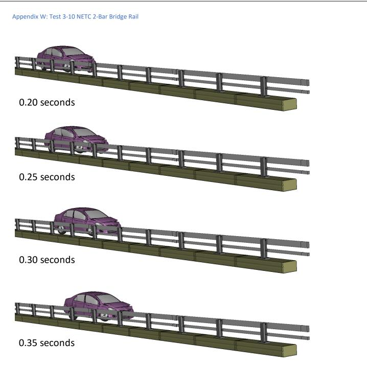
Figure W-3. [Continued] Sequential views from analysis of MASH Test 3-10 for NETC 2-Bar bridge rail from an oblique viewpoint.
