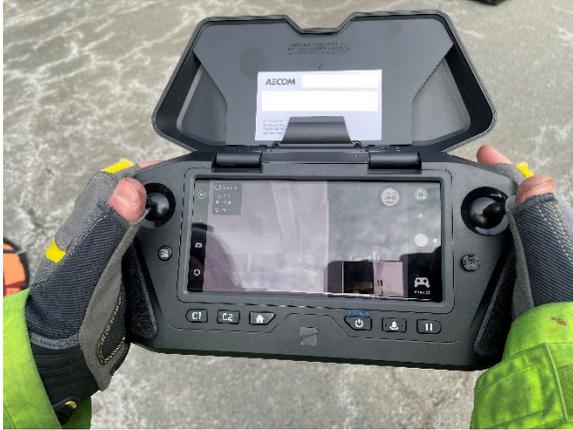
*Figure 62 - Screen Glare on Skydio Enterprise Controller*
