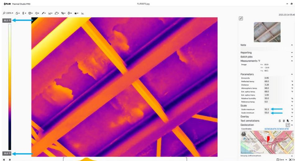
Figure 33 - Manual Entry for Minimum and Maximum Temperatures
