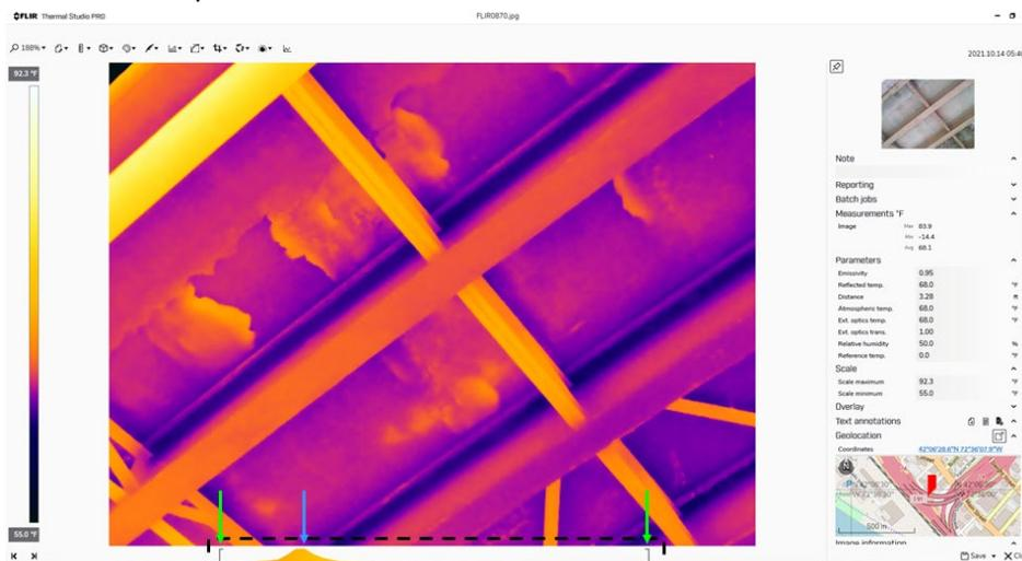
Figure 34 - Adjusting Temperature Values Using Histogram
