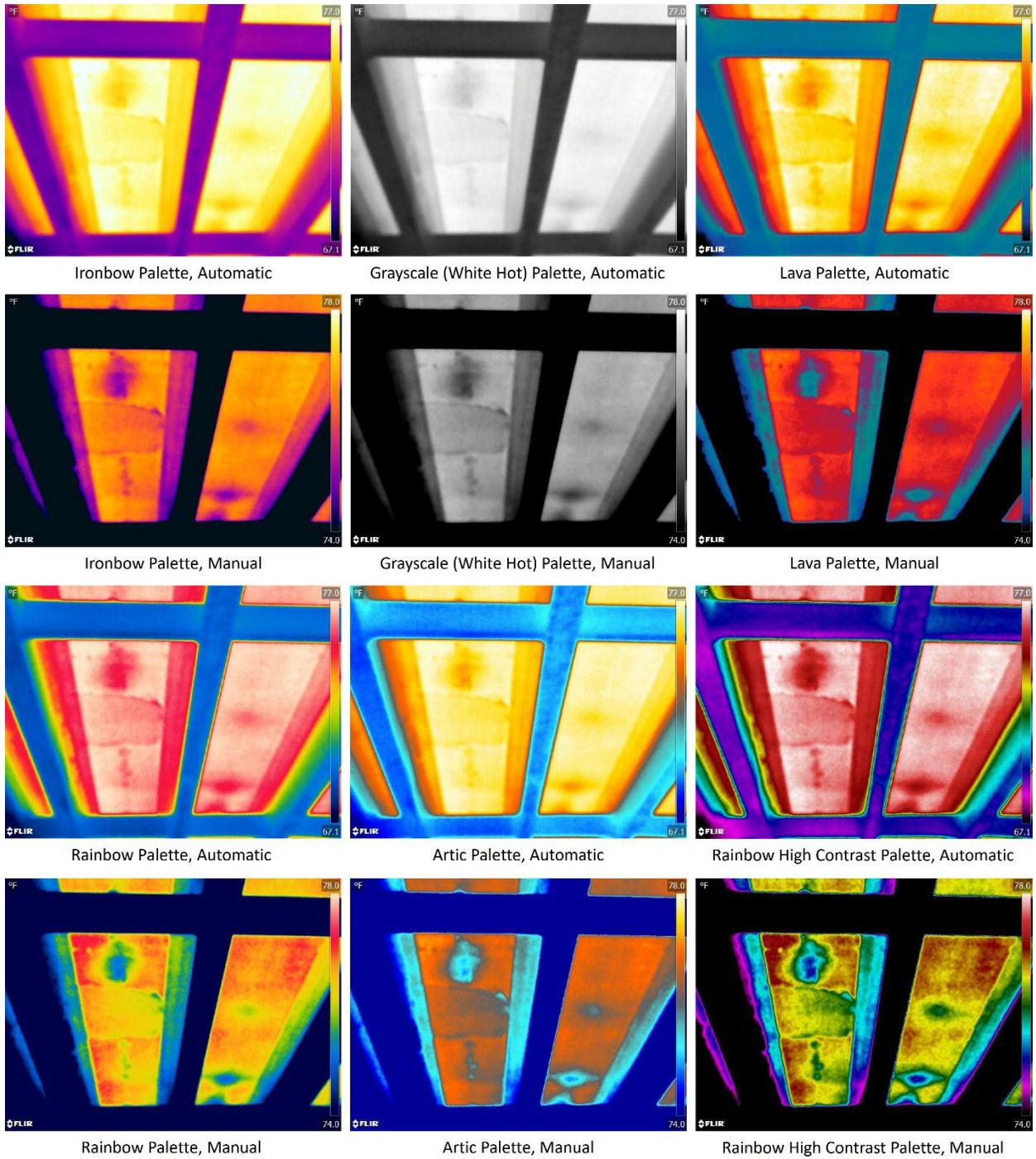
Figure 30 - Comparison of Color Palettes for Flir E96
