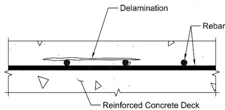
*Figure 1 - Concrete Delamination*
