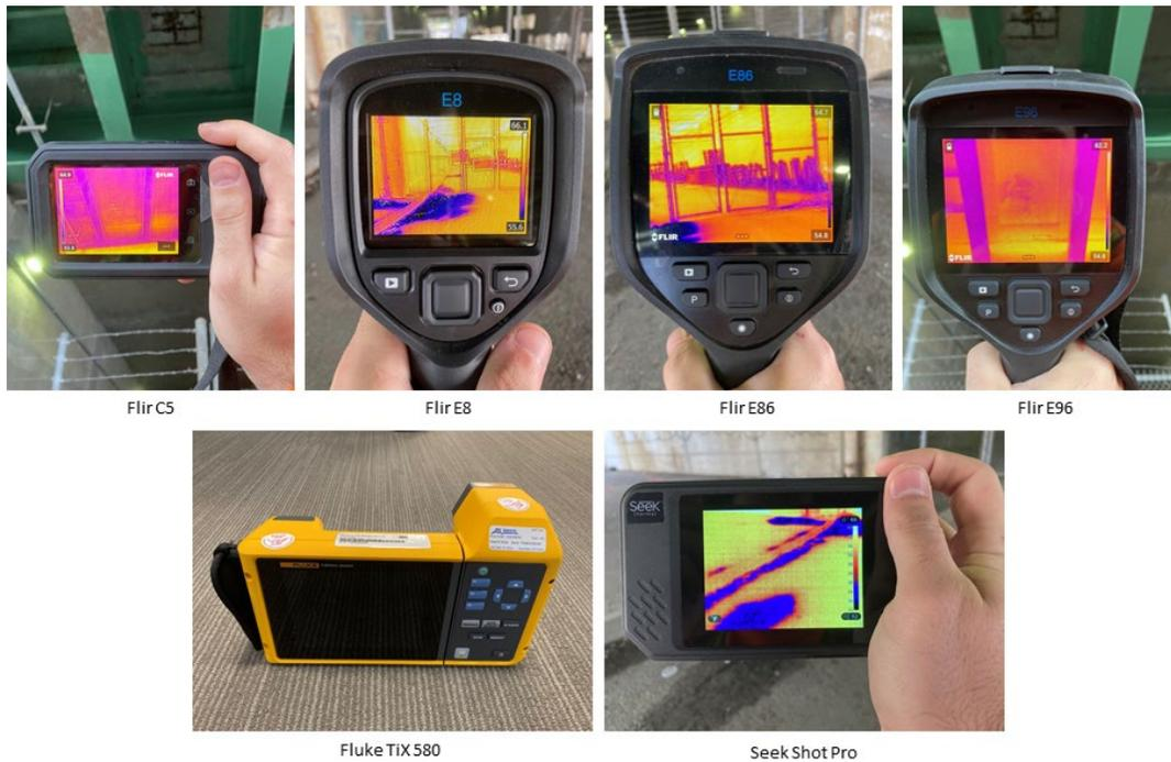
Figure 10 - Field-Tested Handheld Thermal Cameras
