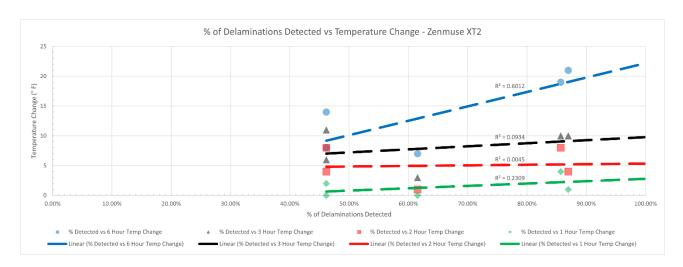
Figure 23 - Delamination Detection versus Temperature Change for Zenmuse XT2
