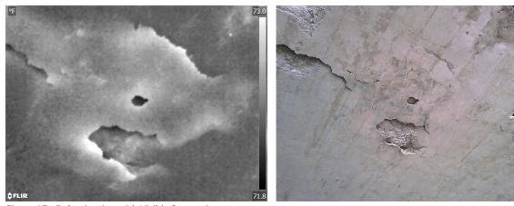
Figure 17 - Delamination with Visible Separation
