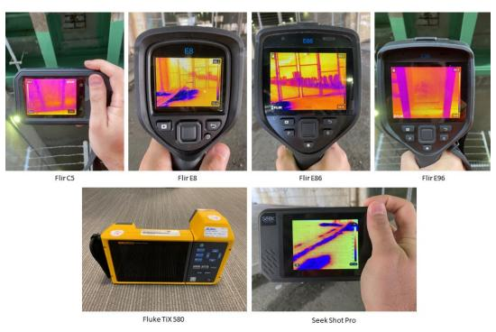
Figure 10 - Field-Tested Handheld Thermal Cameras
