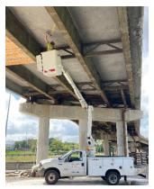
Figure 4 - Inspector Hammer Sounding Deck
