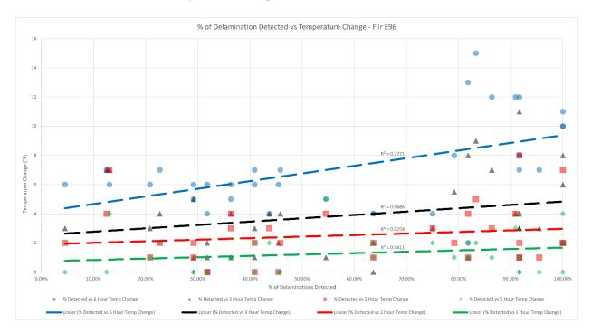
Figure 22 - Delamination Detection versus Temperature Change for Flir E96
