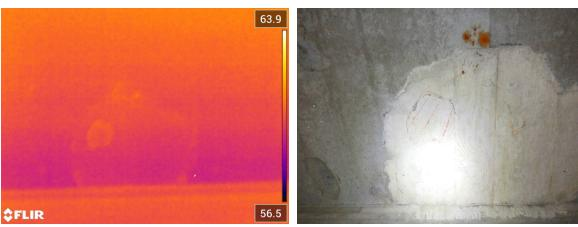
Figure 20 - Delamination within Otherwise Sound Patch
