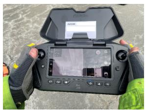
Figure 62 - Screen Glare on Skydio Enterprise Controller
