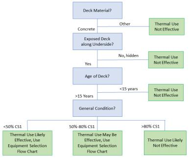
Figure 24 - Flow Chart to Determine Effectiveness for Underside of Bridge Decks
