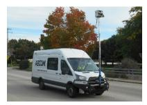
Figure 5 - Van Equipped with IR Sensor
