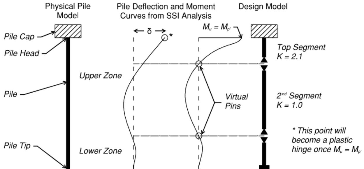
Figure 3-2: Pile Design Model When  $M_u = M_p'$
