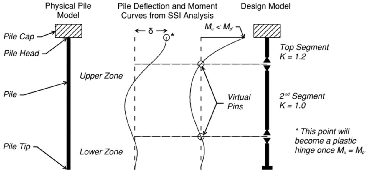
Figure 3-1: Pile Design Model When  $M_u < M_p'$
