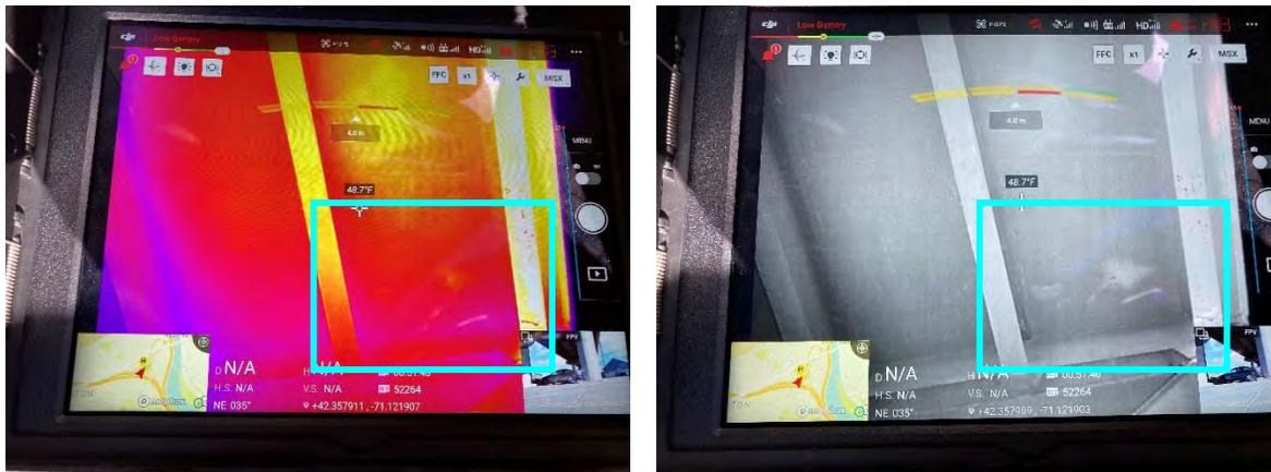
Figure 10 - Screen Shots of Ironbow and White Hot Color Palettes Showing Delamination
