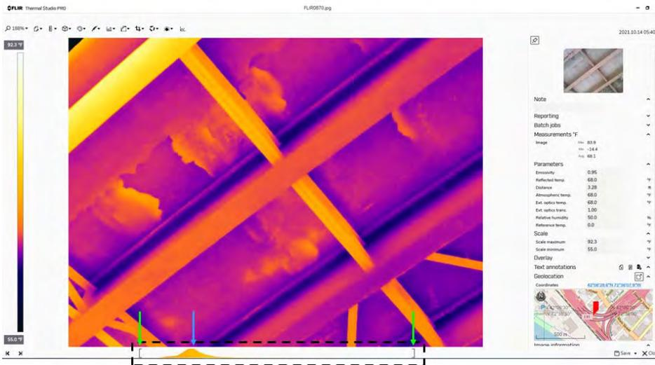
Figure 15 – Adjusting Temperature Values using Histogram
