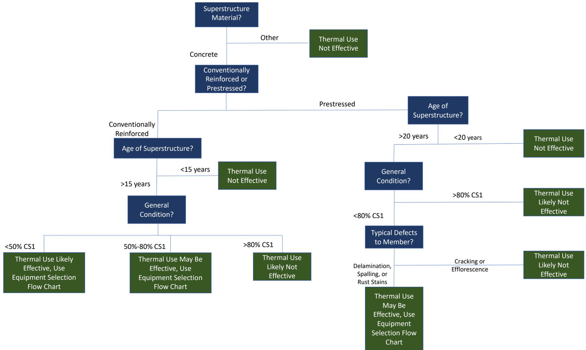
Flow Chart to Determine Effectiveness for Substructure Elements
