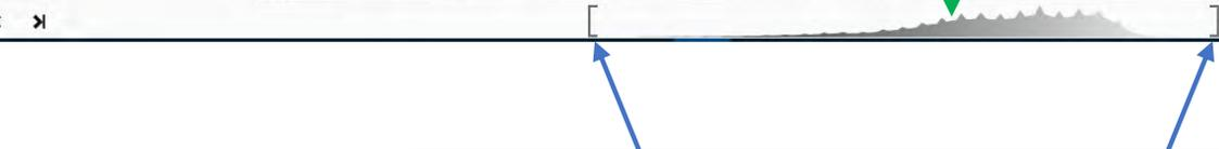
Hover cursor over bracket, the cursor will change to a horizontal line with arrows on either end. Once the cursor changes, it can be clicked and dragged to adjust the minimum/maximum temperature values
