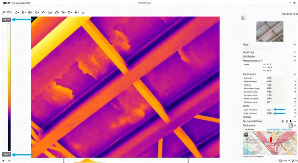
Figure 14 - Manual Entry for Minimum and Maximum Temperatures
