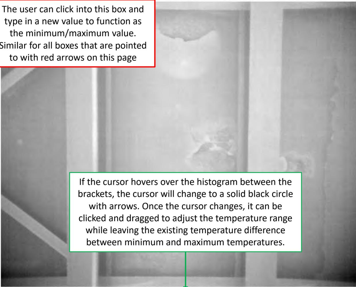
If the cursor hovers over the histogram between the brackets, the cursor will change to a solid black circle with arrows. Once the cursor changes, it can be clicked and dragged to adjust the temperature range while leaving the existing temperature difference between minimum and maximum temperatures.
