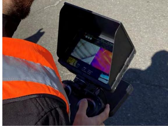
Figure 41 - Sun Shield on DJI Crystal Sky Tablet
