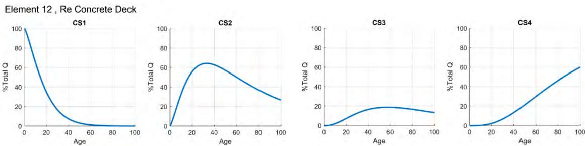
Figure 7 - Deterioration Curves for Reinforced Concrete Deck
