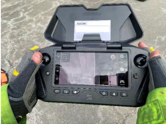
Figure 40 - Screen Glare on Skydio Enterprise Controller
