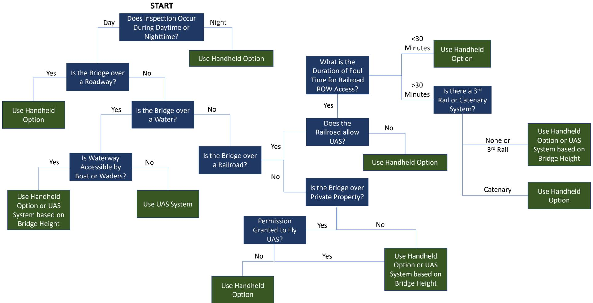
Flow Chart to Determine Effectiveness for Underside of Bridge Decks
