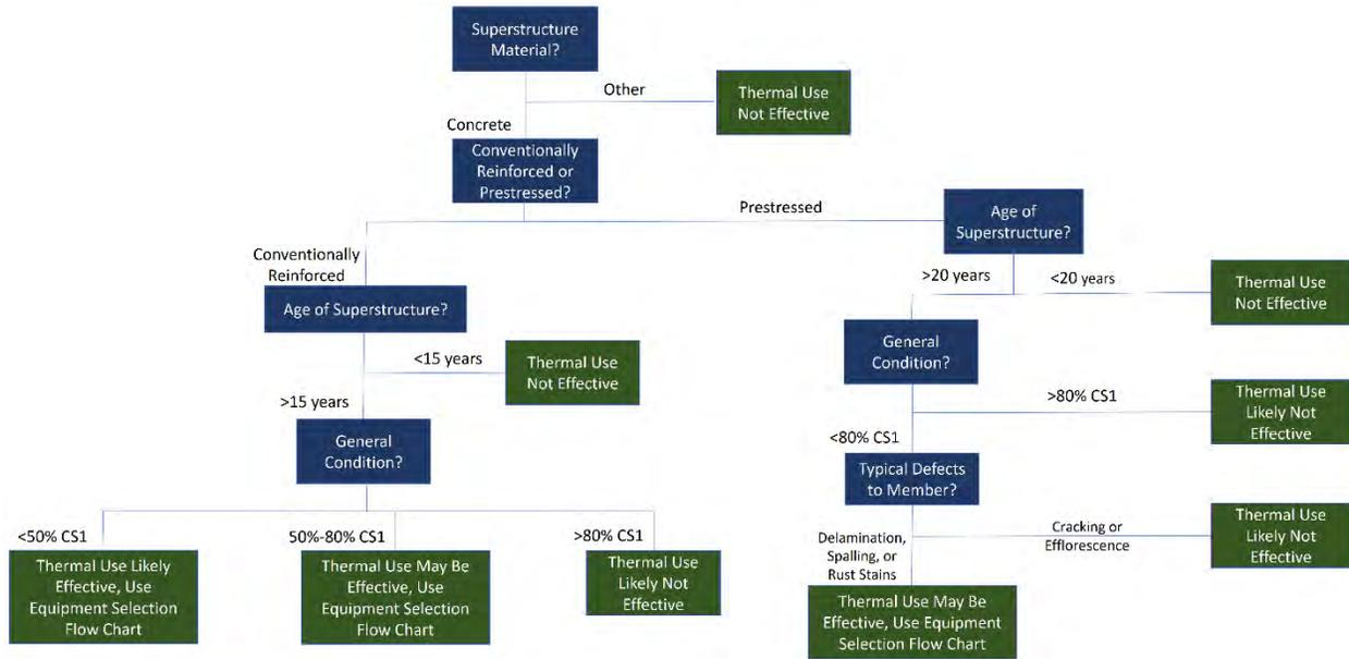
Figure 5 - Flow Chart to Determine Effectiveness for Superstructure Elements
