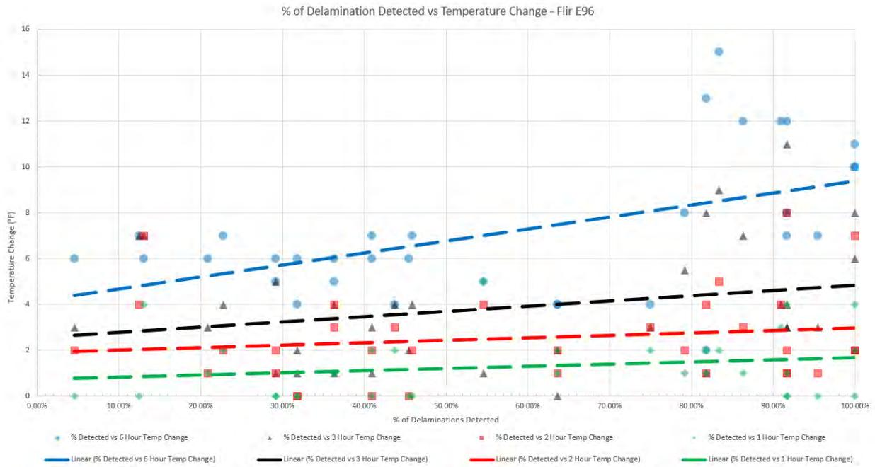
Figure 2 - Delamination Detection versus Temperature Change for Flir E96
