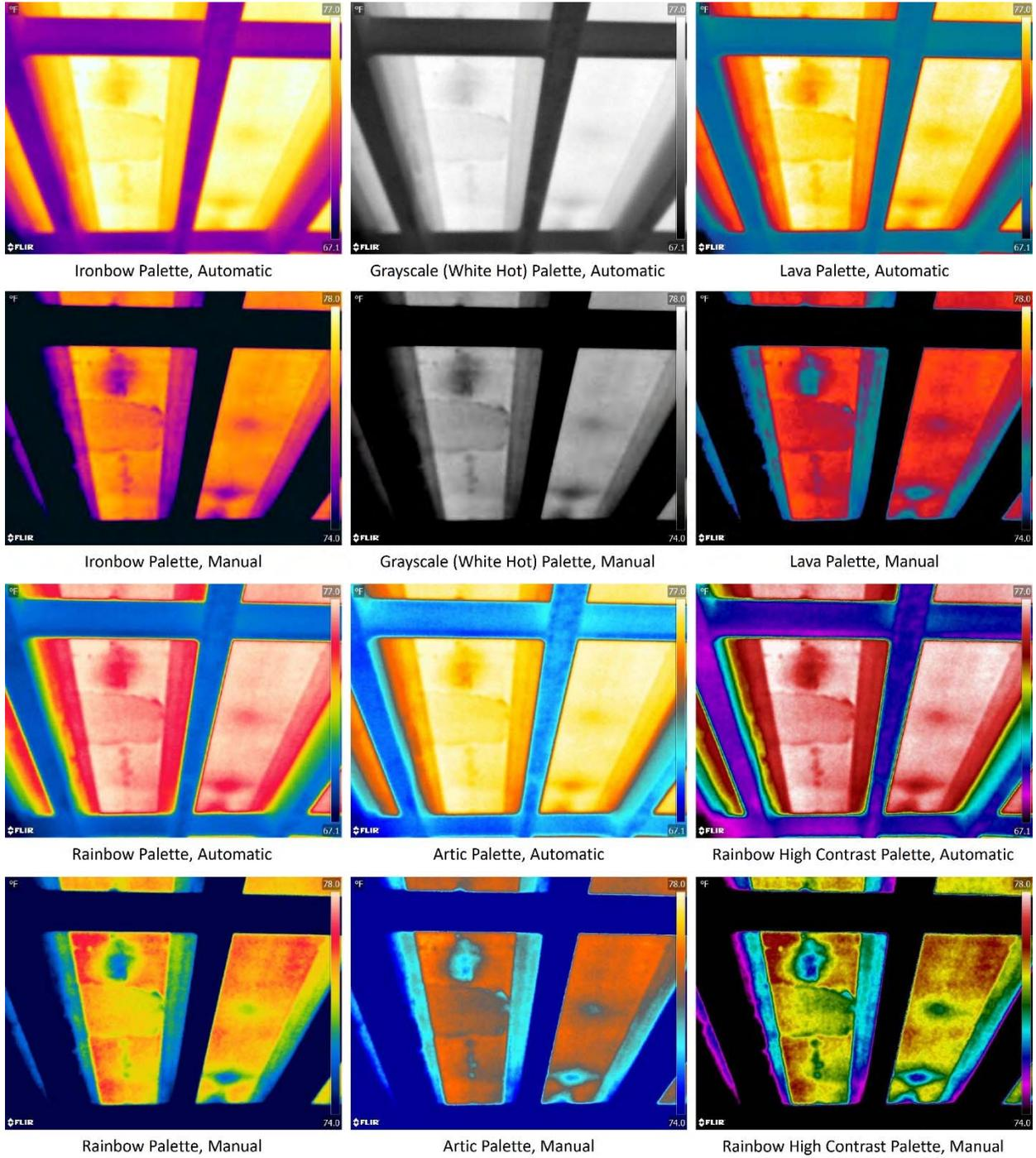
Figure 12 - Comparison of Color Palettes for Flir E96
