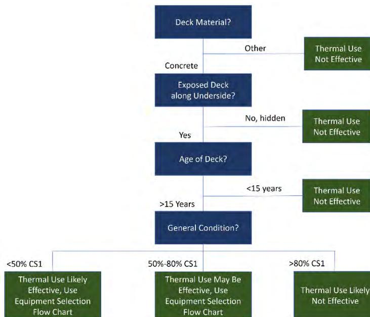
Figure 4 - Flow Chart to Determine Effectiveness for Deck Underside
