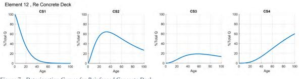
Figure 7 - Deterioration Curves for Reinforced Concrete Deck
