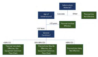
Figure 6 - Flow Chart to Determine Effectiveness for Substructure Elements
