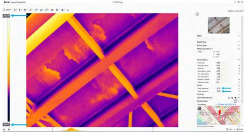
Figure 14 - Manual Entry for Minimum and Maximum Temperatures
