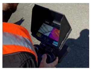
Figure 41 - Sun Shield on DJI Crystal Sky Tablet
