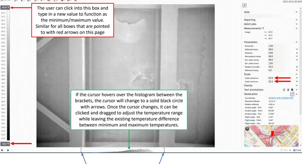
Hover cursor over bracket, the cursor will change to a horizontal line with arrows on either end. One the cursor changes, it can be clicked and dragged to adjust the minimum/maximum temperature values
