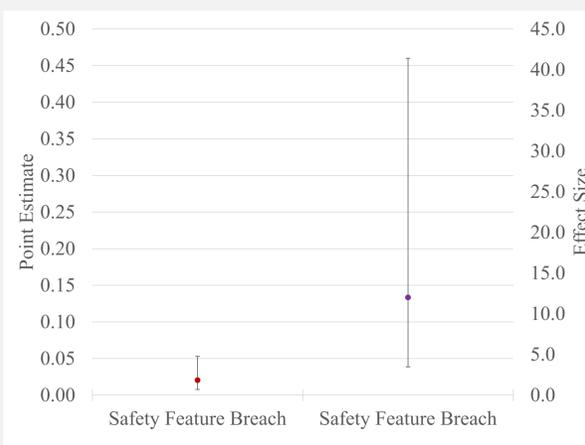
Proportion of NETC bridge rail and AGT crashes that breach the barrier (left); Effect Size for breaching the barrier (right) – full dataset.
