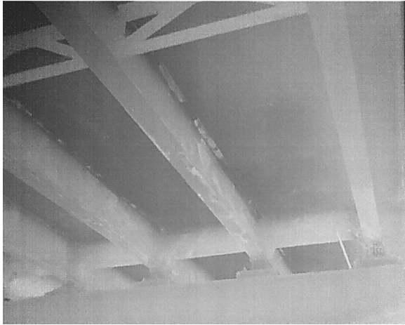
Figure 41 - Temperature Differential caused by Paint Failure along Top Flange
