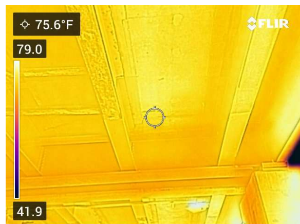
Figure 35 - Visible Sky affecting Thermal Span
