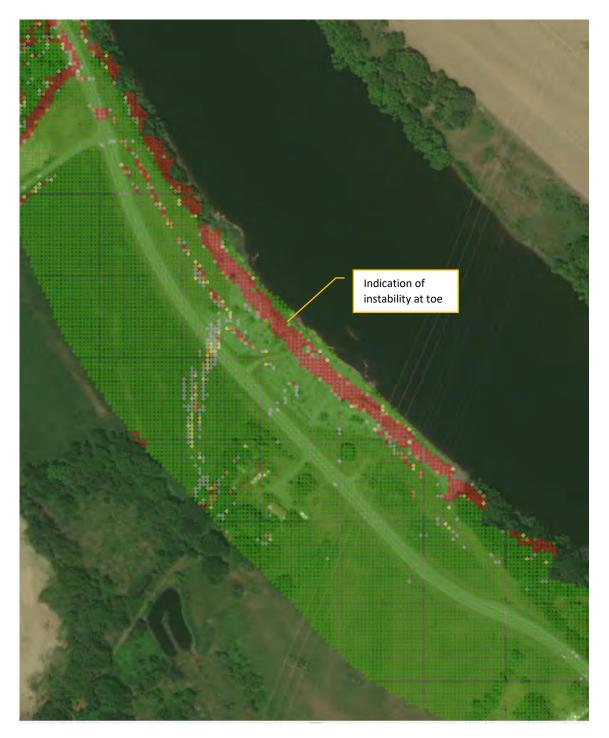
Figure 2: Slope Failure Site at Route 136
