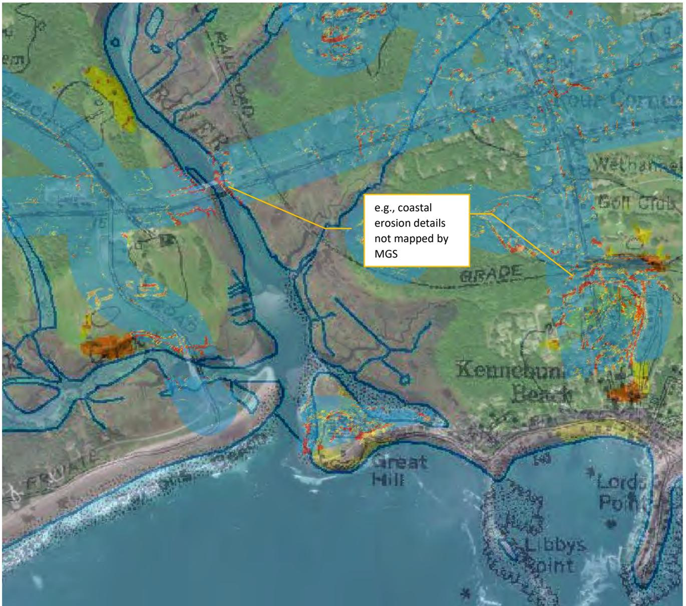
Note: Aerial image and MGS landslide susceptibility map overlaid with GZA computed slope stability hazard index. PDF is slightly offset due to projection.
