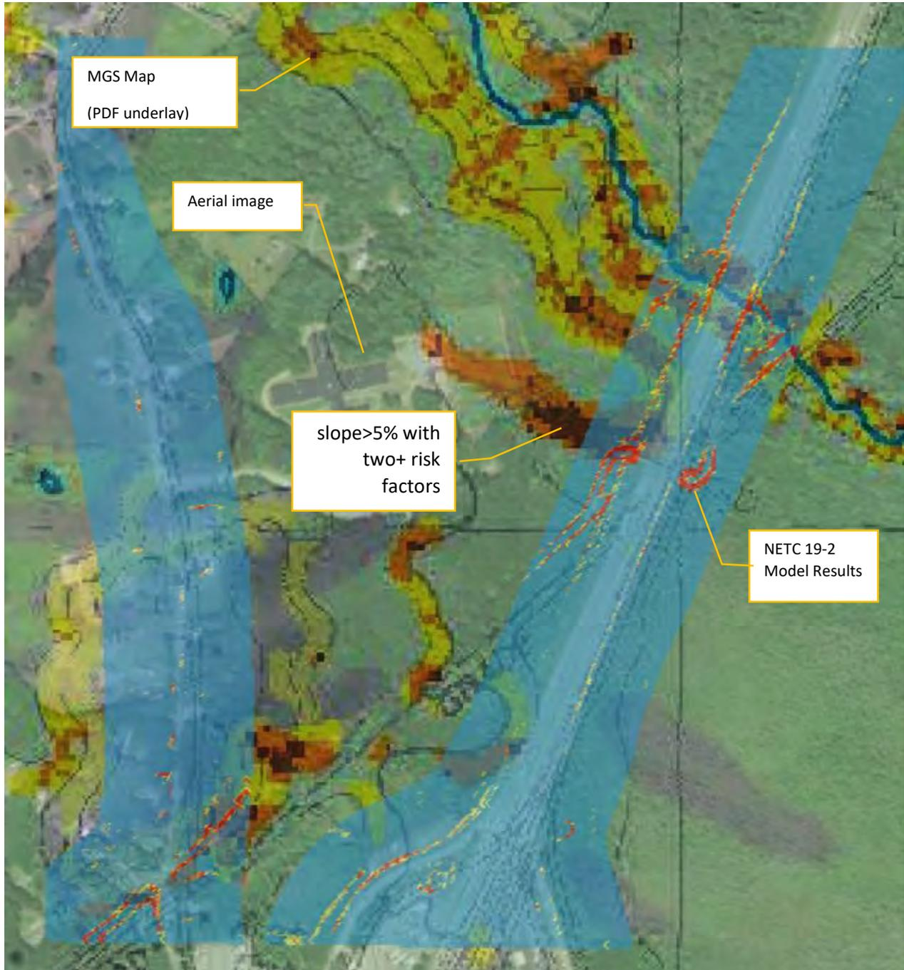
Note: Aerial image and MGS landslide susceptibility map overlaid with NETC 19-2 computed slope stability hazard index. PDF is slightly offset due to projection.
