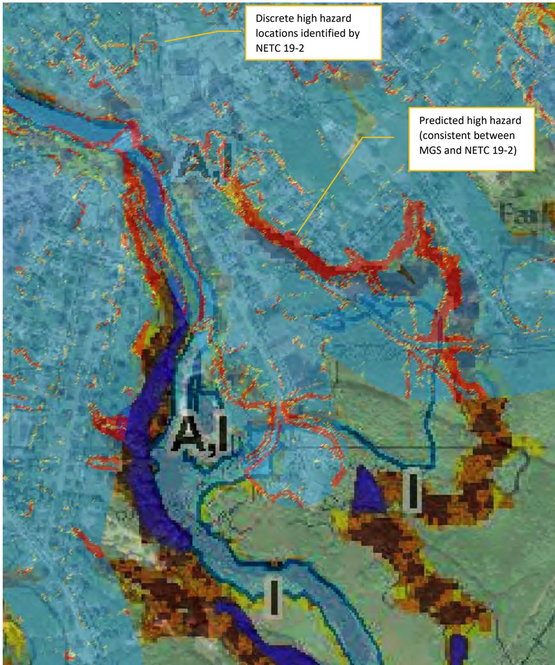
Note: Aerial image and MGS landslide susceptibility map overlaid with GZA computed slope stability hazard index. PDF is slightly offset due to projection.
