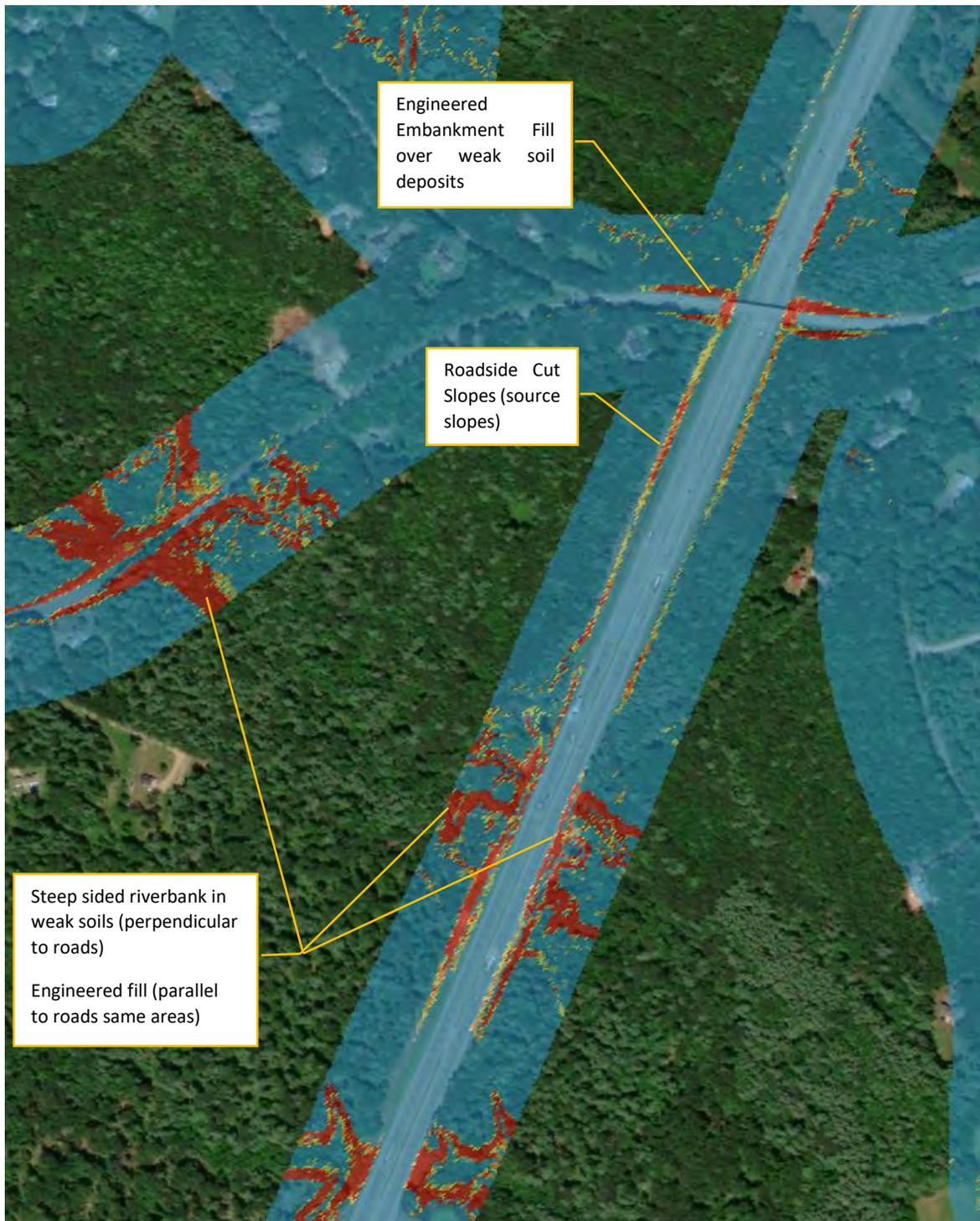
Note: Manmade slopes not part of underlying surficial geology layer used as model input.
