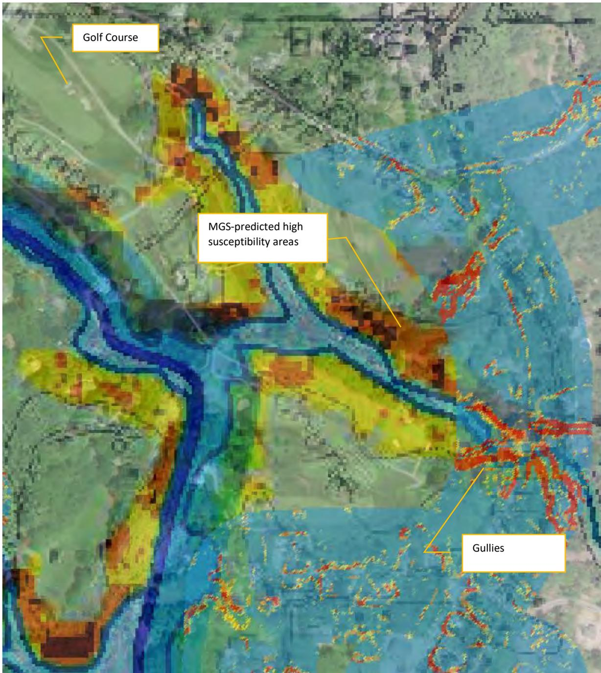
Note: Aerial image and MGS landslide susceptibility map overlaid with GZA computed slope stability hazard index. PDF is slightly offset due to projection.
