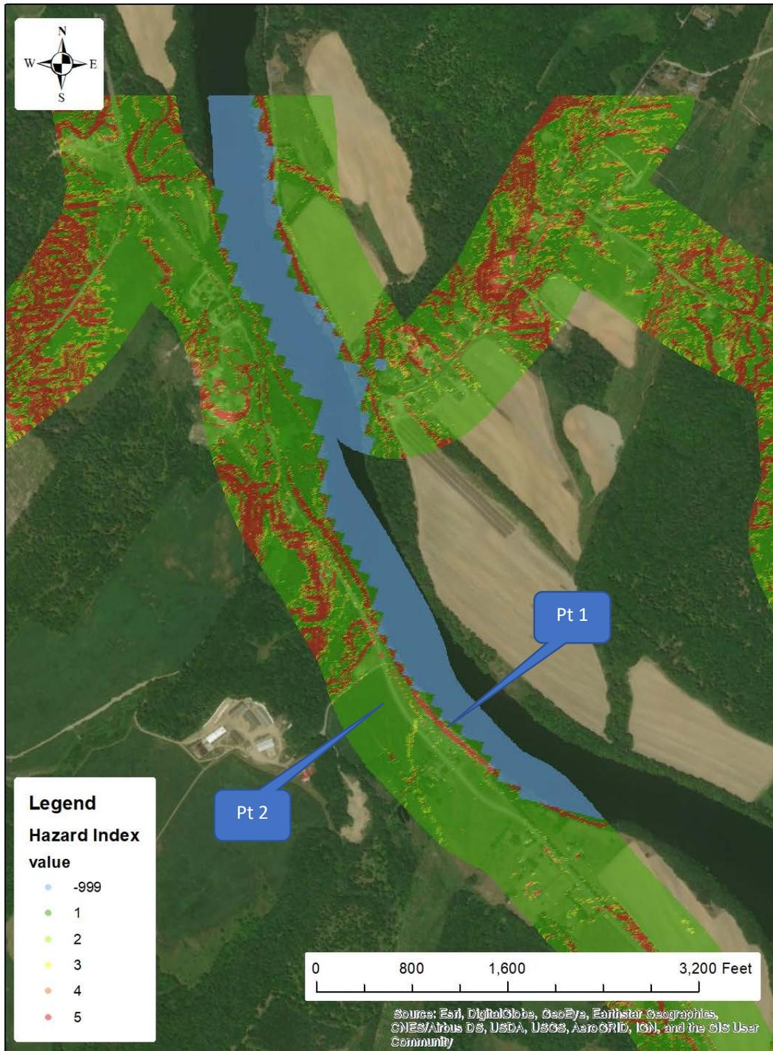
Note: Index values of 4 and 5 indicate marginal stability and instability per GZA’s modeling results. “-999” denotes area covered by water. Key parameters for Point locations Pt1 and Pt2 shown in Figure 9.
