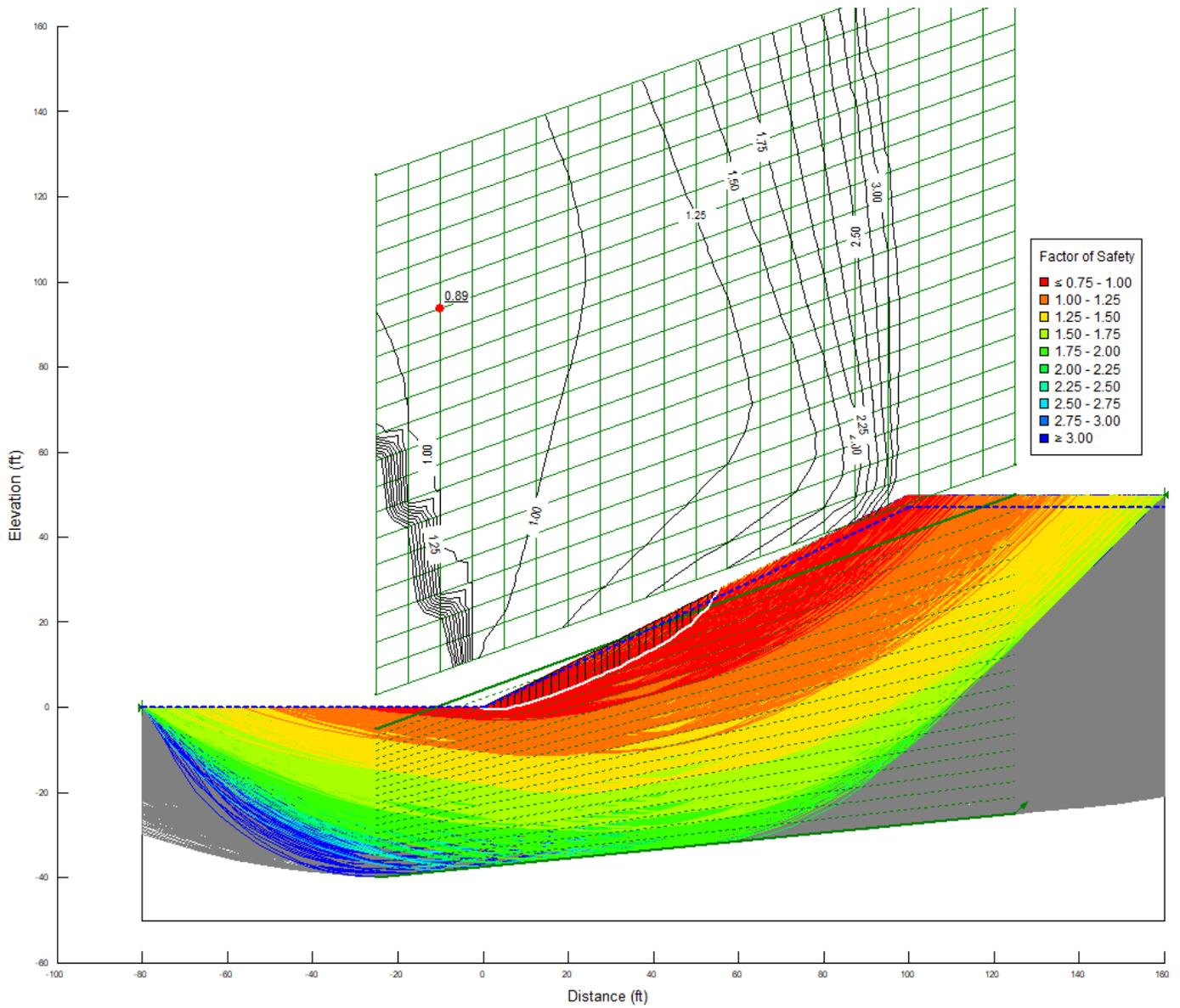
Figure A-11: SLOPE/W-Calculated Factor of Safety Results – Medium Stiff Clay (C2) on 2:1 Slope
