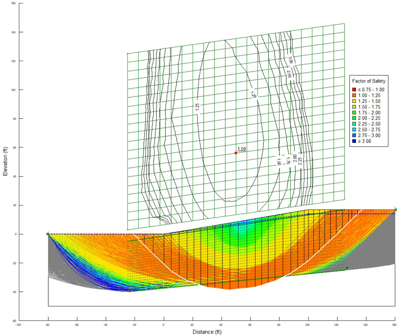
**Figure A-3: SLOPE/W-Calculated Factor of Safety Results – Loose Sand (G1) on 4:1 Slope**
