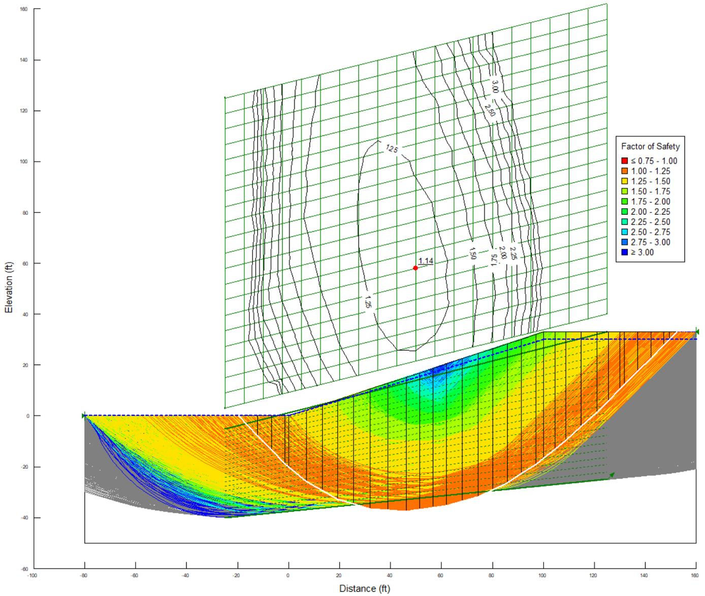
Figure A-9: SLOPE/W-Calculated Factor of Safety Results – Medium Dense Sand (G2) on 2:1 Slope
