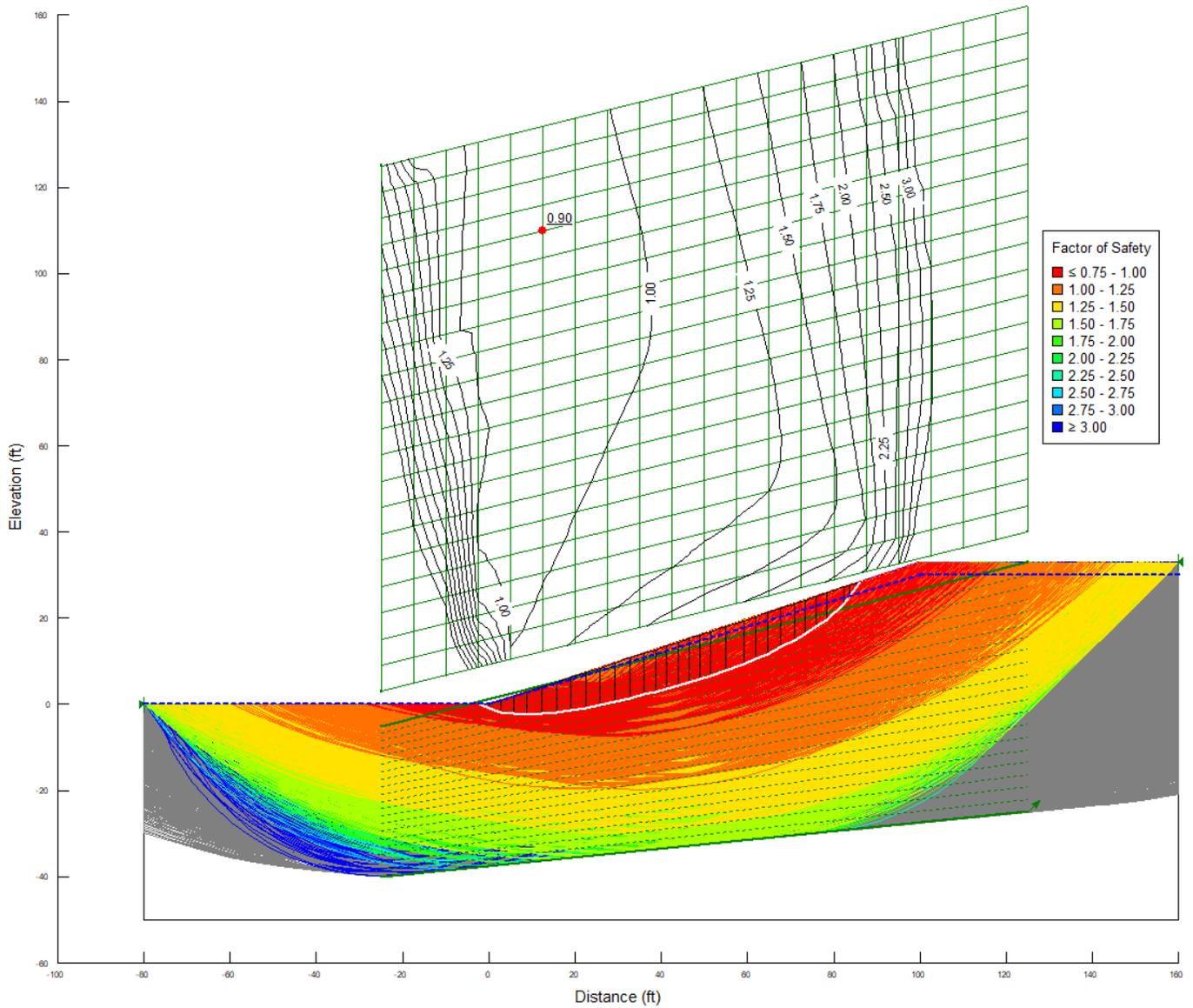
Figure A-6: SLOPE/W-Calculated Factor of Safety Results – Medium Dense Sand (G1) on 3:1 Slope
