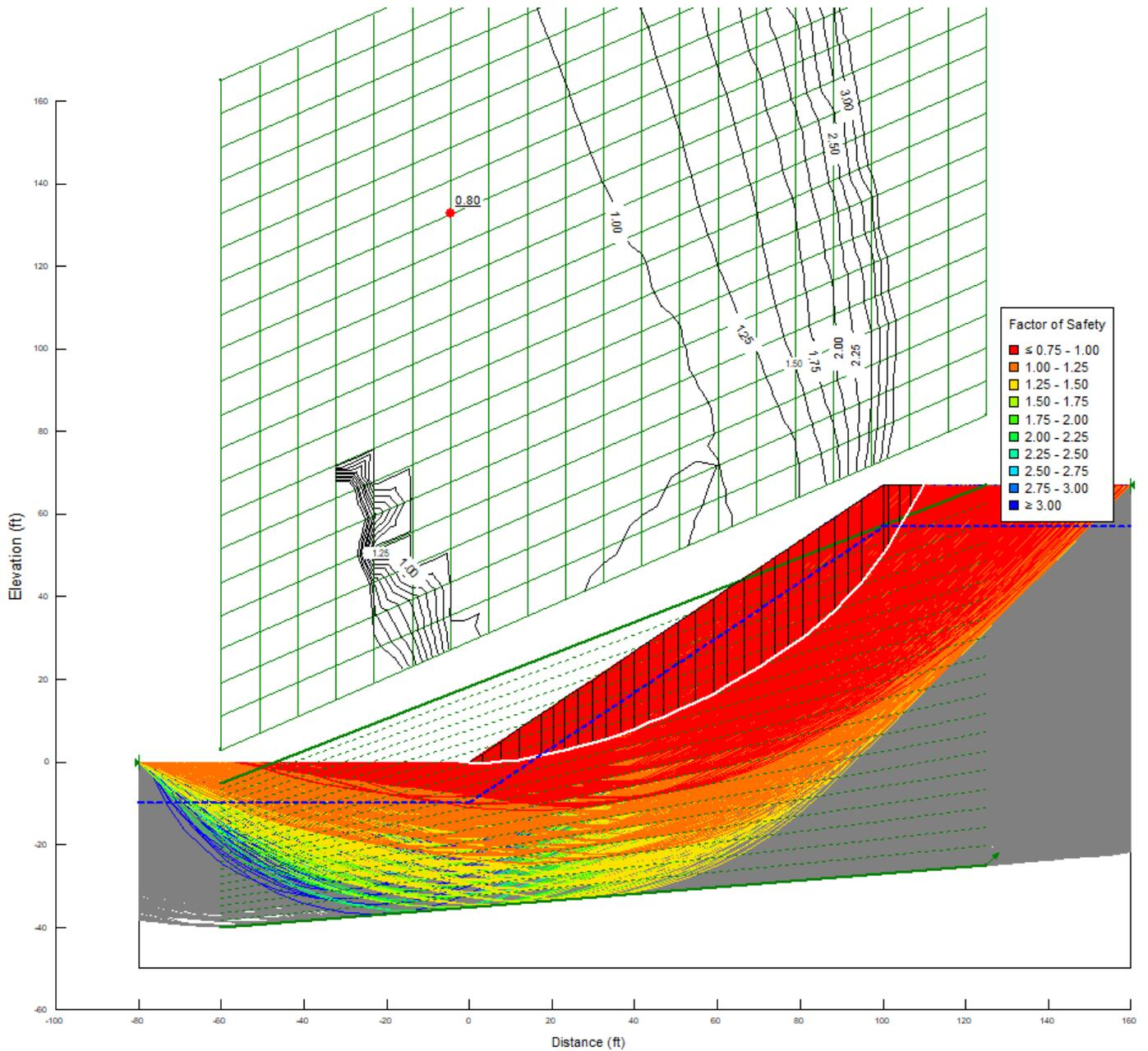
Figure A-13: SLOPE/W-Calculated Factor of Safety Results – Dense Sand (G3) on 1.5:1 Slope
