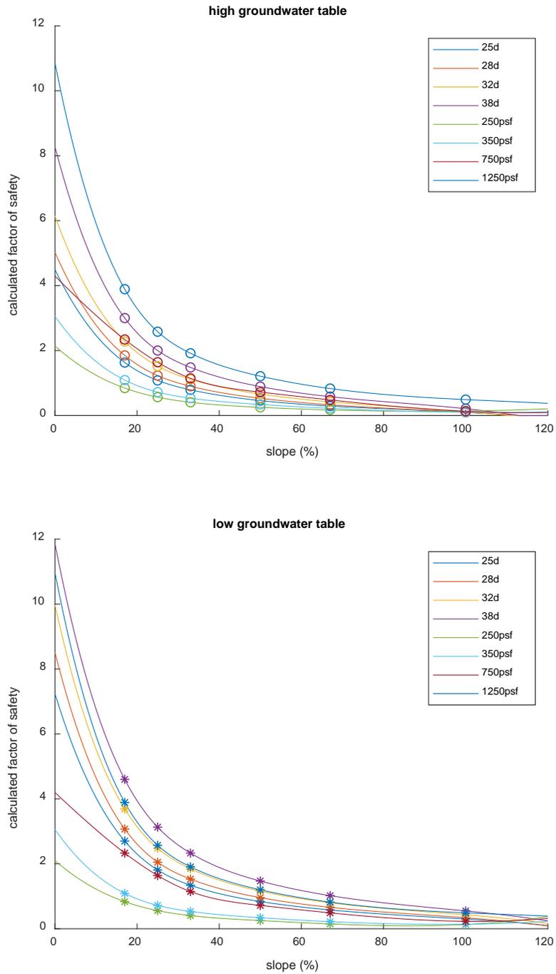
Note: Open circle or asterisk denotes SLOPE/W calculated values for both high and low groundwater conditions; curve denotes MATLAB spline-interpolated values at 1% intervals.
