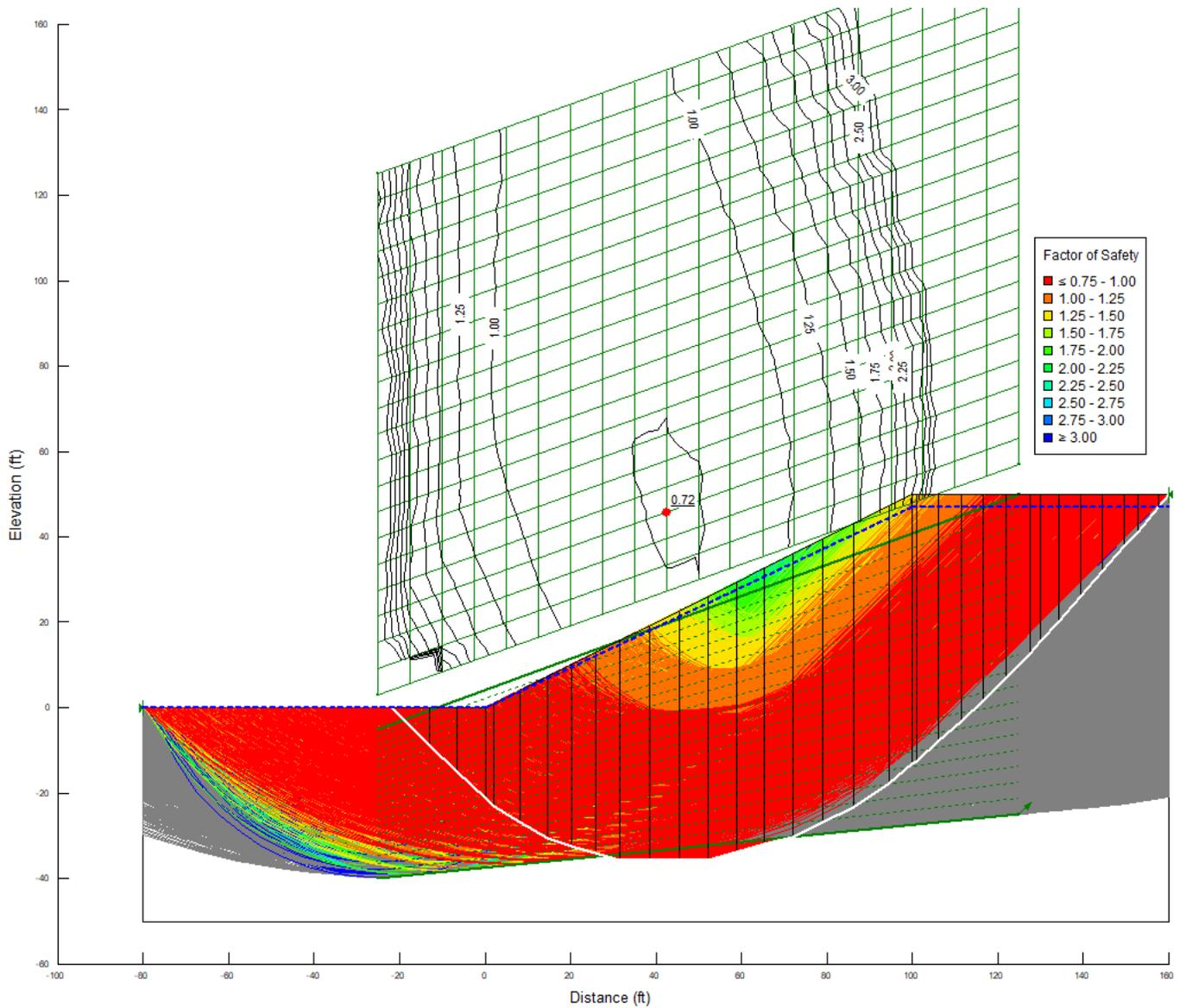
Figure A-12: SLOPE/W-Calculated Factor of Safety Results – Medium Dense Sand (G2) on 1.5:1 Slope
