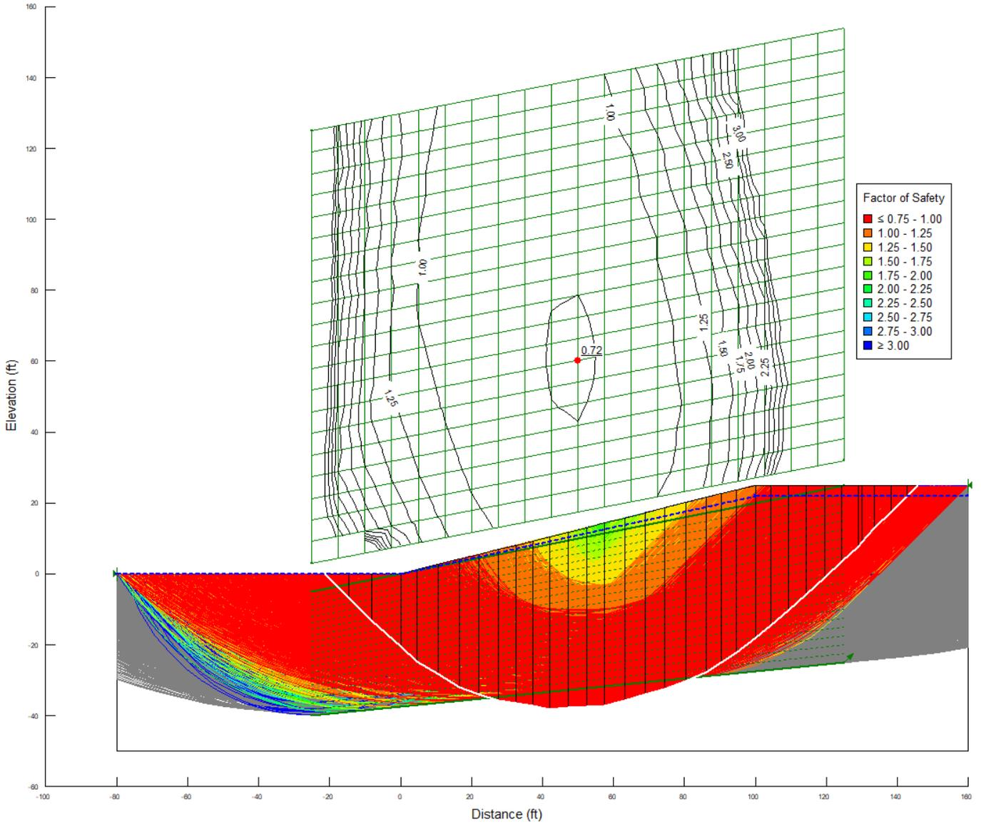
Figure A-5: SLOPE/W-Calculated Factor of Safety Results – Loose Sand (G1) on 3:1 Slope
