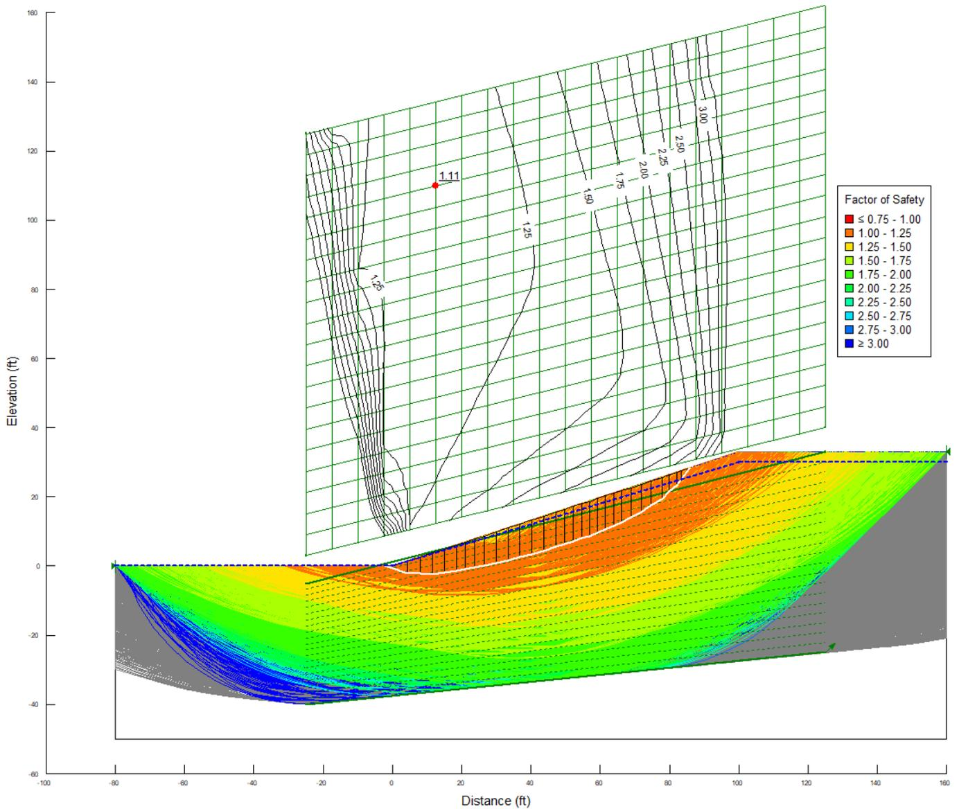
**Figure A-7: SLOPE/W-Calculated Factor of Safety Results – Dense Sand (G3) on 3:1 Slope**
