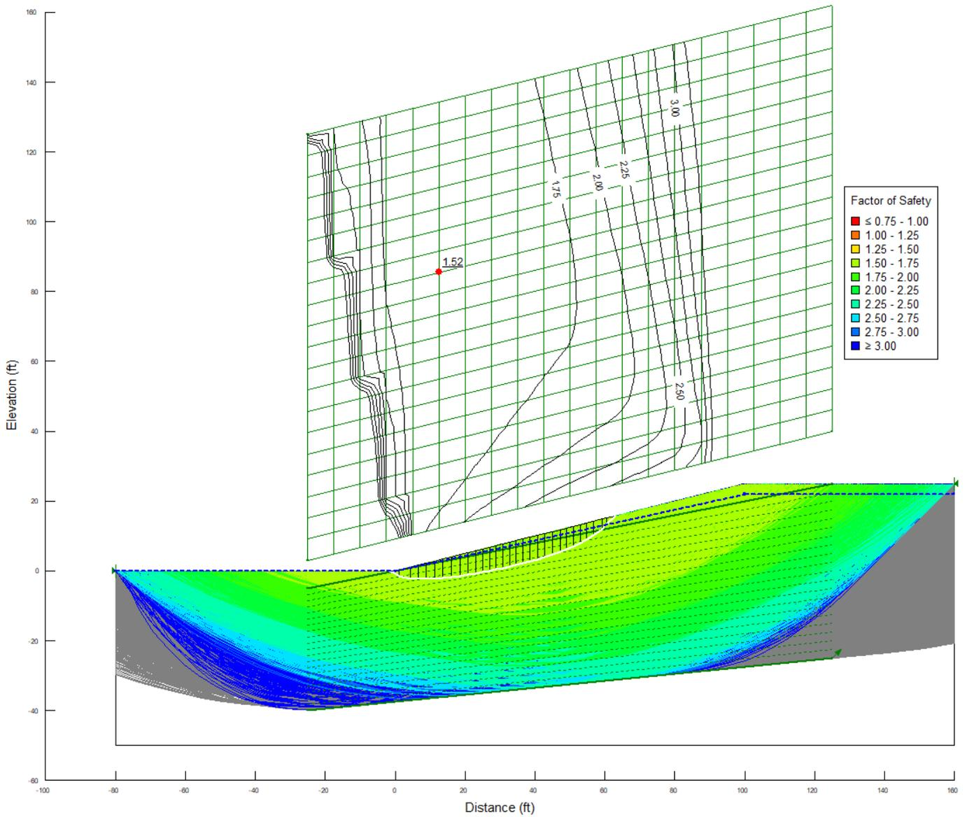
Figure A-4: SLOPE/W-Calculated Factor of Safety Results – Soft Clay (C1) on 4:1 Slope
