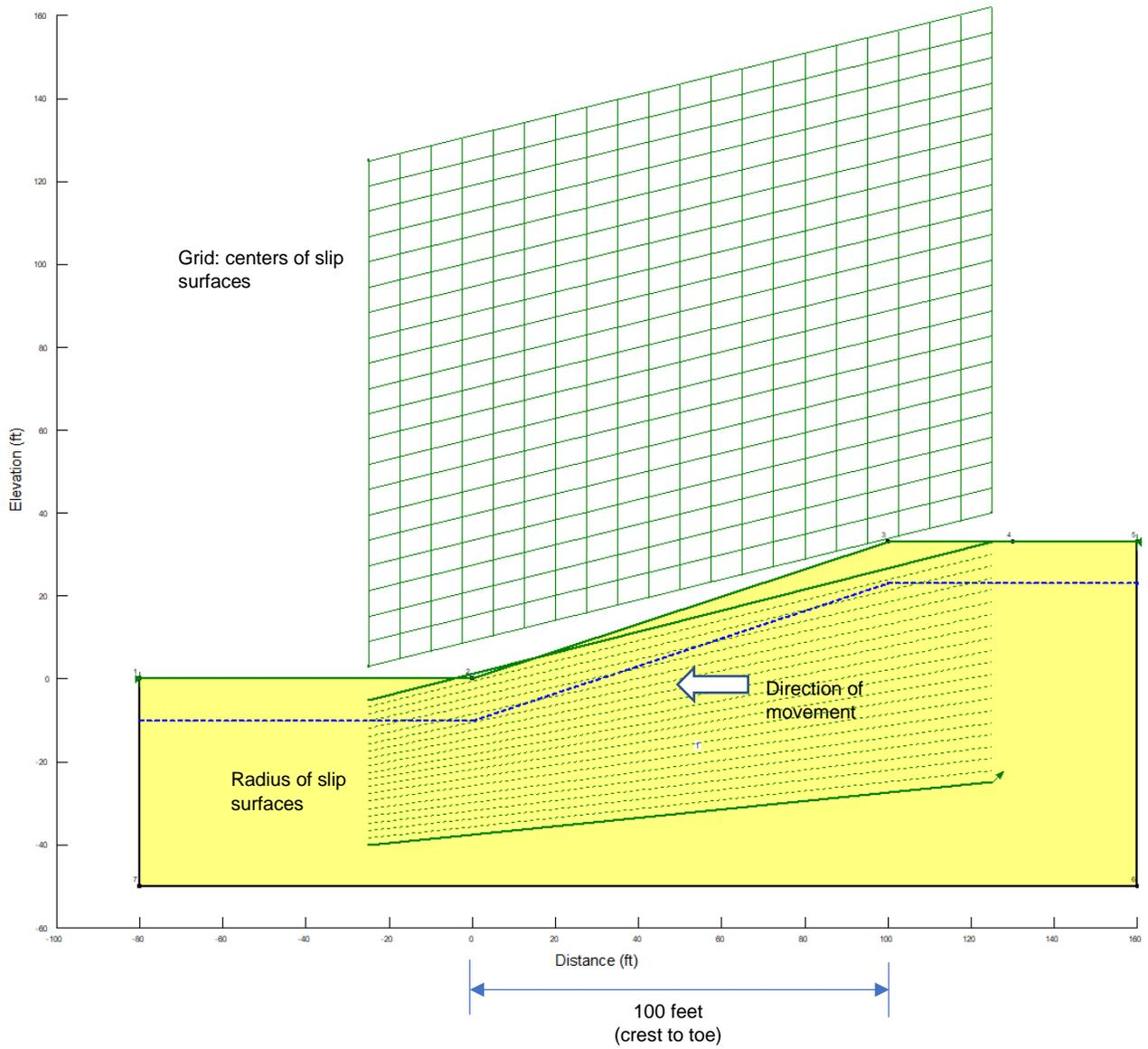
Note: Example shows a 3H:1V slope with one uniform material. Grid and radius method used for Grid and radius for circular slip surfaces.
