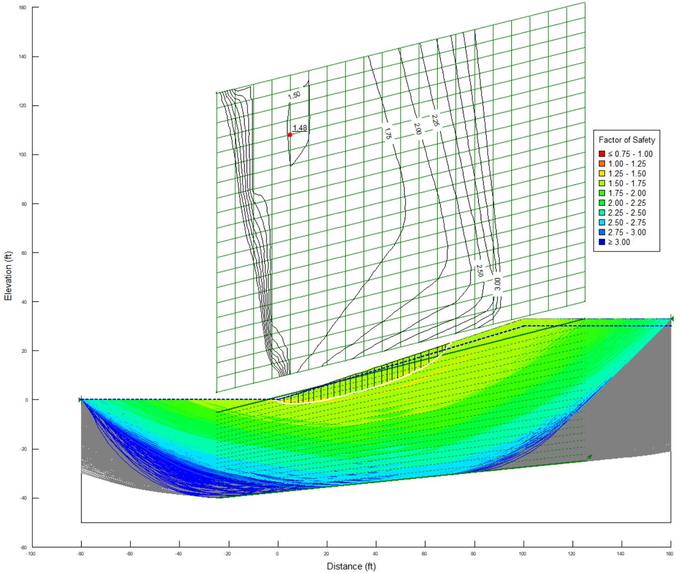
Figure A-8: SLOPE/W-Calculated Factor of Safety Results – Medium Stiff Clay (C2) on 3:1 Slope
