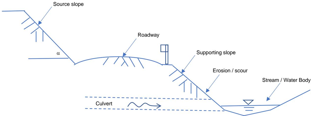
**Figure 2: Schematic of SLOPE/W Model**
