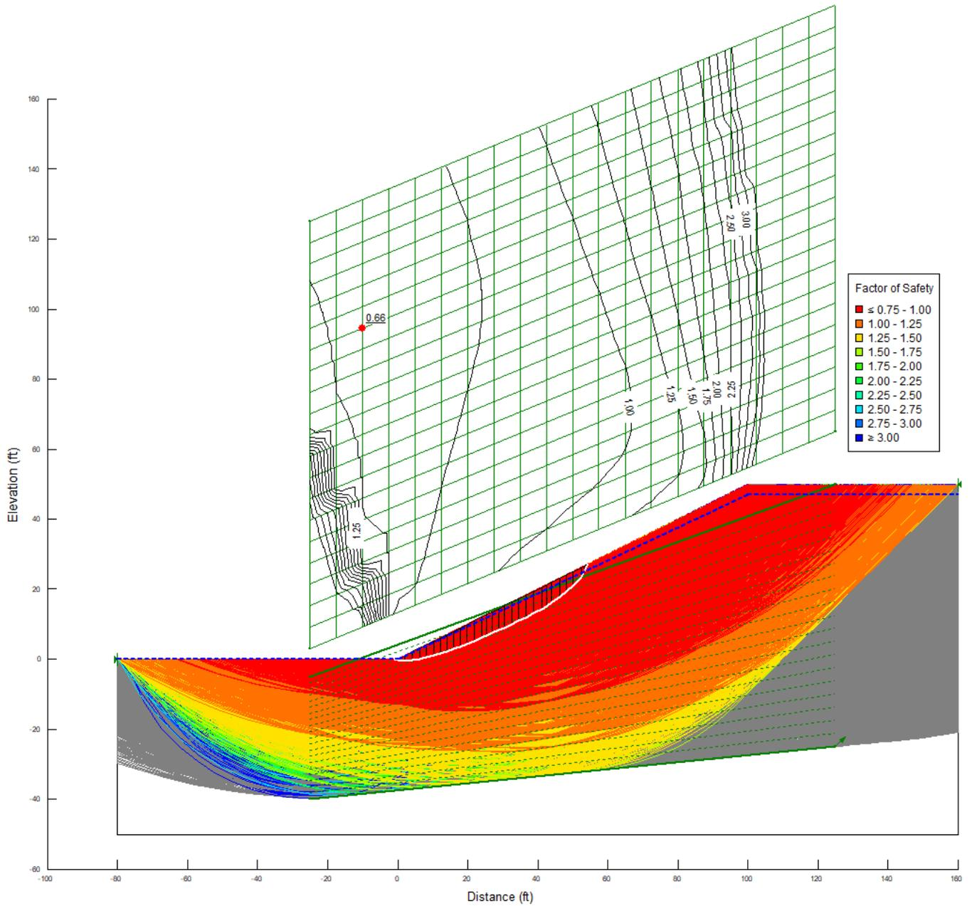
**Figure A-10: SLOPE/W-Calculated Factor of Safety Results – Dense Sand (G3) on 2:1 Slope**
