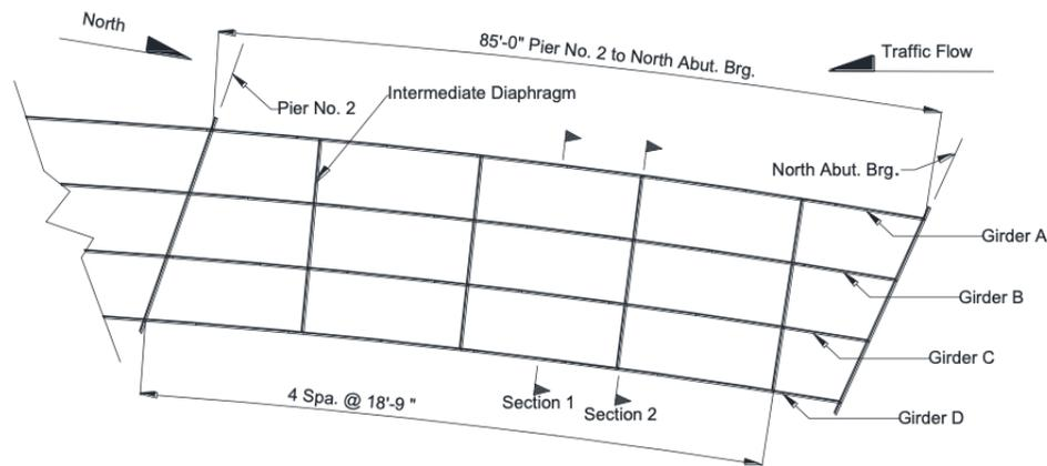
*Figure 1.5 - Plan View of Bridge 309 Instrumentation Sections [7]*
