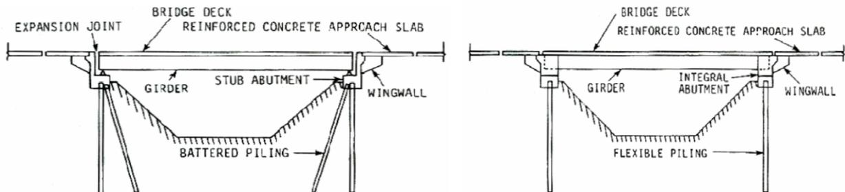
*Figure 1.1 - Schematic of a Jointed Bridge (Left) and an Integral Abutment Bridge (Right) [2]*
