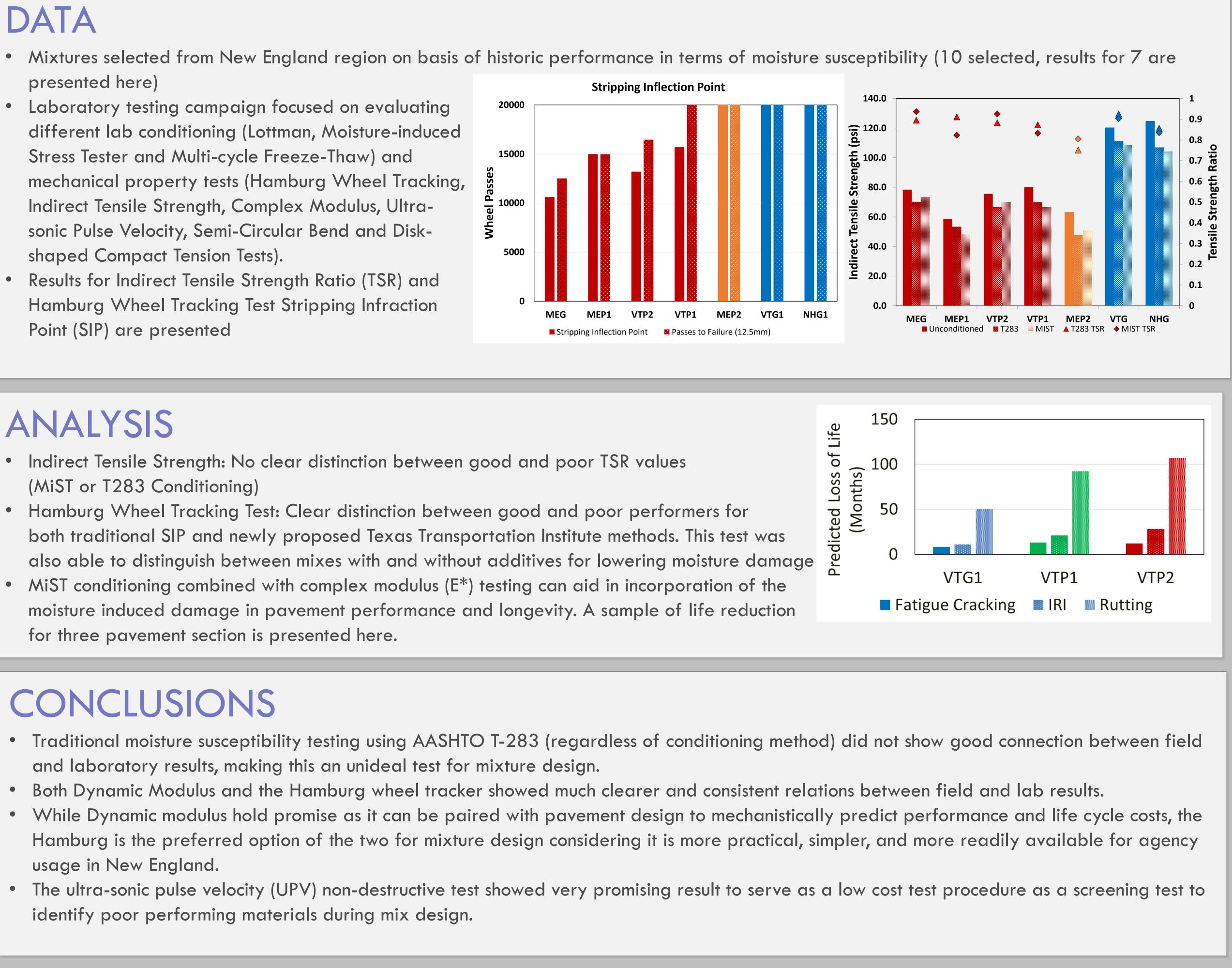
Results for Indirect Tensile Strength Ratio (TSR) and Hamburg Wheel Tracking Test Stripping Infraction Point (SIP) are presented
