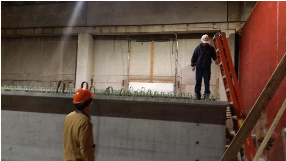
Figure 6 - Post-Pour Inspection; QA Inspector Observing QC Personnel Measure Camber after Destressing Bulb-Tee. (image taken at J.P. Carrara and Sons facility by researchers during site visit)
