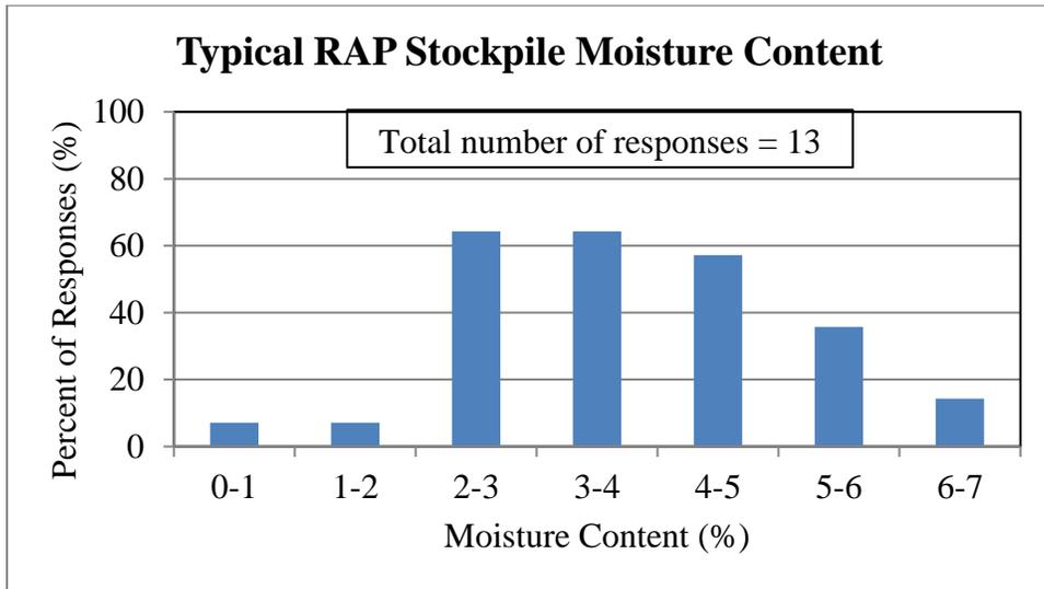
**FIGURE 2 Industry Survey Result - Typical RAP Stockpile Moisture Contents**
