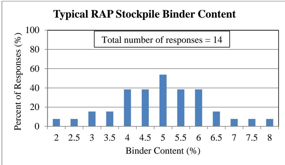
**FIGURE 1 Industry Survey Result - Typical RAP Stockpile Binder Content**
