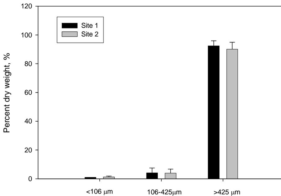
**Figure 3-3. Particle Size Distribution in the Sediments**
