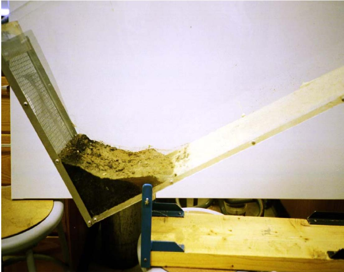
**Figure 6.1 Photo of 2-D Test Apparatus with Wood Waste Berm**
