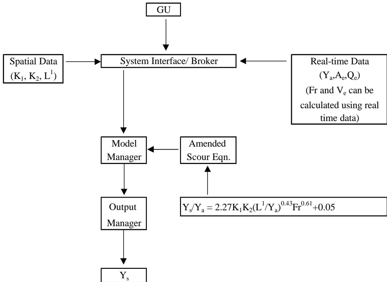
Figure 9: Flowchart of system architecture for engineering application
