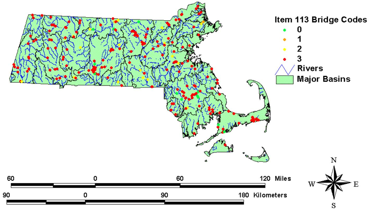
Figure 13. Multiple span, scour critical bridges in MA
