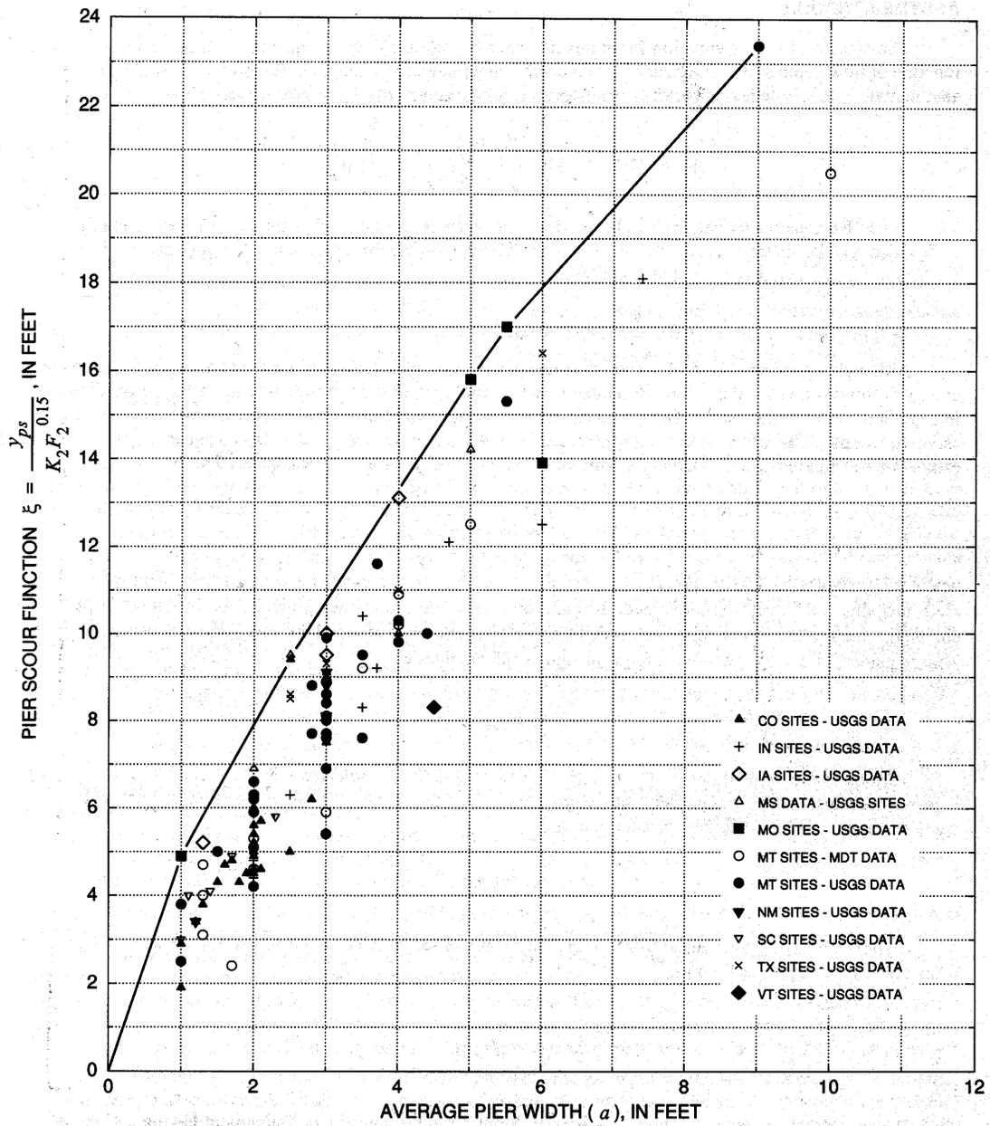
Figure 14. Envelope curve for estimation of pier scour (from Holnbeck and Parrett 1997)
